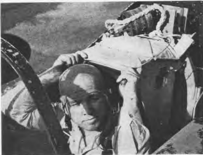
EJECTION SEAT FIRES WHEN FURTEK PULLS CURTAIN OVER FACE
