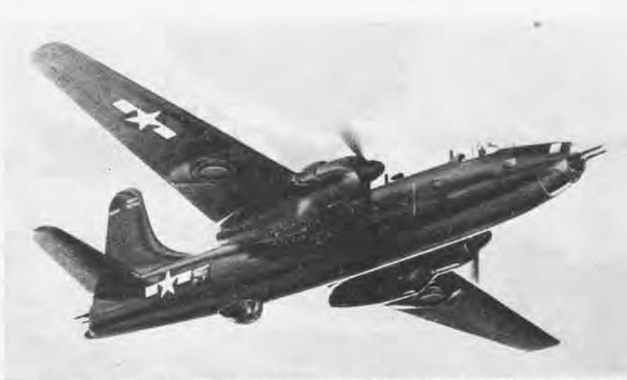
PHOTO OF MODEL XP4M SHOWS TANDEM MOUNTS OF BOTH RADIAL AND JET POWER PLANTS
