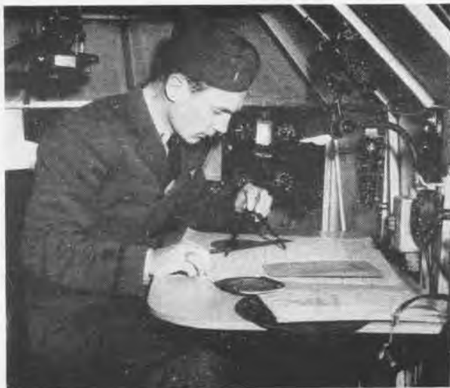
The celestial link trainer is fully equipped to simulate a night navigation flight, having even a shifting canopy of stars to watch
