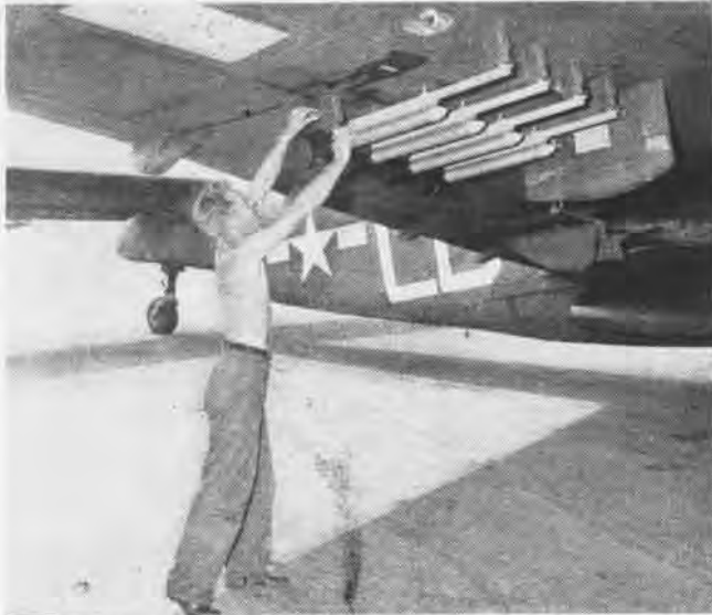
For safety the "pigtail" electrical firing circuit wire is plugged in at the end of runway just before take-off on rocket training flight
