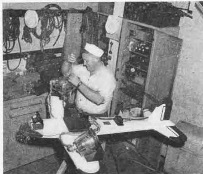
Long range oversea patrols are only as accurate as the aircraft's compasses. Here the transmitter of flux gate compass gets check
