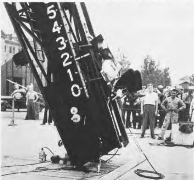
MAN PULLS CANVAS CURTAIN, FIRING SEAT'S POWDER CHARGE
