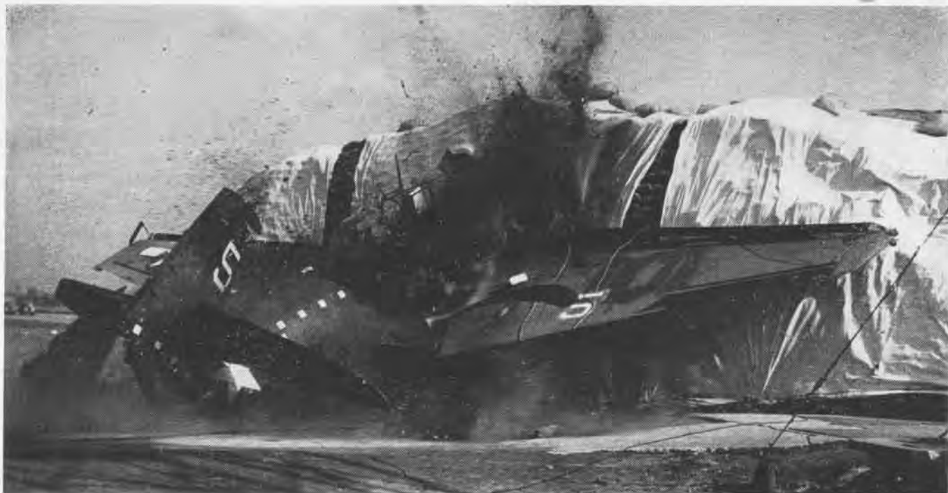
SURVEYED TBM RAMS SANDBAG BARRIER AT MUSTIN FIELD TO TEST NEW CRASH HARNESS; NOTE PROPELLER BLADE IN MIDAIR (CENTER)
