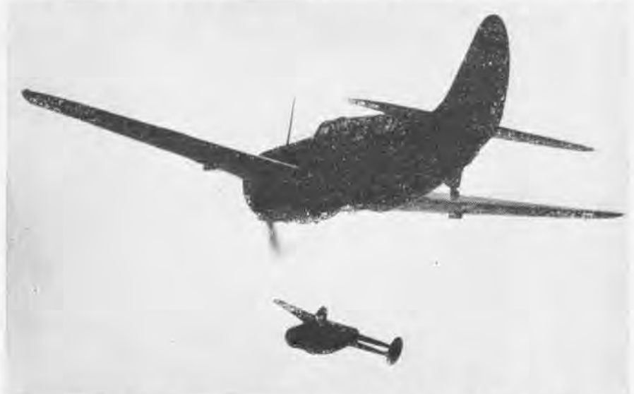
BAT BEING RELEASED BY HELLDIVER IS ON ITS OWN AFTER BEING SET UP BY OPERATOR
