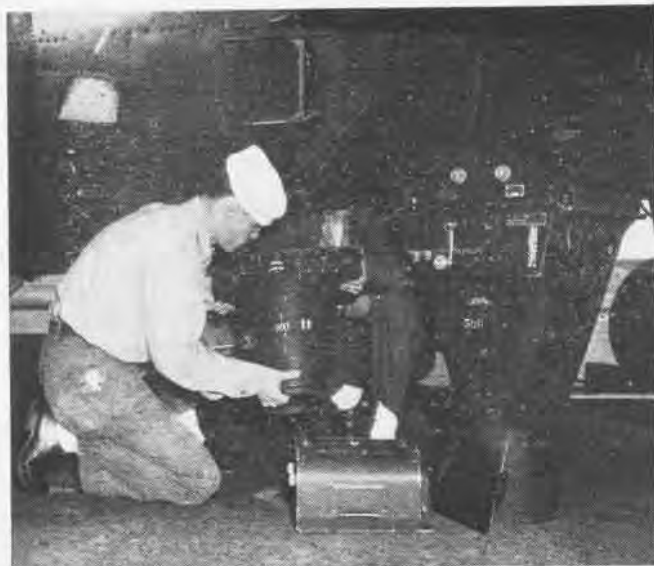
Fighter planes equipped for photographic recco training are used at Whiting. Here service crewmen put cameras in F6F-5P aircraft
