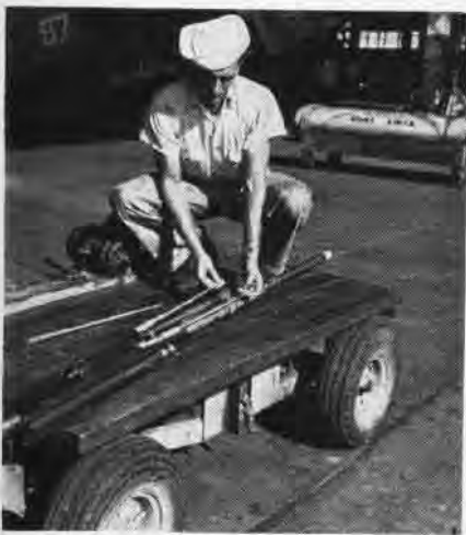
TIE RODS MODIFIED TO ALLOW ADJUSTING
