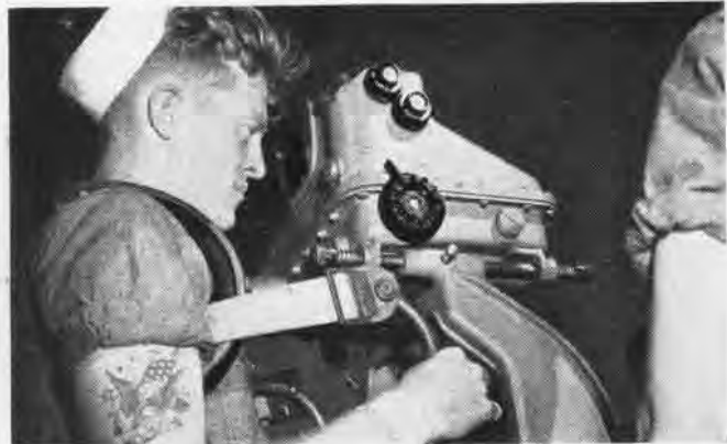
Midway's quadruplicate 40's are controlled by individual directors like this one. In this case it happens to be a Mk 51 director
