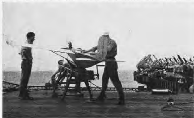
For antiaircraft gunnery, the Midway carried her own TDD unit, with crew and 15 drones. Drones were catapulted from the deck
