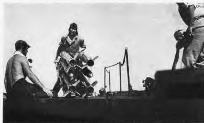
Red-capped V-3s bring ammunition from the magazine hatches to the planes. Here a load of rockets is rolled off an ammo elevator
