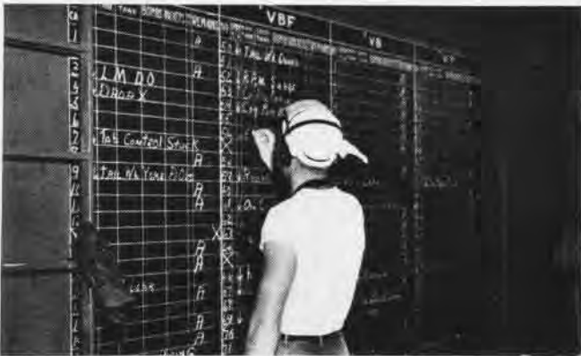
Status control board on the flight deck tabulates all troubles; information is relayed to Air Plot, Flight Deck Control, and V-2
