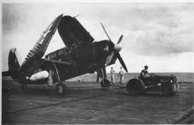
Re-spotting the Midway's vast flight deck is a complicated job for the plane handlers, and is accomplished largely with tractors
