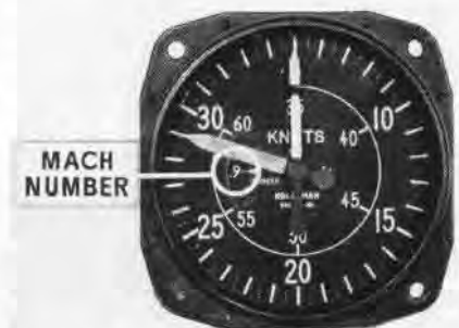
INDICATOR WARNS WHEN SPEED TOO HIGH
