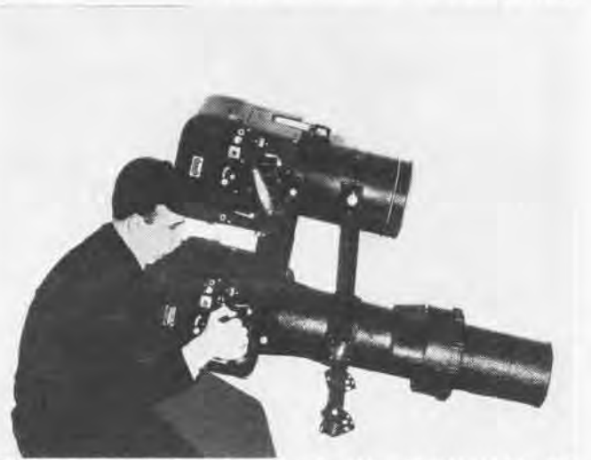
PICK-A-BACK F-56 CAMERAS WITH 20" AND 40" LENSES IN PBM
