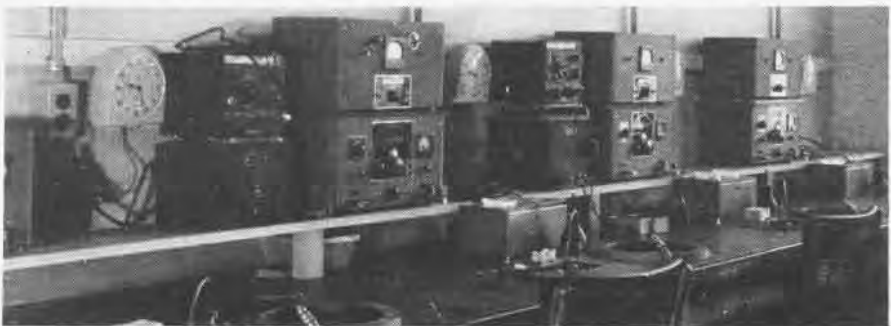
THESE HORIZONTAL LAPS GRIND CRYSTALS TO REQUIRED FREQUENCY IN FINAL PROCESS
