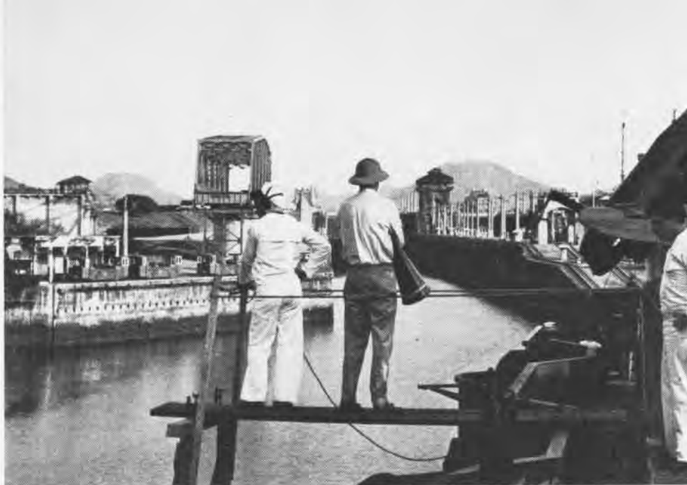
Saidor approaches a lock in the Panama Canal, with one of deck-corner pilots posted on a platform with megaphone and talker to advise skipper of wide-beam CVE on approach
