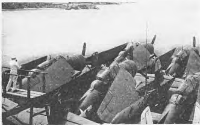
Aiming pole on bow and another on stern help chief pilot (left) line up Saidor to enter locks; ship has only five feet clearance
