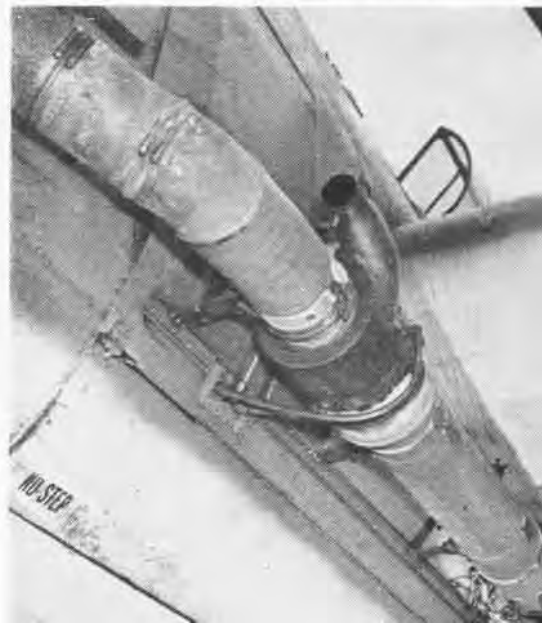
DDT tanks for F4U can be mounted in half hour. Adaptable to several Navy and Army planes, they can be jettisoned for combat
