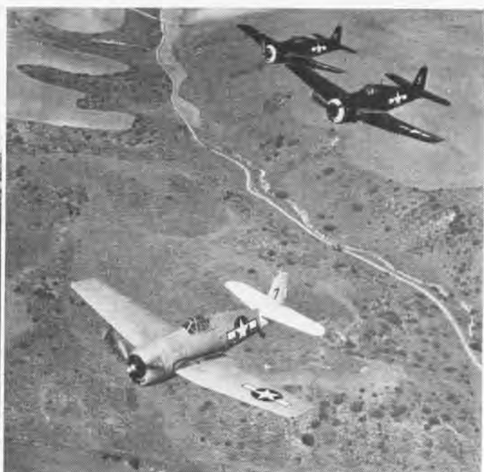
With its two mother F6F 's, a brightly-painted drone makes test flight; control planes will fly it into mushroom cloud of bomb
