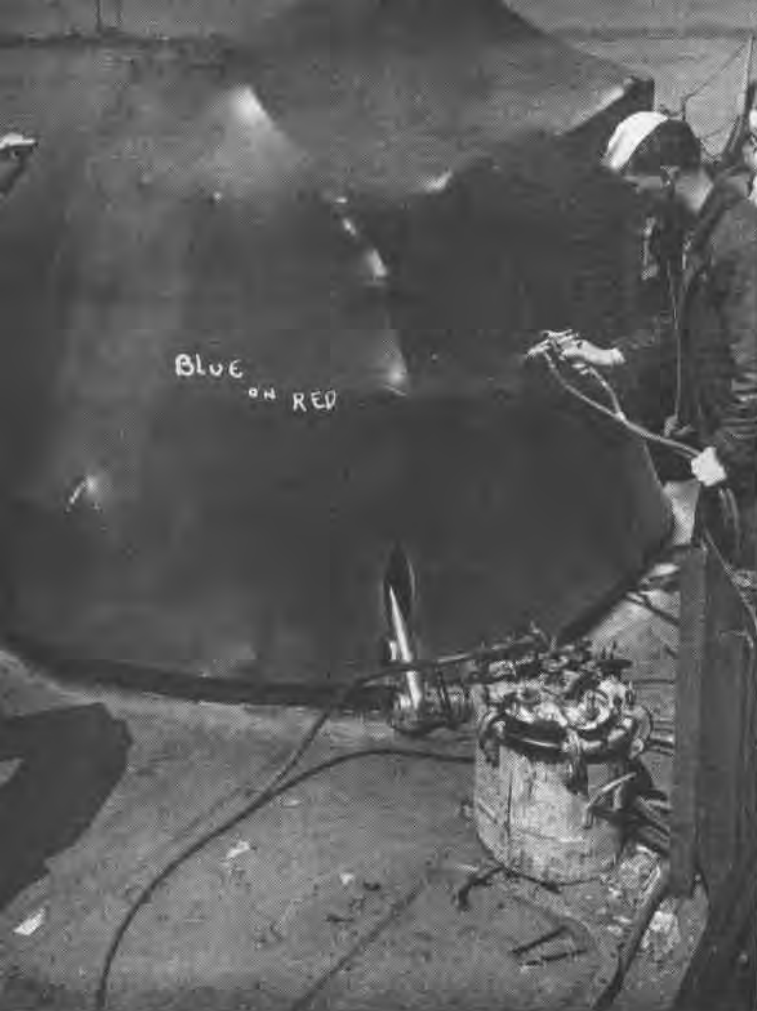
By using different colored plastic sprays, number of coats can be figured; here a blue coat covers red layer on 40 mm. twin mount Spray gun in hand, worker completes webbing on a 40 mm. twin mount; six different colored coats are applied to permit counting
