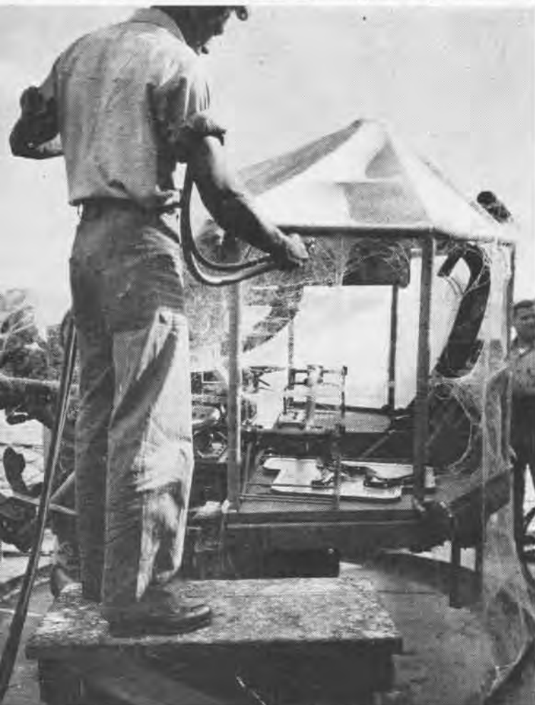
By using different colored plastic sprays, number of coats can be figured; here a blue coat covers red layer on 40 mm. twin mount Spray gun in hand, worker completes webbing on a 40 mm. twin mount; six different colored coats are applied to permit counting
