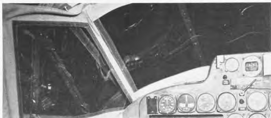
WITH IFIS-DEVELOPED BLUE-AMBER CURTAIN, INSTRUCTOR CAN SEE OUT, NOT STUDENT
