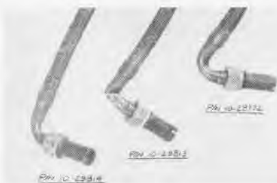
OVER-TIGHT NUTS CAUSE ELBOW BENDING
