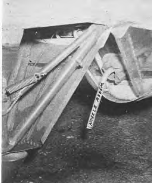
Lethal nozzle replacing tunnel gun in TBM leaves 300 foot swath. Avenger covers 550 acres in one hop at 165 mph ground speed
