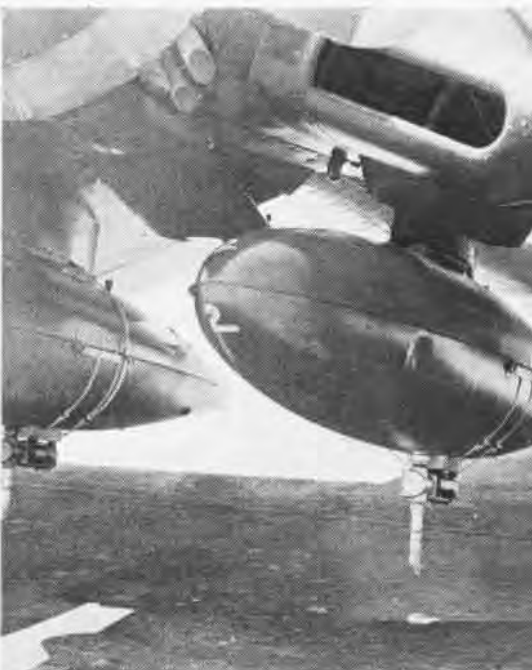
DDT tanks for F4U can be mounted in half hour. Adaptable to several Navy and Army planes, they can be jettisoned for combat
