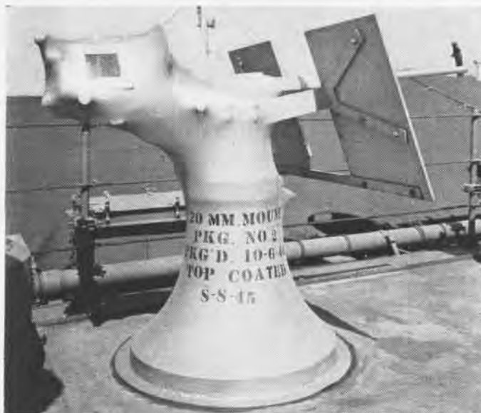
Tight plastic film covers a 20 mm. mount and barrel; window at breach enables a worker to see amount of humidity on the inside
