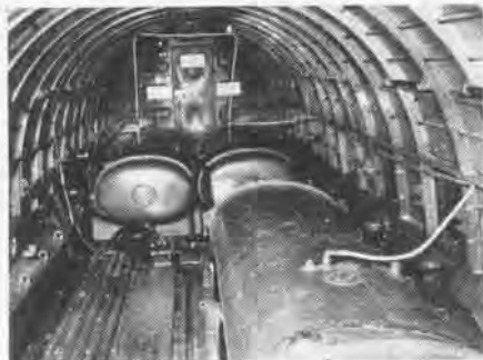
TANKS HOLD 510 GALLONS OF BUG SPRAY
