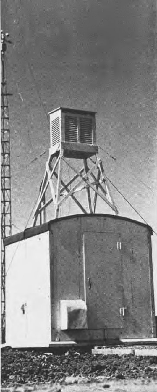
Land type automatic weather station used in Newfoundland, Hawaii, the Aleutian area. Meteorological equipment is housed in the superstructure. Lower shelter holds power plant, transmitter, and control apparatus.
