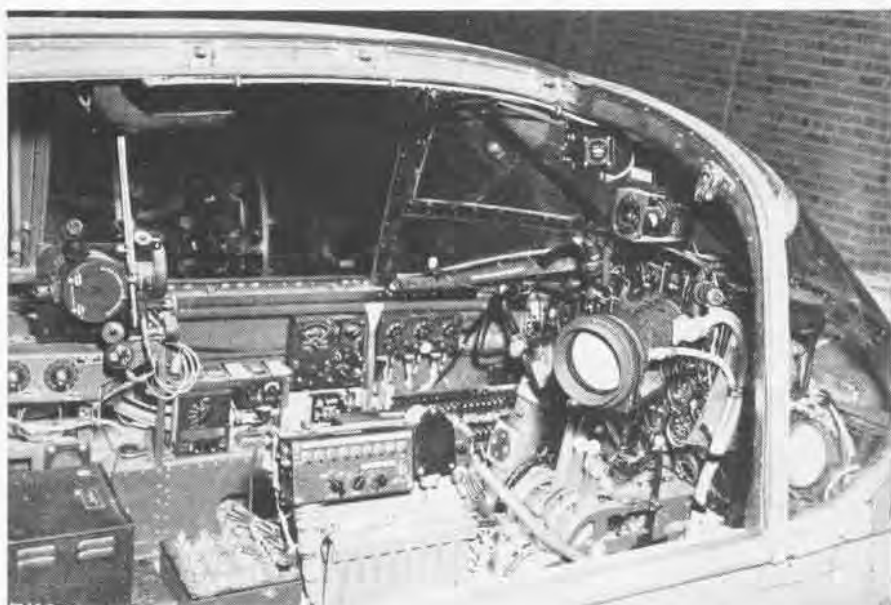
JD-1 cockpit is cramped to give pilot radar scopes and to allow navigator's gear to be placed in forward compartments of the multi-purpose high-speed aircraft
