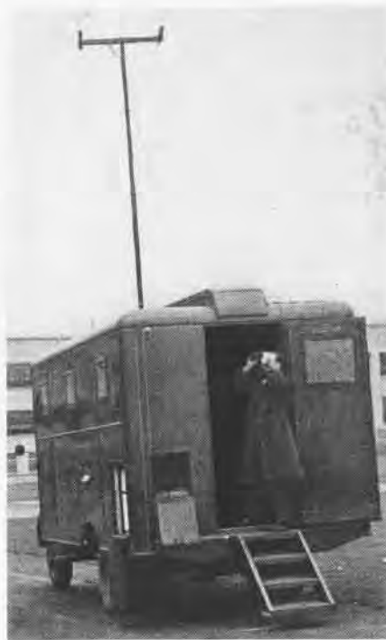
This mobile receiving unit houses radio, television devices to record flight test data of planes at ranges up to 25 miles
