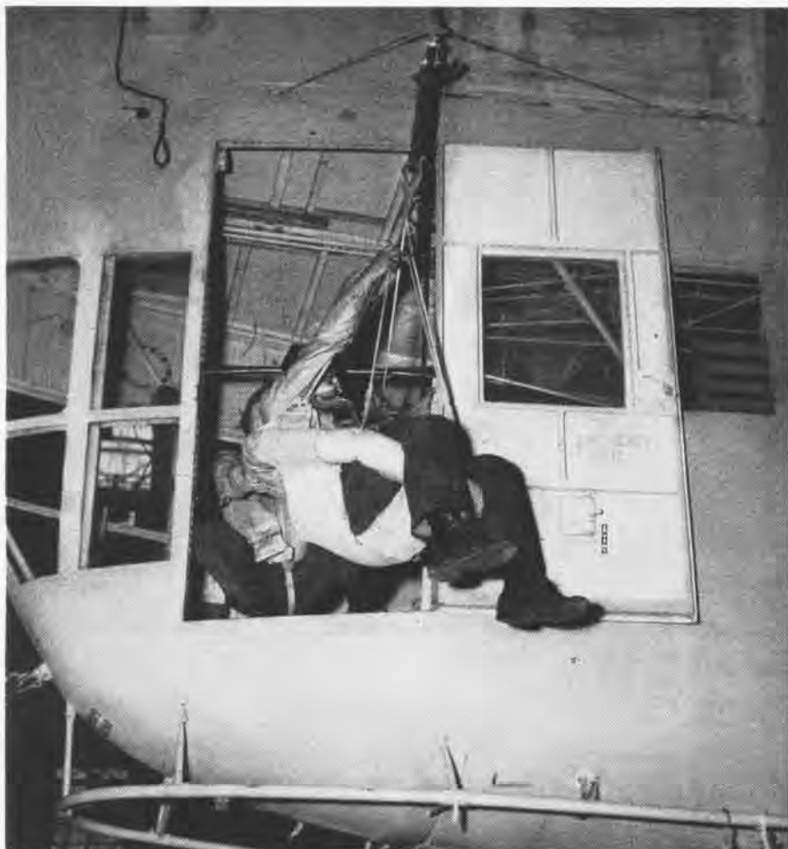
AFT DOOR OF THE K-65 SHOWS RIGGING OF LIFE RING USED IN RAISING AND LOWERING
