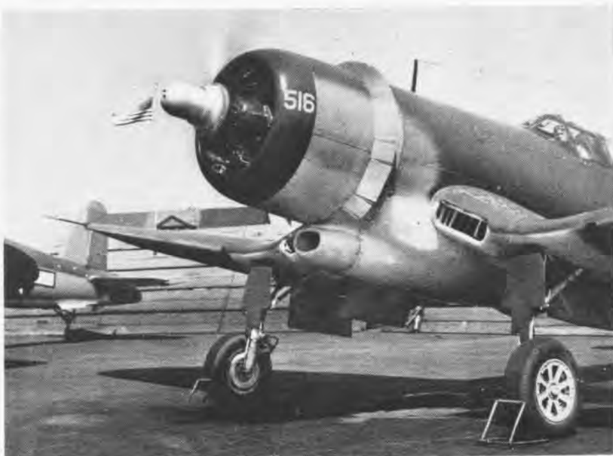
NEW TURBO-SUPERCHARGER IS INSTALLED WITHIN COWLING BUT REMAINS AIR COOLED
