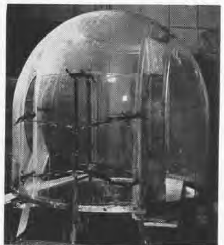
RIGID CLAMPS HELP IN PATCHING PLEXIGLAS
