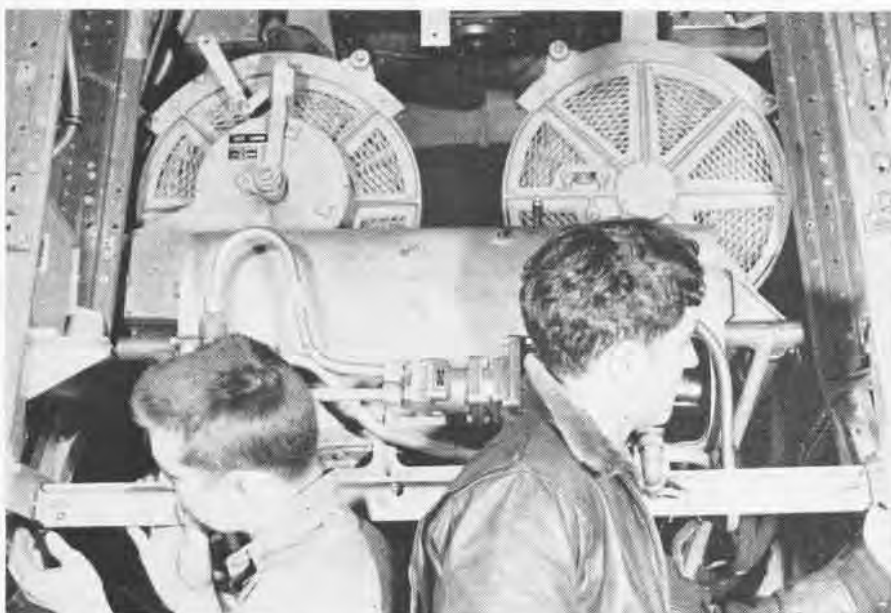
Mar 1k Mod 0 power system (hydraulic) is used to supply energy for this Mk 8 Mod 0 tow-target reel. Men above are applying easy method of removing the power unit
