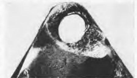
BACKFIRE DOOR BOLTHOLE AFTER 25 HRS.
