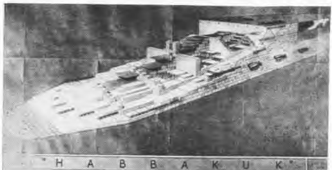
Europe. The proposed unsinkable carrier was to be constructed of reinforced ice blocks, having a length of 2000 feet, a width of 300 feet and a depth of 200 feet. After considerable research a 1000-ton
