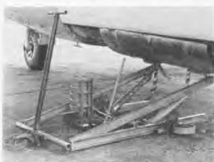
HOIST SPEEDS BAY TANK INSTALLATIONS
