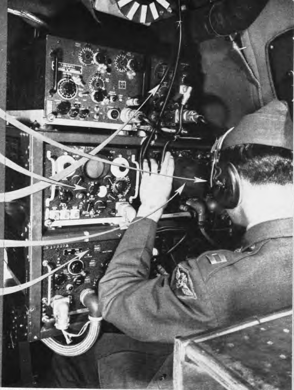
RCM INSTALLATION ON PV PUTS ALL INSTRUMENTS WITHIN REACH OF OPERATOR, WHO RECEIVES, ANALYZES AND JAMS ENEMY RADAR
