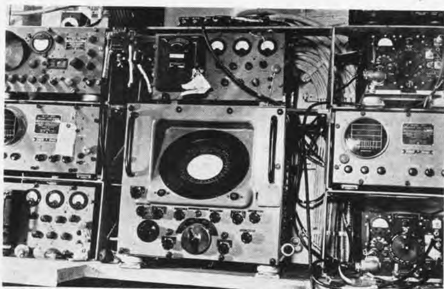
SHIPBOARD RCM INSTALLATION WITH DIRECTIONAL SCOPE IN CENTER, RECEIVER ABOVE
