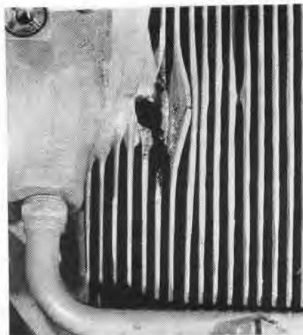
WANDERING VALVE STEM CUTS CYLINDER
