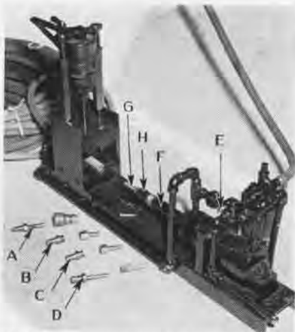
ADAPTERS ACCOMMODATE VARIOUS SIZES
