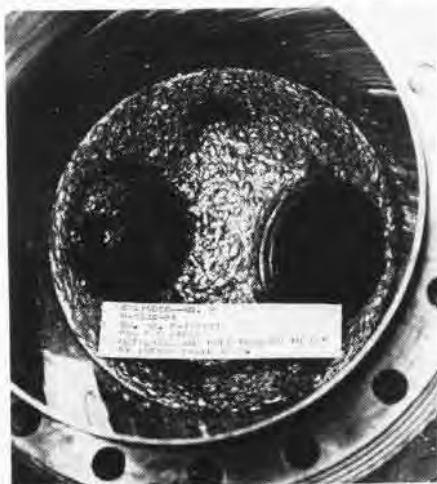
DAMAGE STARTED FROM A LOOSE LOCK NUT
