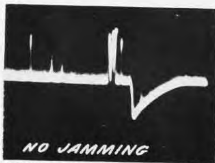
JAMMING MAKES CLEAR SIGNAL ON SCOPE (LEFT) UNREADABLE WITH 'GRASS' (RIGHT)
