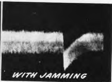
JAMMING MAKES CLEAR SIGNAL ON SCOPE (LEFT) UNREADABLE WITH 'GRASS' (RIGHT)
