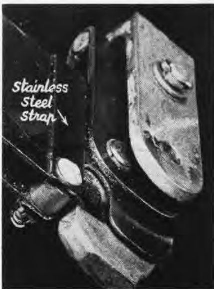
NEW STRAP ON SPACER PREVENTS FAILURE
