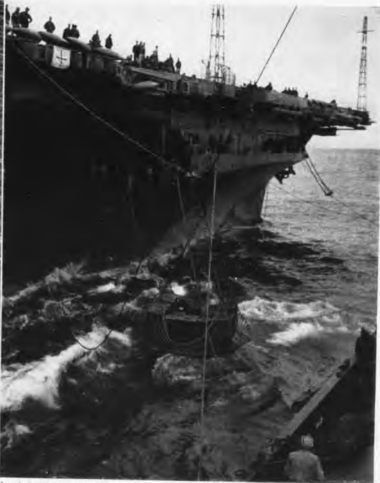
Loaded cargo nets are passed from supply ship to the carrier by means of "burtoning" method. Personnel move from ship to ship on the trolley rig
