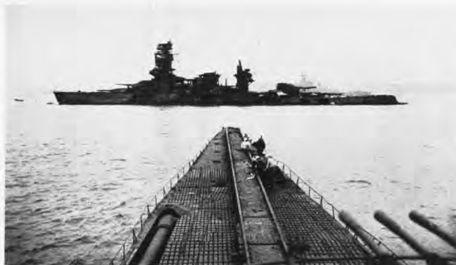
CATAPULT RUNWAY EXTENDS FROM 'TUBE' HANGAR TO BOW; BB NAGATO IN BACKGROUND
