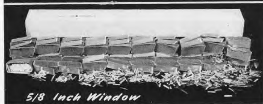
American aircraft tossed out window of various lengths according to wave length of enemy radar or utilized the 400-foot streamers of 'rope' which proved effective radar jammers
