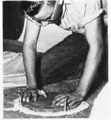
insures even bearing. Three sizes of plates are used for each test section
