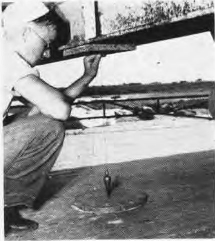
Centering plate for load. Areas showing surface cracks make good spots for tests
