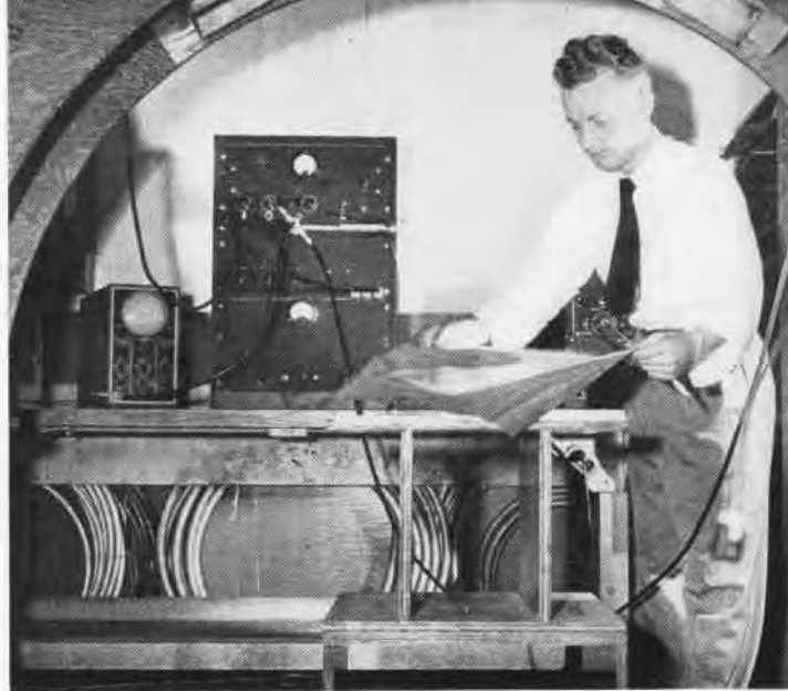
Reflection measurements of 'harp' indicate reflection coefficients at micro wave frequencies. This is radar 'window' test
