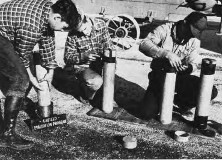
Undisturbed soil samples taken from site of plate loading tests are capped, taped, and paraffin sealed for accurate lab analysis
