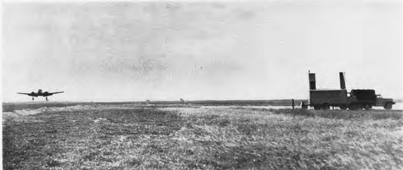
SNB LANDS AT BANANA RIVER, HAVING BROKEN THROUGH A 150-FOOT OVERCAST AT THE COMPLETION OF GCA CONTROLLED APPROACH
