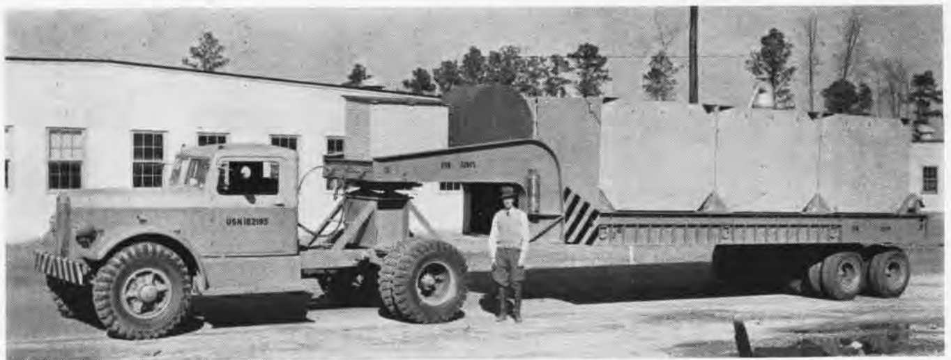
TANKS OF WATER ARE CONVENIENT METHOD FOR PROVIDING 75,000 POUND LOAD ON TRAILER USED FOR PLATE LOADING TESTS
