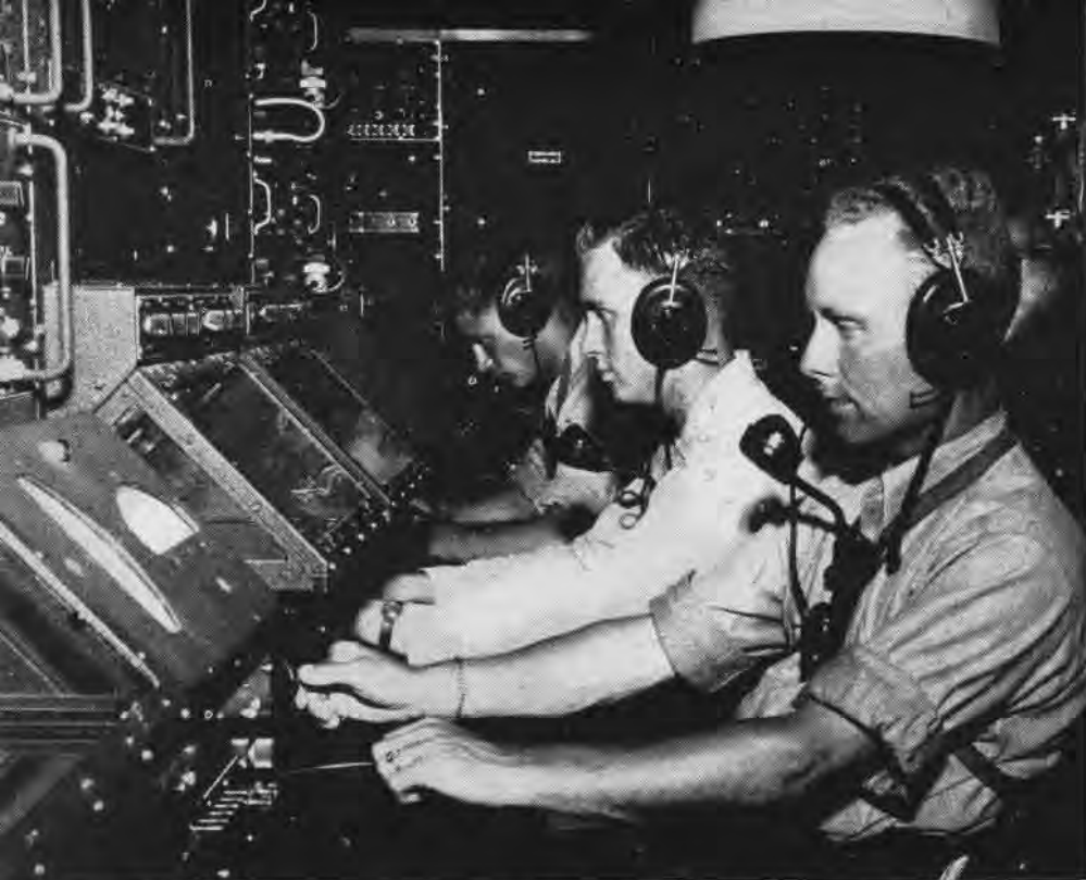
Three crewmen concentrate on the landing of a fogbound plane. In the foreground may be seen the scale with built-in miniature plane which interprets variations
