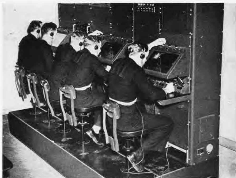
Five man crew functions as one mind in lowering aircraft through fog and stratus to the deck. In order to communicate with each other, panels are placed together
