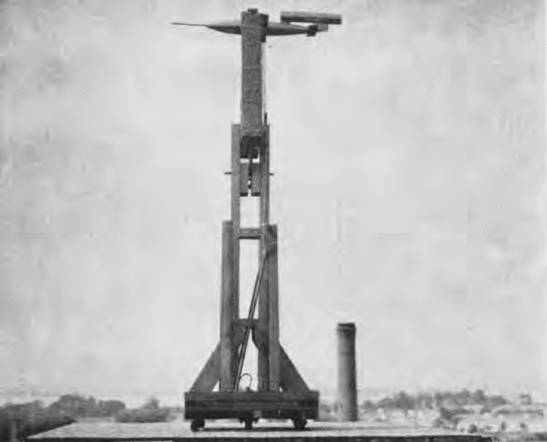
Among the most recent projects undertaken by NRL is developing of jet and pilotless missiles. This is the JB-2 ready to launch
