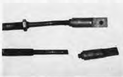
BENT AND BROKEN ARENS ACTUATING RODS
