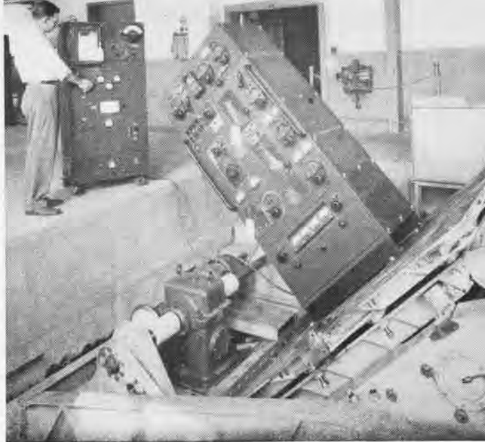
Testing devices simulate realism. This table tests equipment under roll of ship, motor vibration, concussion hammer 'explosion'
