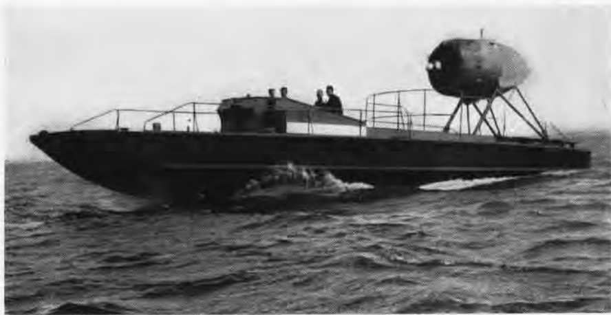
46' REMOTELY-CONTROLLED TARGET BOAT PERMITS UNRESTRICTED ATTACK TECHNIQUES
