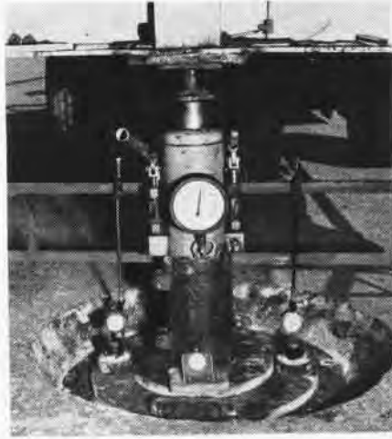
Loading test being made on subgrade soil; dial gauges measure amount of settlement
