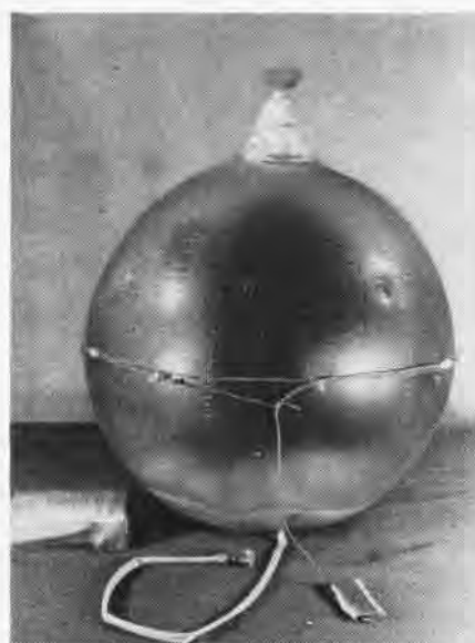
INFLATED STILL READY TO PRODUCE WATER
