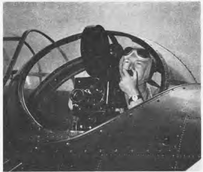
Extremely good still and motion pictures were taken from modified turrets of Saidor's Avengers ; special crutch held F-56 20" camera
