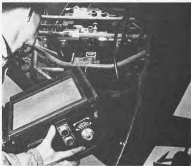
Technician loads magazine of K-17 vertical camera; Hellicat mount also holds two oblique cameras for shooting out of fuselage ports
