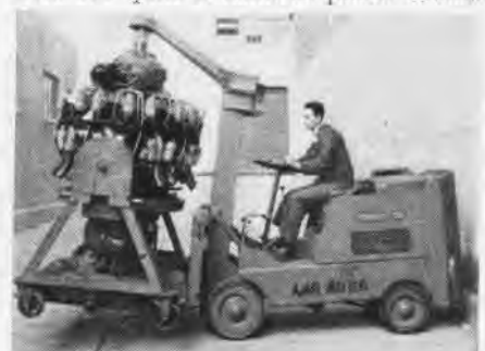
STACKER CARRIES ENGINES WITH STANDS
