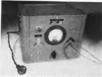
HYGROMETER POWER AND INDICATOR UNIT
