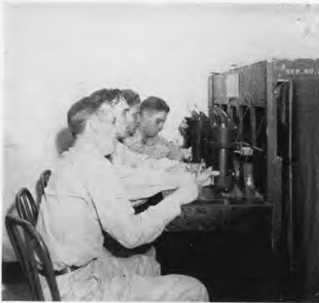
Smile of nearest student indicates a Jap in the sights. Idea of device is to mark when aircraft at end of tunnel is in range
