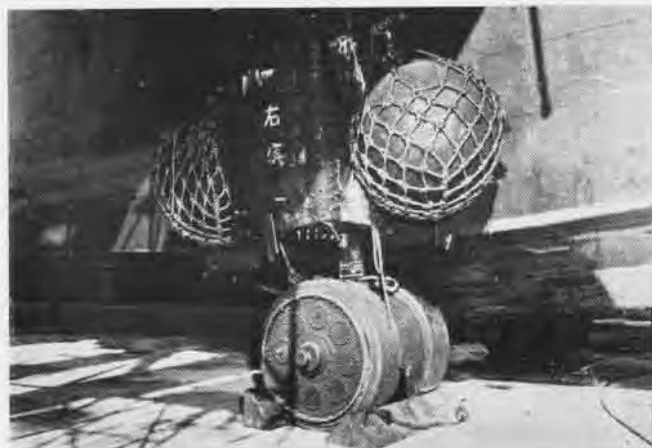
ODD JAP BEACHING GEAR WITH FLOAT BALLS HAD TO BE FIXED
