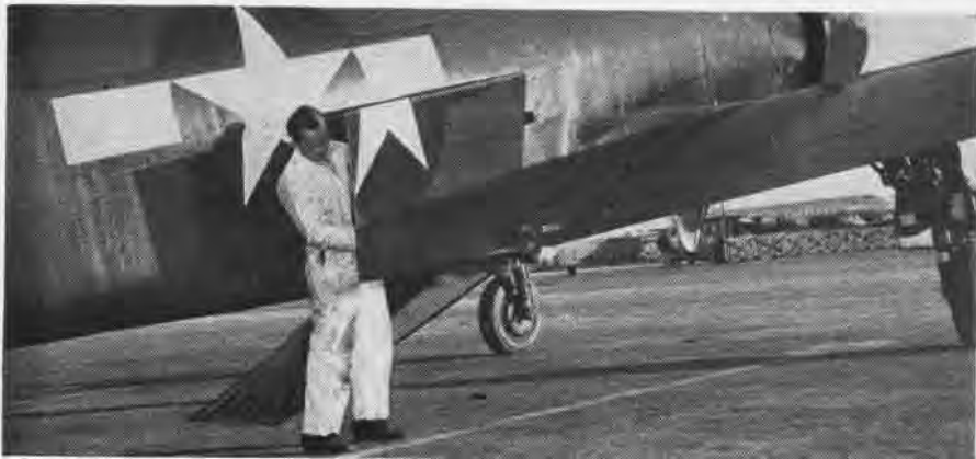
THREE FUSELAGE FLAPS REPLACE OLD BANANA-PEEL TYPE TRIED ON EARLIER BTD PLANE
