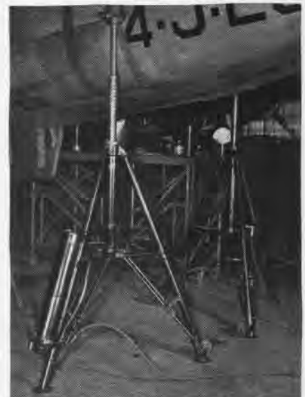
TWIN MODEL JACKS AID IN LIFTING PLANE
