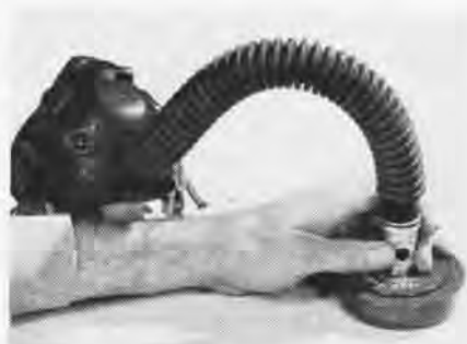
HOSE OF MASK PLUGS IN THE CONNECTOR
