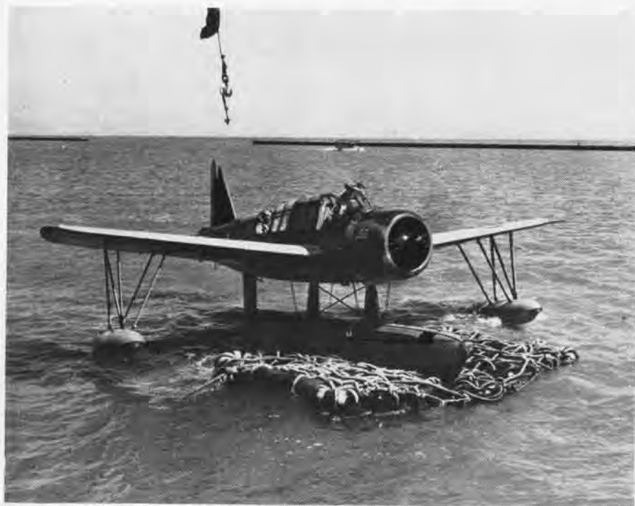
USE OF OLD TIRES FOR BEACHING SEAPLANES SAVES SQUADRON TIME AND MANPOWER
