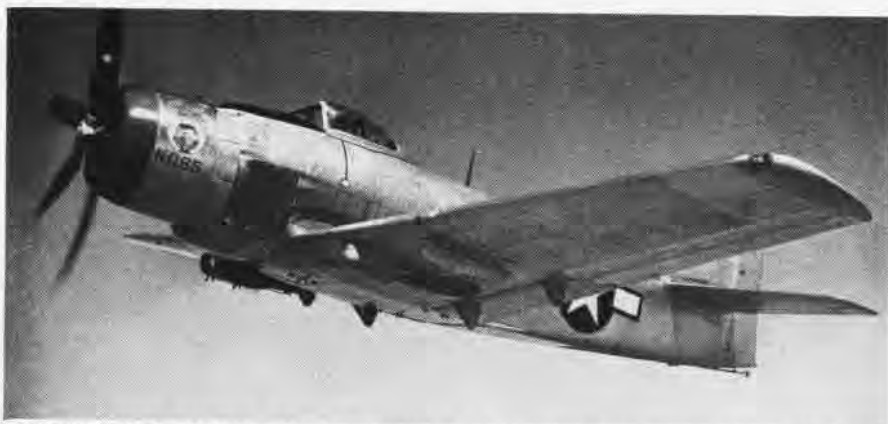
NEW SKYRAIDER CARRIES BOMBS, TORPEDOES EXTERNALLY TO BOOST GET-AWAY SPEED
