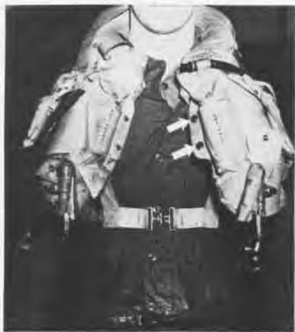
FASTENERS FAIL TO HOLD ON VEST LOBES
