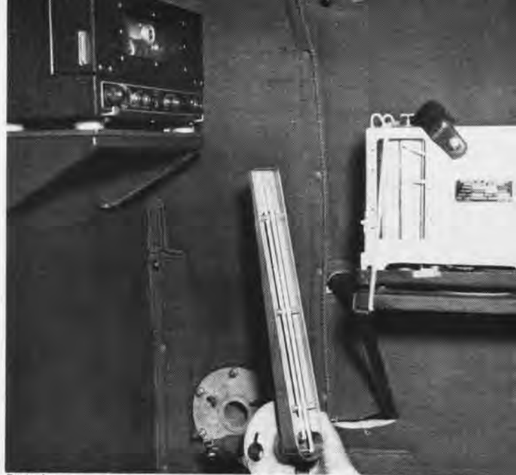
Part of meteorological equipment on Navy hurricane patrol plane shows from left to right: wire recorder, psychrometer, barograph
