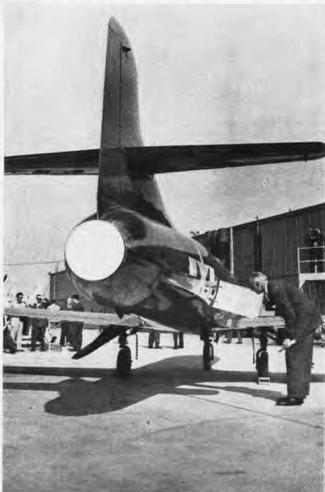
CIGAR-SHAPED FUSELAGE, HIGH RUDDER FEATURE 'SKYSTREAK'
