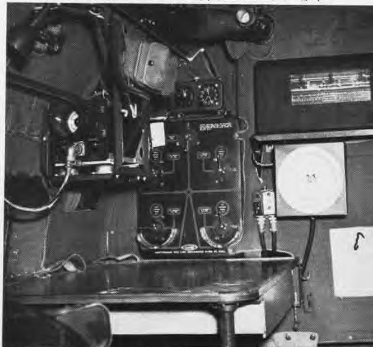
Within close reach of aerologist's table are the radio altimeter, pressure altimeter, 24-hr. clock, aneroid barometer and aerograph
