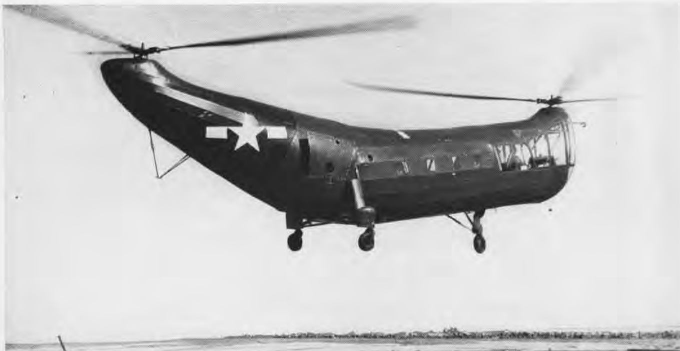
PIASECKI HELICOPTER, PIONEERED BY NAVY, IS FIRST TANDEM MODEL TO FLY; CAN LIFT 10 PERSONS, INCLUDING CREWMEN
