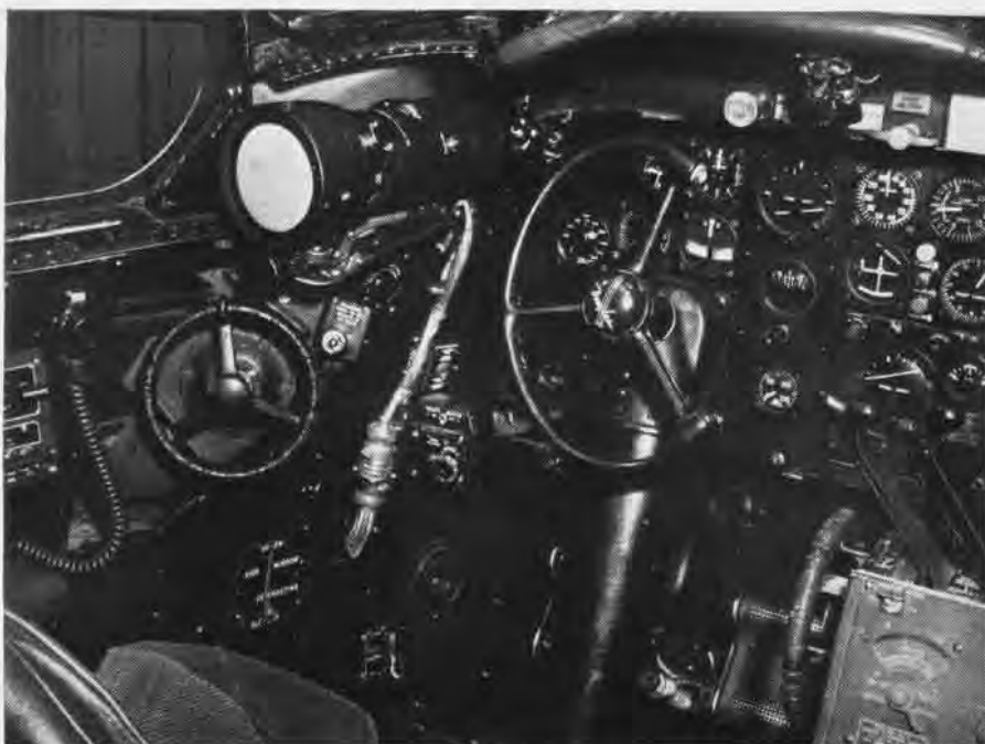
AIRLINER PILOT CAN KEEP ONE EYE ON SCOPE; PPI LOCATED ON CO-PILOT'S SIDE TOO
