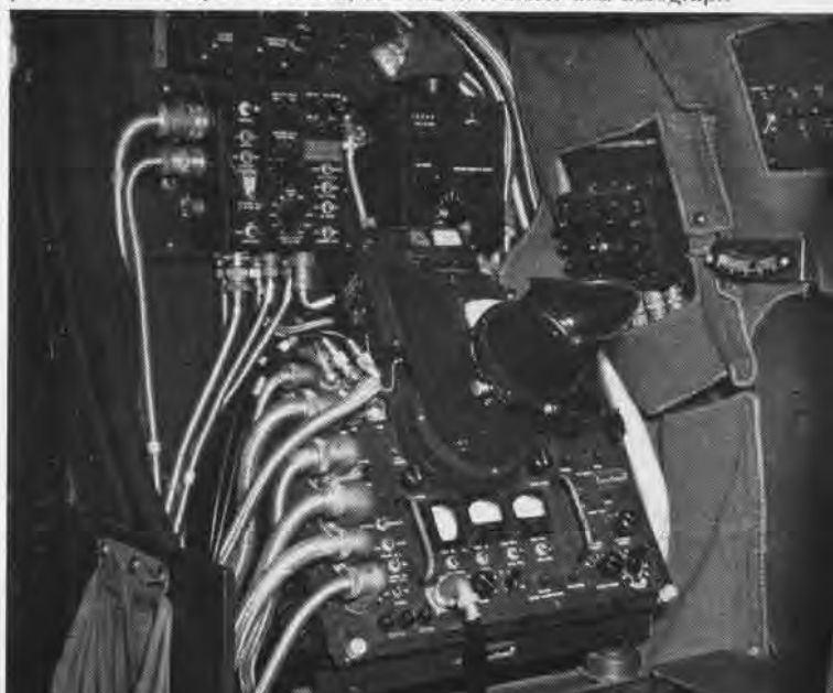
Within close reach of aerologist's table are the radio altimeter, pressure altimeter, 24-hr. clock, aneroid barometer and aerograph
