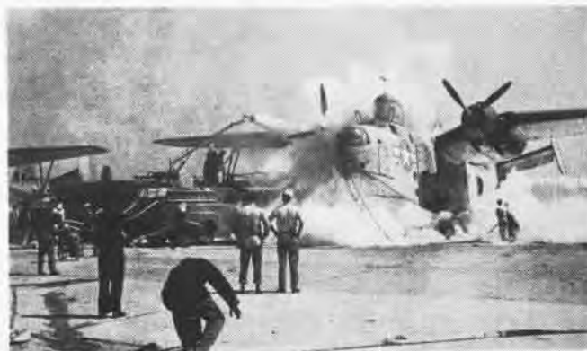
Mariner engine fire is extinguished by FFN-5 truck (front) squirting fog and foam and FFN-4 covering engine with CO 2
