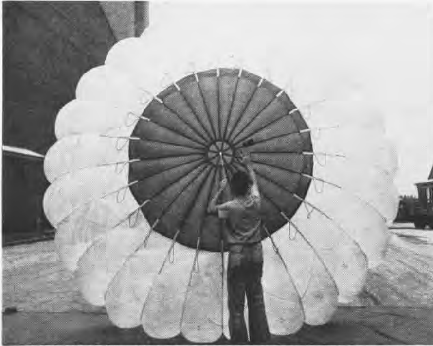
COLORED SECTION FORMS A CAP WHICH RAISES ON ELASTIC CORDS WHEN CHUTE FIRST OPENS
