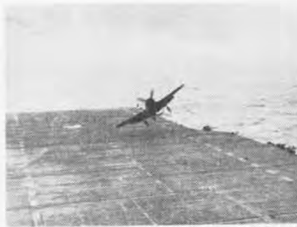
2 Bearcat's airspeed is too slow and plane abruptly stalls out to right
