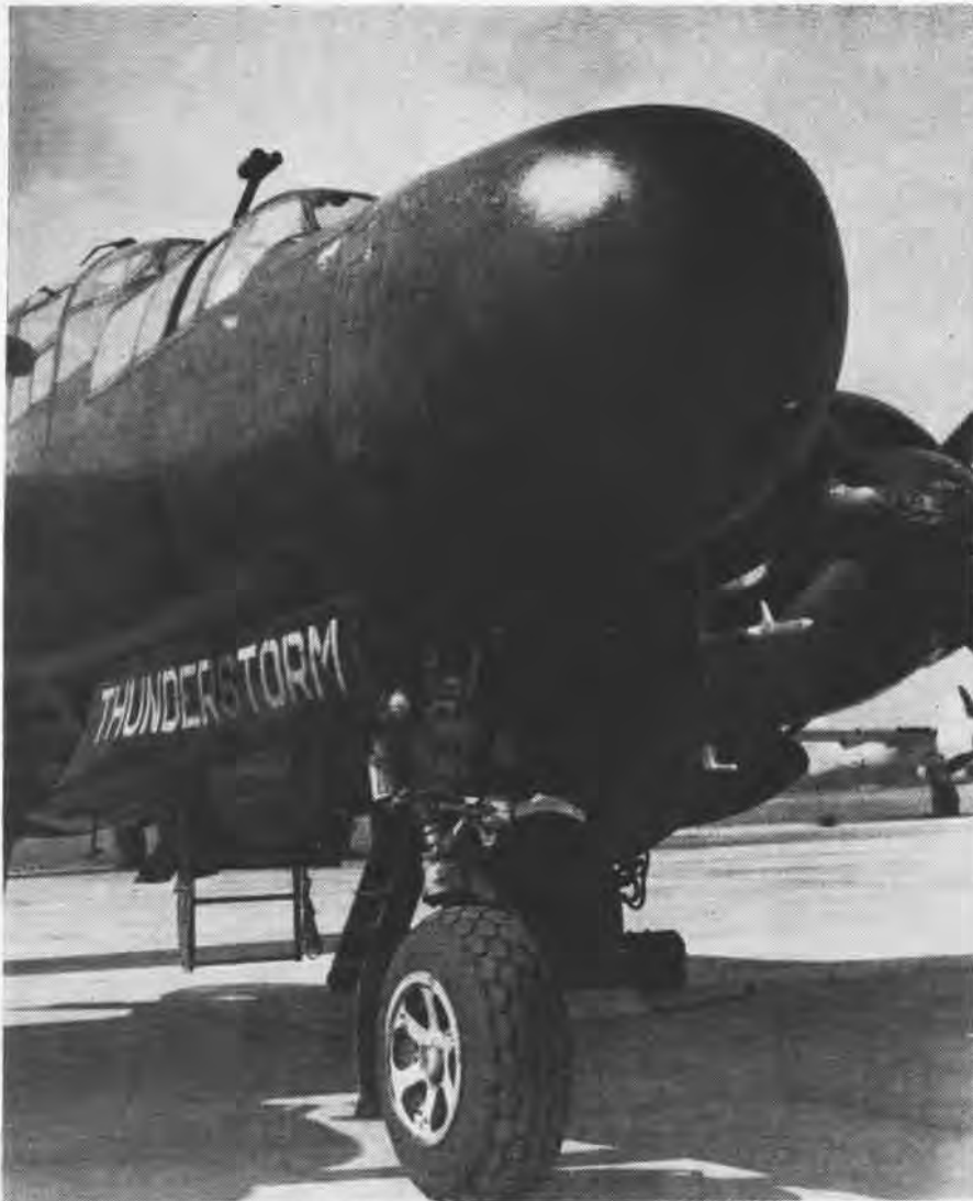
BLACK WIDOW HAS SPECIAL PITOT FOR AIRSPEED RECORDER AND A TEMPERATURE GAUGE ON TOP
