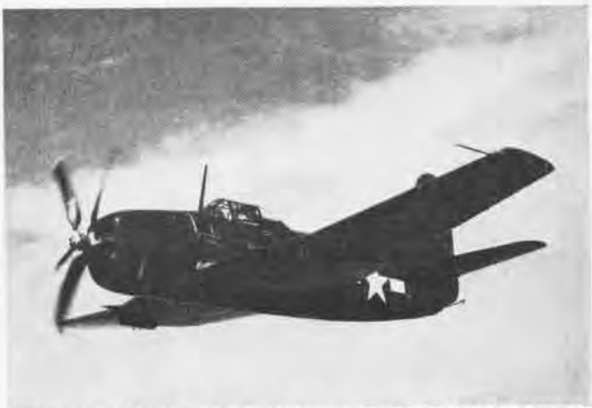
XBTC-2 WITH COUNTER-ROTATING PROP WAS ATTACK PLANE ANCESTOR
