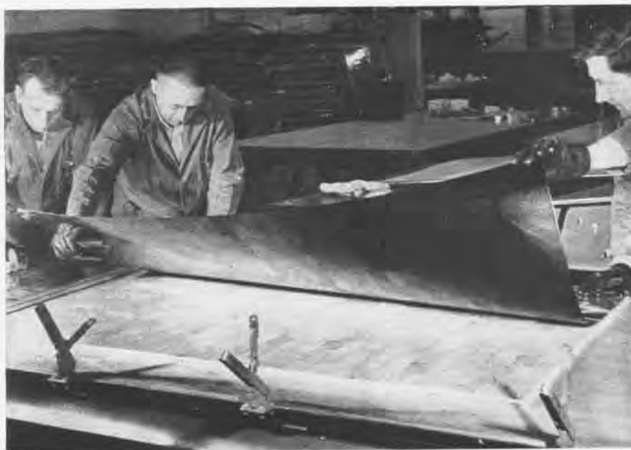
ALUMINUM ALLOY PLATE APPLIED TO CORE OF Balsa WOOD GIVES F6U GREAT STRENGTH
