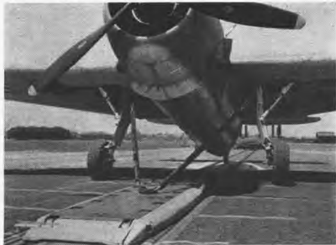
SADDLE FOR SLING CONNECTS TO UPPER PLATE OF SHUTTLE CAR
