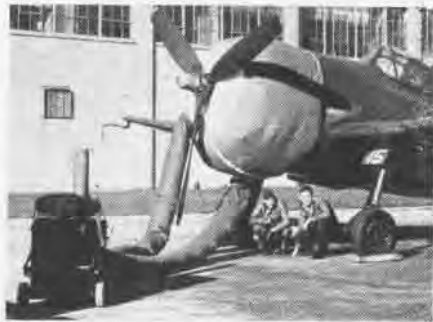
PRE-HEATER INSTALLED ON FRIGID F6F
