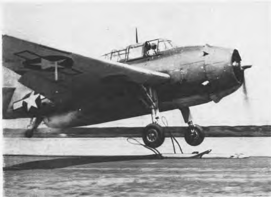
TBM, AT END OF ONLY 350-FOOT RUN, TAKES TO THE AIR; CAR IS STOPPED BY DC CURRENT
