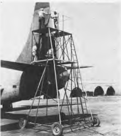
RUDDER REPAIR STAND HANDLES FOUR MEN
