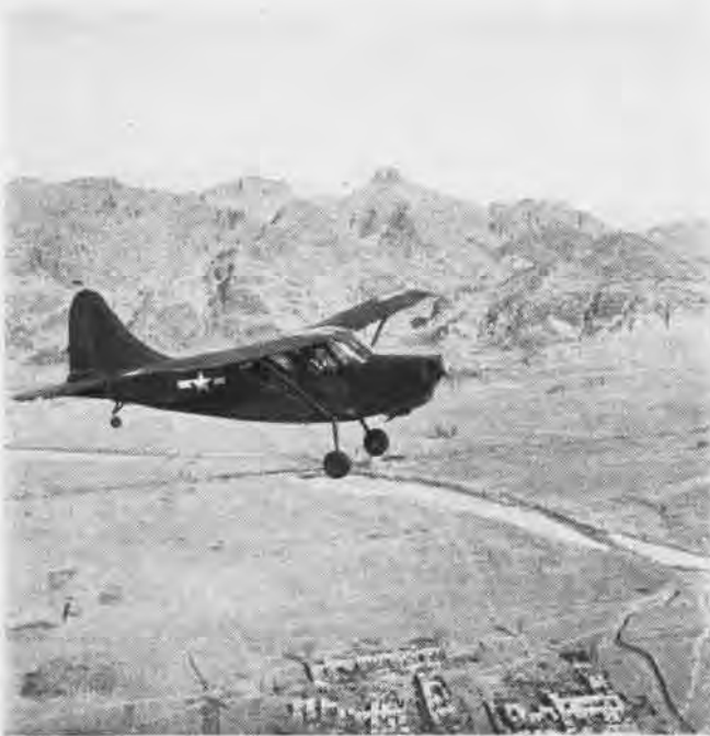
Marine OY on patrol in China is type used by tactical and gunnery observers to report on enemy forces and to direct, adjust gunfire
