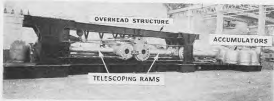
MOCKUP OF H8 CATAPULT SEEN BY VISITORS AT NAF'S OPEN HOUSE IN PHILADELPHIA
