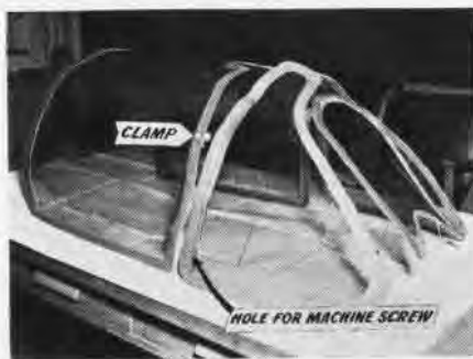
FOUR-PIECE HOOD FASTENS ON TIGHTLY
