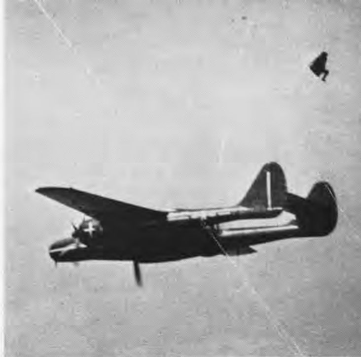
AAF'S SECOND EJECTION FROM P-51 SHOWS MAN HIGH OVER TAIL
