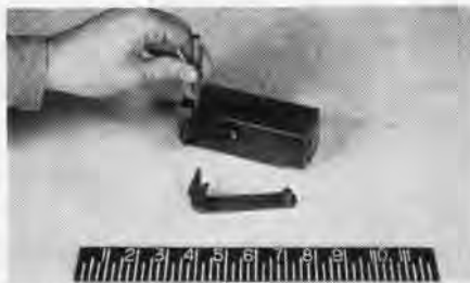
RECESSED BLOCK HOLDS THE EXTRACTOR
