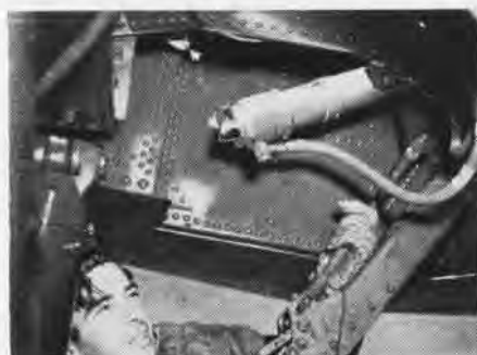
BROKEN ROD RESULT OF UPLOCK FAILURE
