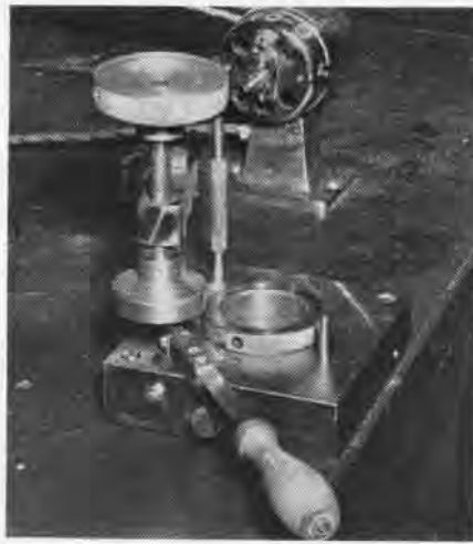
KNURLED BUSHING PERMITS A ROTATION
