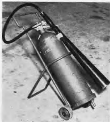
The aviation metal shop at NAS NEW ORLEANS A&R has manufactured eight fire bottle carts from an idea outlined in NAVAL AVIATION NEWS. It has been shown that the carts protect the CO 2 bottles from damage and improve the line appearance.
