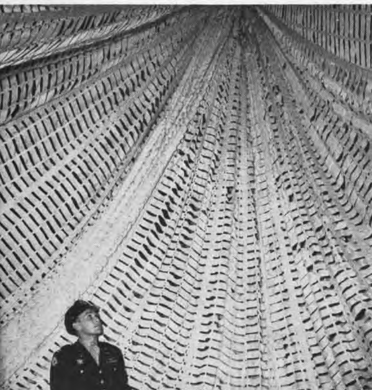
CAPTURED GERMAN DROGUE CHUTE USED TO BRAKE JET PLANES
