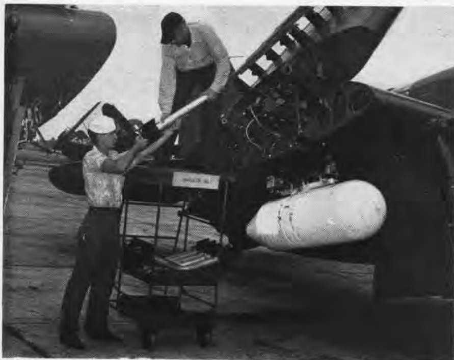
STAND ON CASTERS HELPS JAX ORDNANCEMEN LOAD SCARS ON WING RACKS OF HELLDIVER
