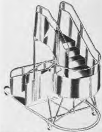
MARTIN RAMP HAS LIGHTS, SPIRAL STAIR
