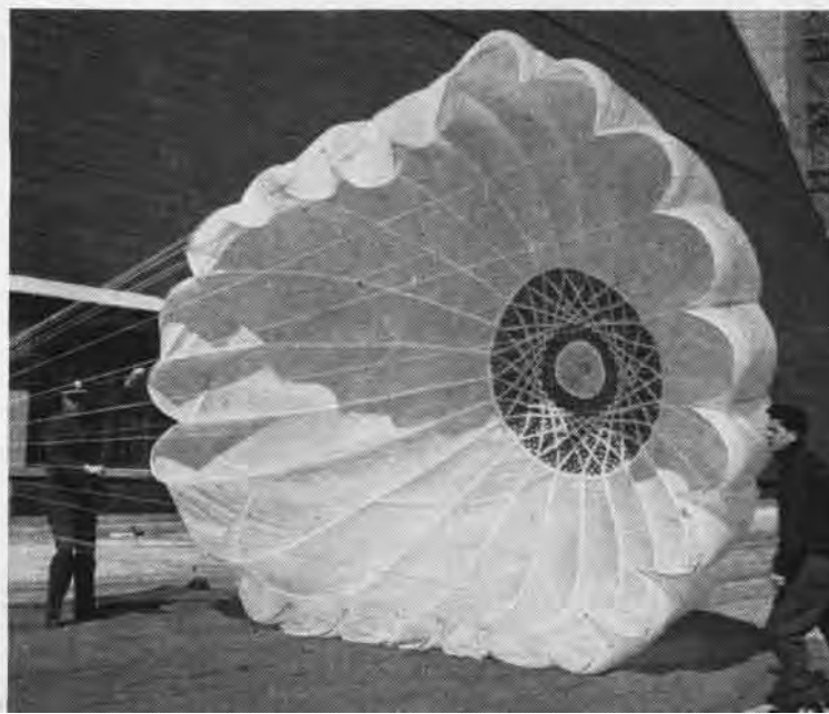
TWO EXPERIMENTAL CHUTES TESTED BY LAKEHURST PARACHUTE UNIT TO TEST AIR ESCAPEMENT THROUGH CHUTE'S CANOPY HOLES
