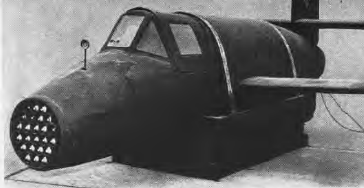
NAZI 'VIPER' HAD CHUTE IN TAIL; NOSE SECTION JETTISONABLE
