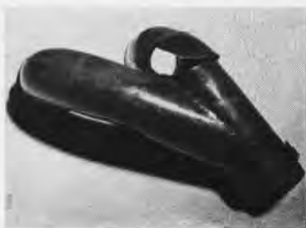
INTAKE BLEW THROUGH FAULTY STARTING
