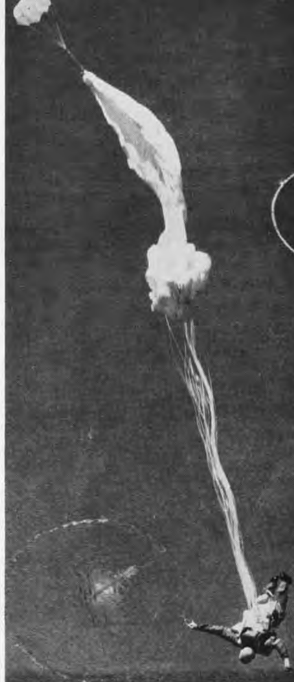
TWO EXPERIMENTAL CHUTES TESTED BY LAKEHURST PARACHUTE UNIT TO TEST AIR ESCAPEMENT THROUGH CHUTE'S CANOPY HOLES
