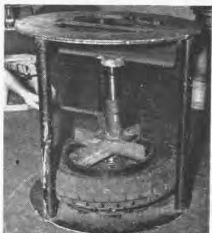
TIRE BEAD IS BROKEN ON BOTH SIDES AT ONCE
