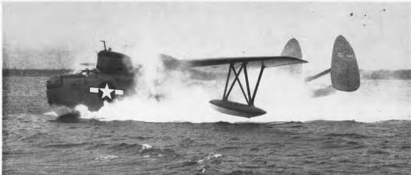
PBM-5 COMES TO A WATERY STOP AT NATC PATUXENT RIVER AFTER REVERSING PITCH OF PROPELLERS; LANDING RUN WAS CUT ABOUT 40 PER CENT
