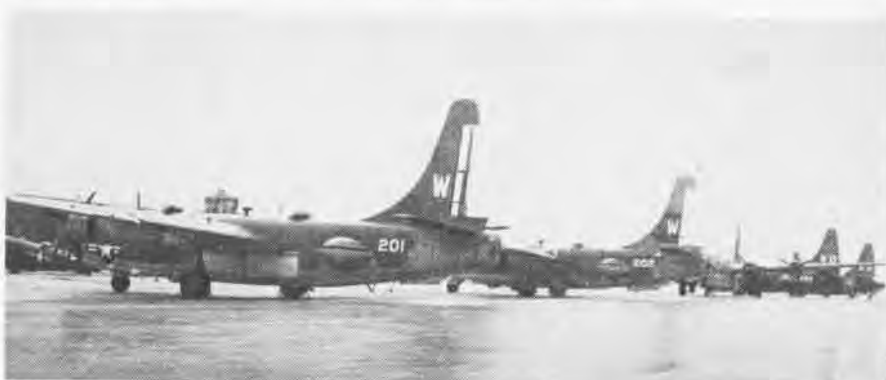
FIRST TWO AIRCRAFT WERE STRIPPED; THIRD FROM LEFT BROKE MOORINGS AND WEATHERCOCKED
