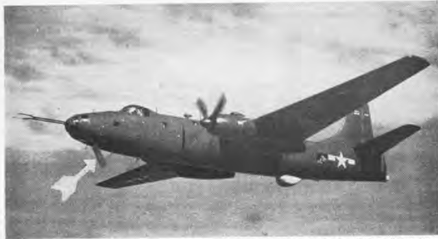
ABOVE PHOTO IS AN ARTIST'S CONCEPTION OF HOW EXTENDED HYDRO-FLAP WILL LOOK ON P4M-1
