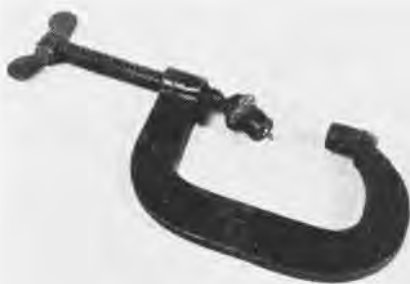
DIMPLING DIES ARE WELDED TO C-CLAMP JAWS
