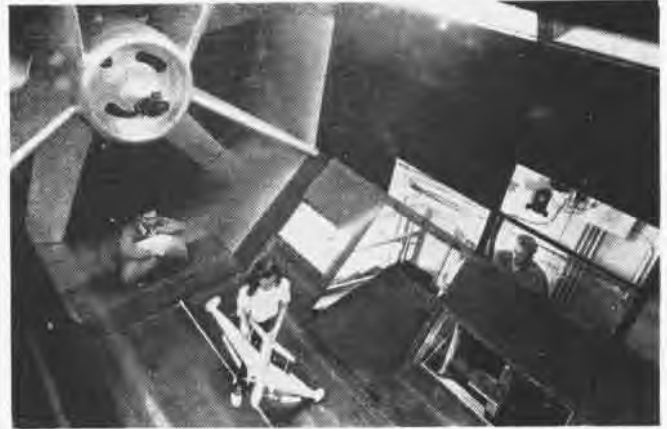
Inside view of free-flight wind tunnel shows pilot in cockpit and assistant adjusting plane of unusual design before flight
