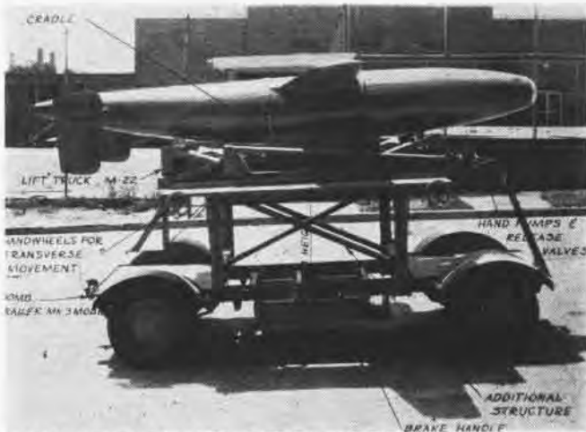
MOBILE LIFT IN COLLAPSED POSITION HAS 70-INCH MINIMUM HEIGHT
