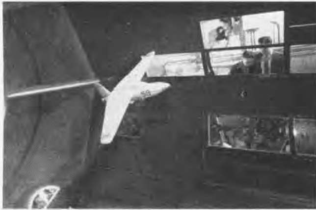
Model of a proposed fighter-type airplane undergoing flight test in the NACA free-flight tunnel at the Langley Laboratory
