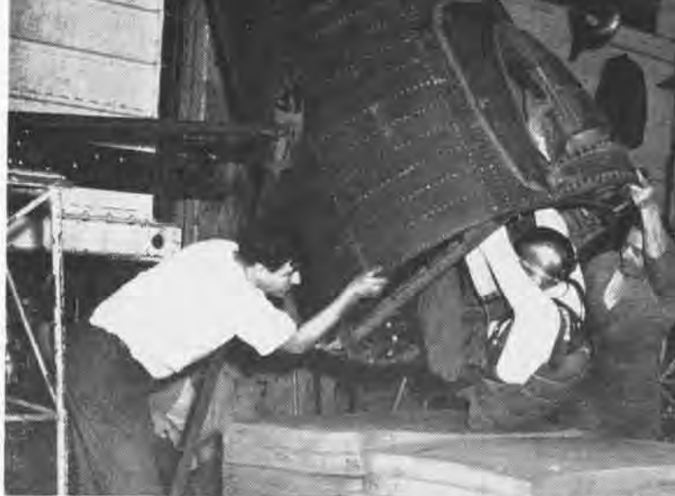
Russ Thaw, Douglas test pilot, tries out the escape mechanism as he drops from nose; decompression of compartment delayed
