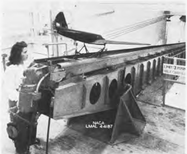
Models being tested in the 'gust-tunnel' are launched with this catapult at 100 mph, and flown through vertical gusts
