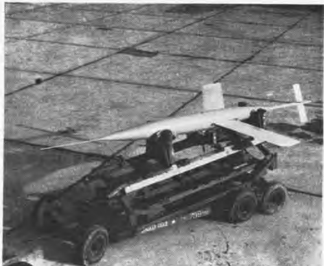
'Needle-nose' will be carried up to some 40,000 feet in B-29 where it will be dropped using NACA 'free-falling' technique
