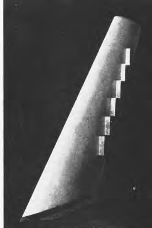
SPOILER TYPE AILERON EFFICIENT TO MACH .98
