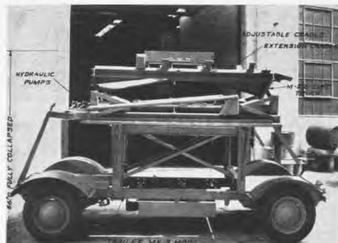
EXTENSION CRADLE RAISES COLLAPSED POSITION HEIGHT TO 86 INCHES
