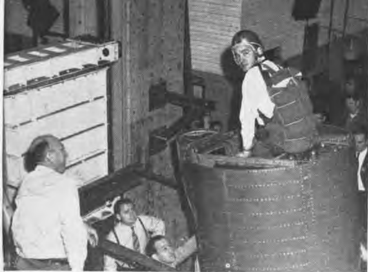
If in trouble, D-558 pilot pulls lever, dropping nose section off plane; he then releases seat, tumbles backward and uses chute
