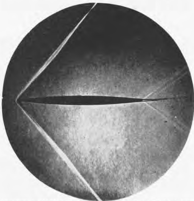
SCHLIEREN PHOTOGRAPH OF HIGH SPEED AIR FOIL AT THE SAME SPEED
