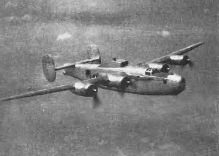
B-24 with jet engine installed in bomb bay sprays water into jet intake at high altitudes to test interior icing on turbine
