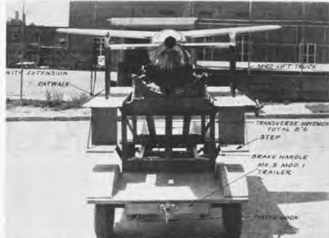
REAR VIEW OF MOBILE LIFT FOR PILOTLESS AIRCRAFT SHOWS CATWALK
