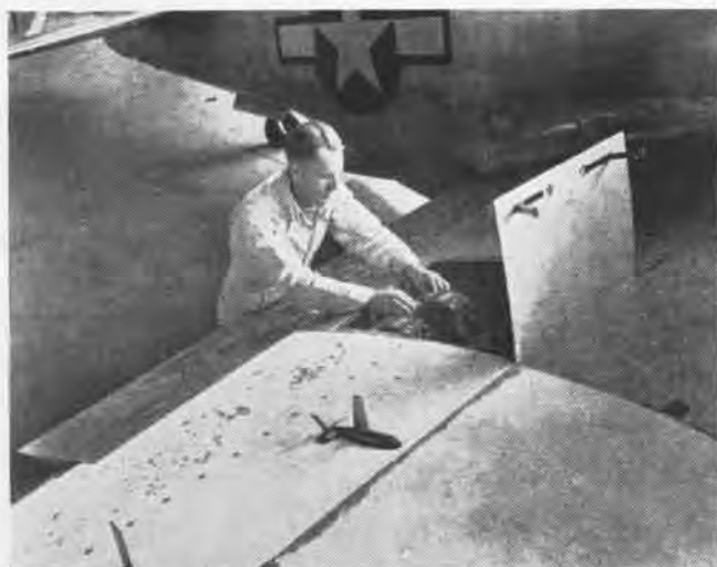
Instruments being installed in wing of a P-51 to measure forces registered on small-scale half fuselage used in flow test
