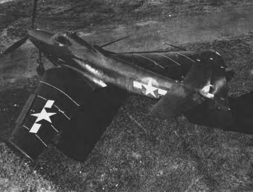
NAVY L-39 IS USED BY NACA TO STUDY SWEEP BACK WING STABILITY AND CONTROL PROBLEMS
