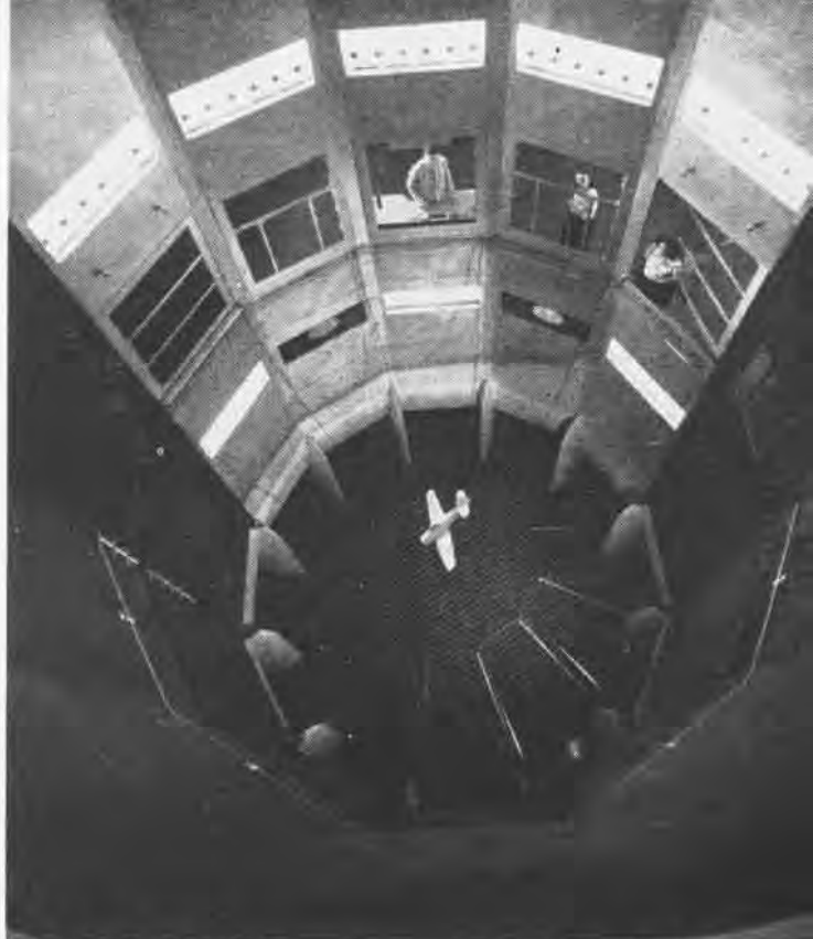
Model of SN2J in spin-tunnel is supported by the vertical air current while motion pictures are taken of plane's reactions
