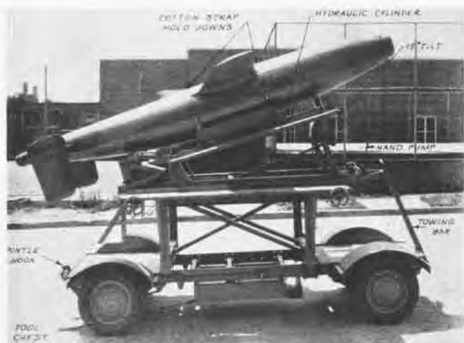
TILTING ANGLE UP TO 15 DEGREES IS REACHED BY USE OF HAND PUMP
