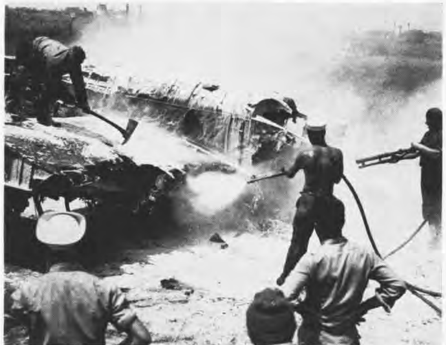
At the request of the New York City government, the Navy is training special airport fire fighting and crash crews at NAS Floyd Bennett Field, in a program to provide highly trained units to man the municipal airports—LaGuardia, Idlewild, Newark and Floyd Bennett. Here an instructor wields a crash axe to expose wing cells of the plane in an effort to release gasoline fumes. The Navy Mobile Fire Fighting Unit is from Memphis.
