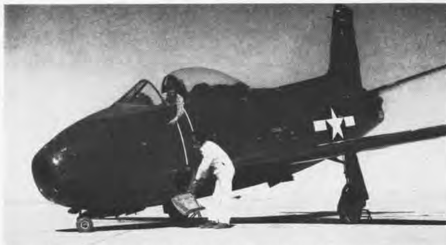
BENDING NOSE GEAR PERMITS NAVY'S XFJ-1 JET FIGHTER TO 'KNEEL DOWN' FOR EASY HANDLING
