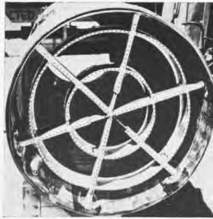
FUEL INJECTOR IN AFTER-BURNER INSTALLATION
