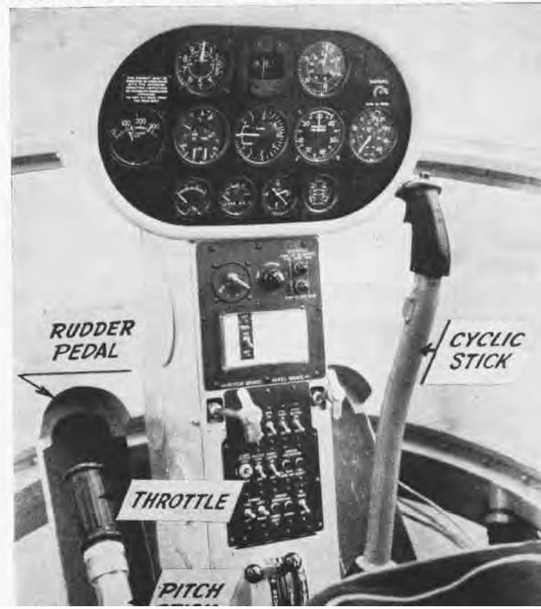
USUAL NEEDLE-BALL AND ARTIFICIAL HORIZON IS MISSING FROM PANEL
