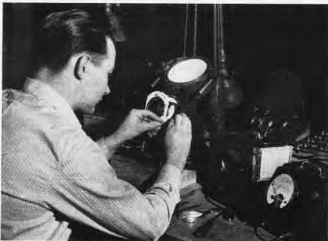
GUNSIGHT ASSEMBLY WORKER TESTS RELAY BOX ON SIGHTING SYSTEM
