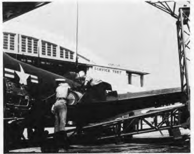
EASY ACCESS TO POWERPLANT IN WINGROOT SPEEDS UP ENGINE CHANGE
