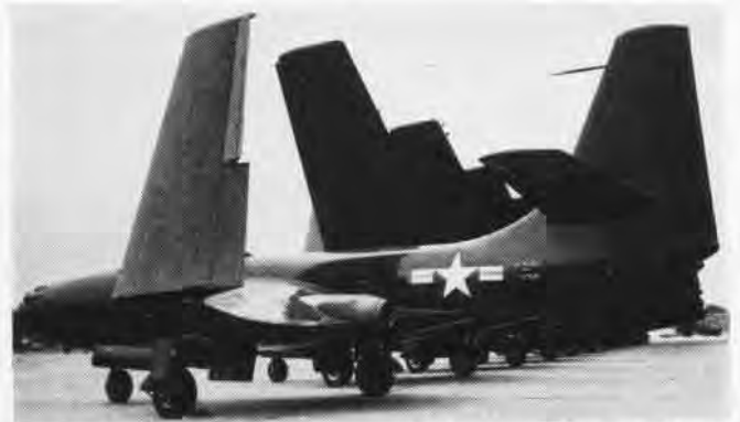
THE BANSHEE FOLDS ITS WINGS IN THE SAME MANNER AS THE PHANTOM
