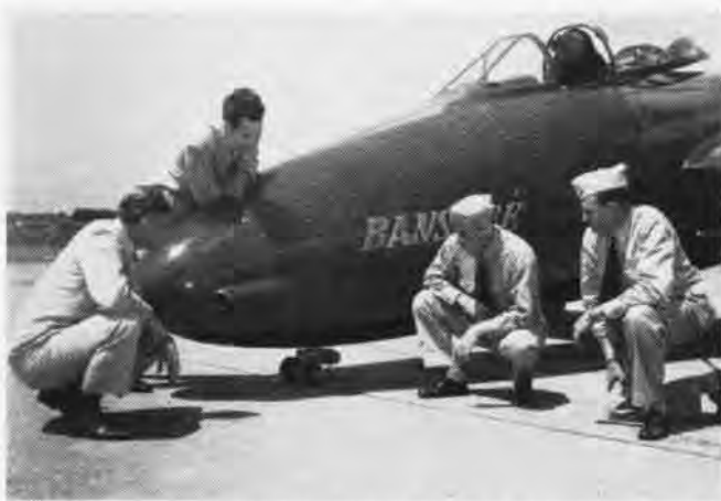
GUN PORTS ARE IN LOWER NOSE WHERE BLAST IS SHIELDED FROM PILOT
