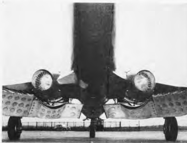
FLAPS EXTEND UNDER ENGINE AND ALMOST MEET UNDERNEATH FUSELAGE
