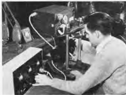
CHECKING RANGE UNIT ON MK 18 PLANE SIGHT
