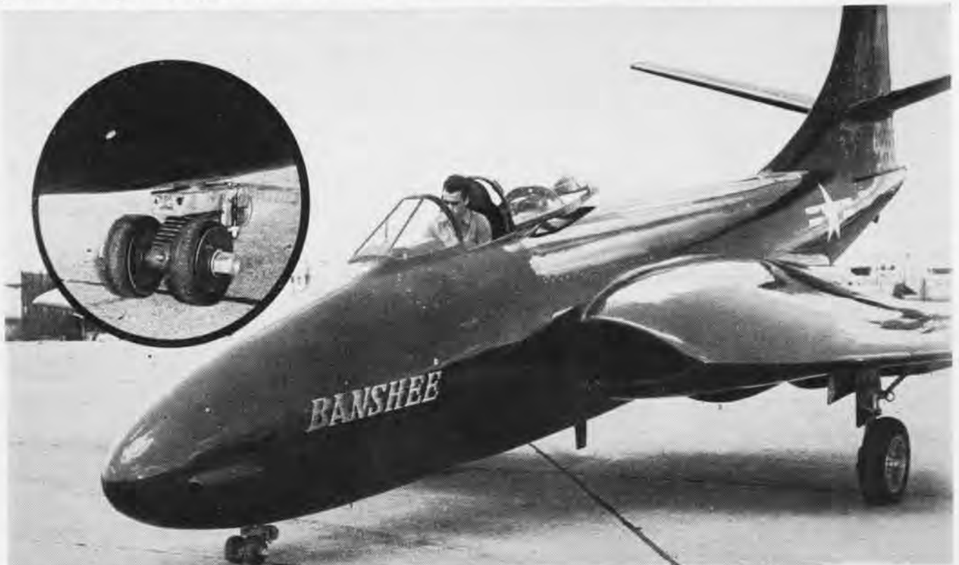
KNEELED ON A SPECIAL AUXILIARY CASTERING NOSEWHEEL THE XF2H-1 CAN FIT WELL UNDER THE TAIL OF ANOTHER SIMILARLY KNEELED BANSHEE
