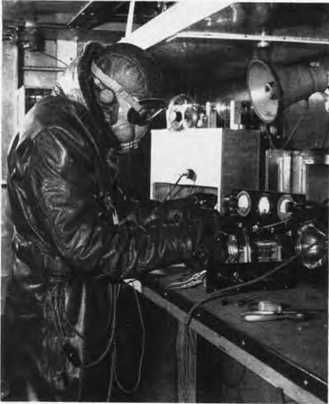
PRESSURE CHAMBER EMPLOYEE WEARS HEATED FLYING SUIT DURING TEST
