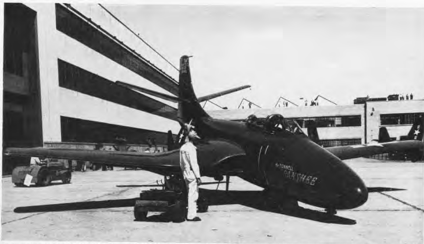
KNEELING ON ITS NOSEWHEEL THE BANSHEE CAN BE TAXIIED AROUND CARRIER DECK WITHOUT DANGER TO GROUND PERSONNEL FROM EXHAUST FUMES
