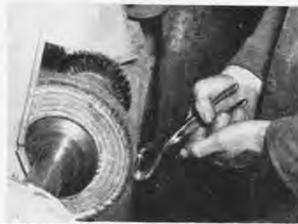
PLIERS ALLOW ROCKER ARM SHAFT TO ROTATE
