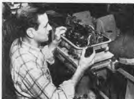
SETTING CAGING SYSTEM ON MK 14 GUN SIGHT
