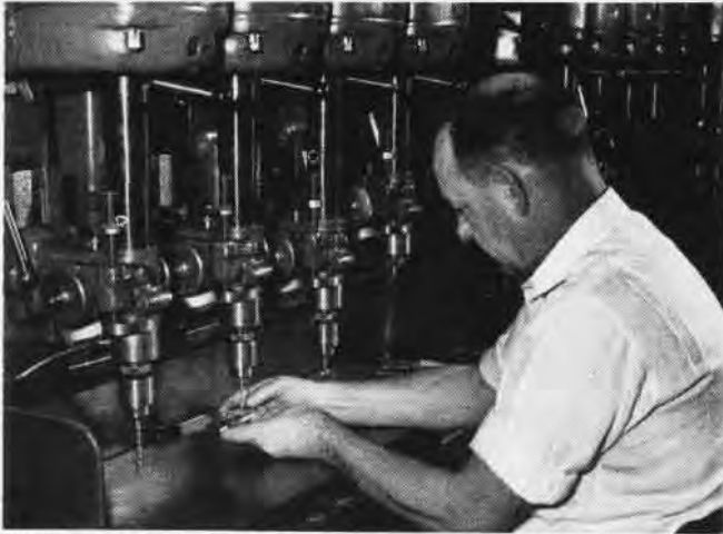
WORKER USES DRILL PRESS TO BURR BRACKET ON A MK 18 GYROSCOPE
