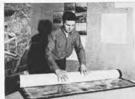
5 Last print of mosaic is laid on aircraft cloth with gum solution
