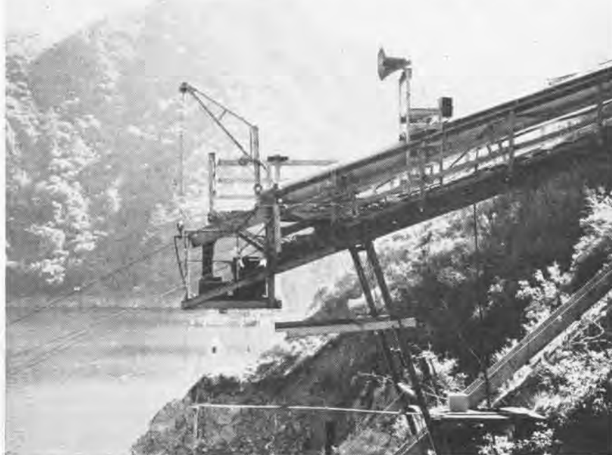
FIXED-ANGLE LAUNCHING TUBE AT MORRIS DAM TEST RANGE HAS FIRED OVER 3000 TORPEDOES
