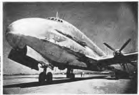
PRODUCTION MODELS OF F2H-1 AND F9F-2 WILL BE EQUIPPED WITH COCKPIT PRESSURIZING UNITS; CONSTITUTION IS PRESSURIZED THROUGHOUT
