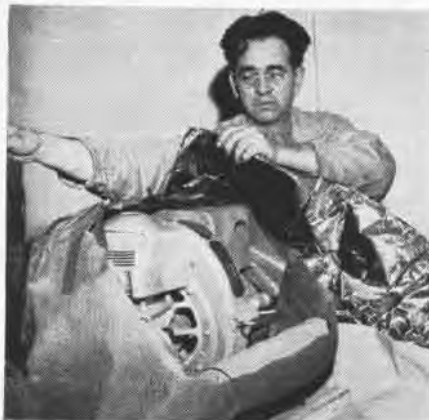
Generator is wrapped with moisture-proof non-corrosive foil for storage
