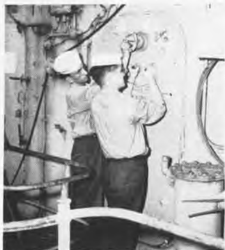
F. Burns, AA, and R. Gortz, AA, remove metal seal through which D/H pipes ran
