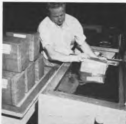
Packages of aviation material are wax-dipped for more complete protection
