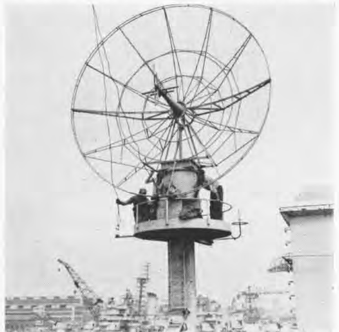
Workers at Philadelphia Naval Shipyard reinstall Cabot's radar screen used by CIC for air search; ship laid up 2 years
