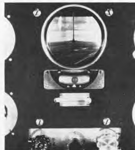
NEW ATTITUDE INDICATOR HAS FIXED HORIZON
