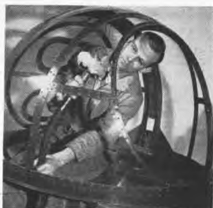
Turret plexiglas is polished prior to the application of a plastic coating
