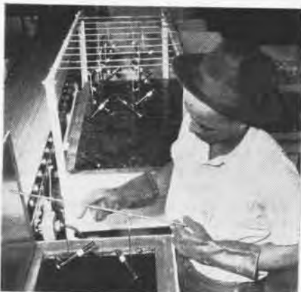
Final stage of the preservation process for aircraft valves is plastic dipping
