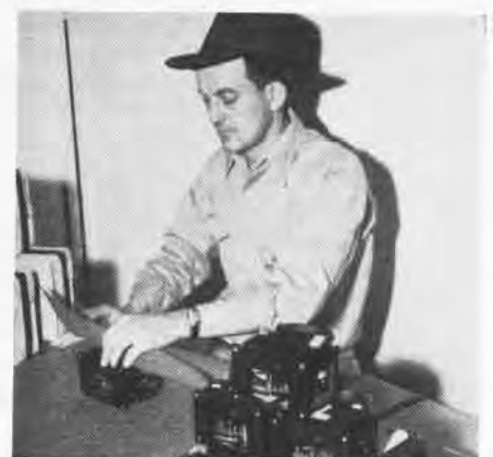
Aviation compasses are given their first wrapping in a non-corrosive paper
