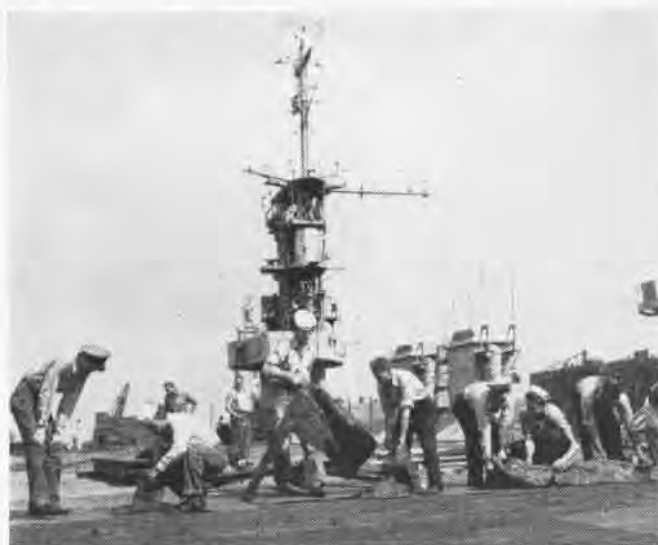
Crew of Cabot removing Komul deck covering from ship's long-unused flight deck, preparing her to go back on duty
