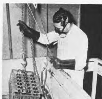
Aircraft valves are degreased in a vapor bath at the start of preservation
