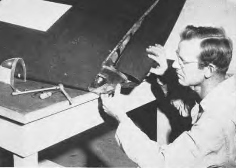
Aviation items needing minor repairs are put in shape before preservation; here a wing tip is receiving attention
