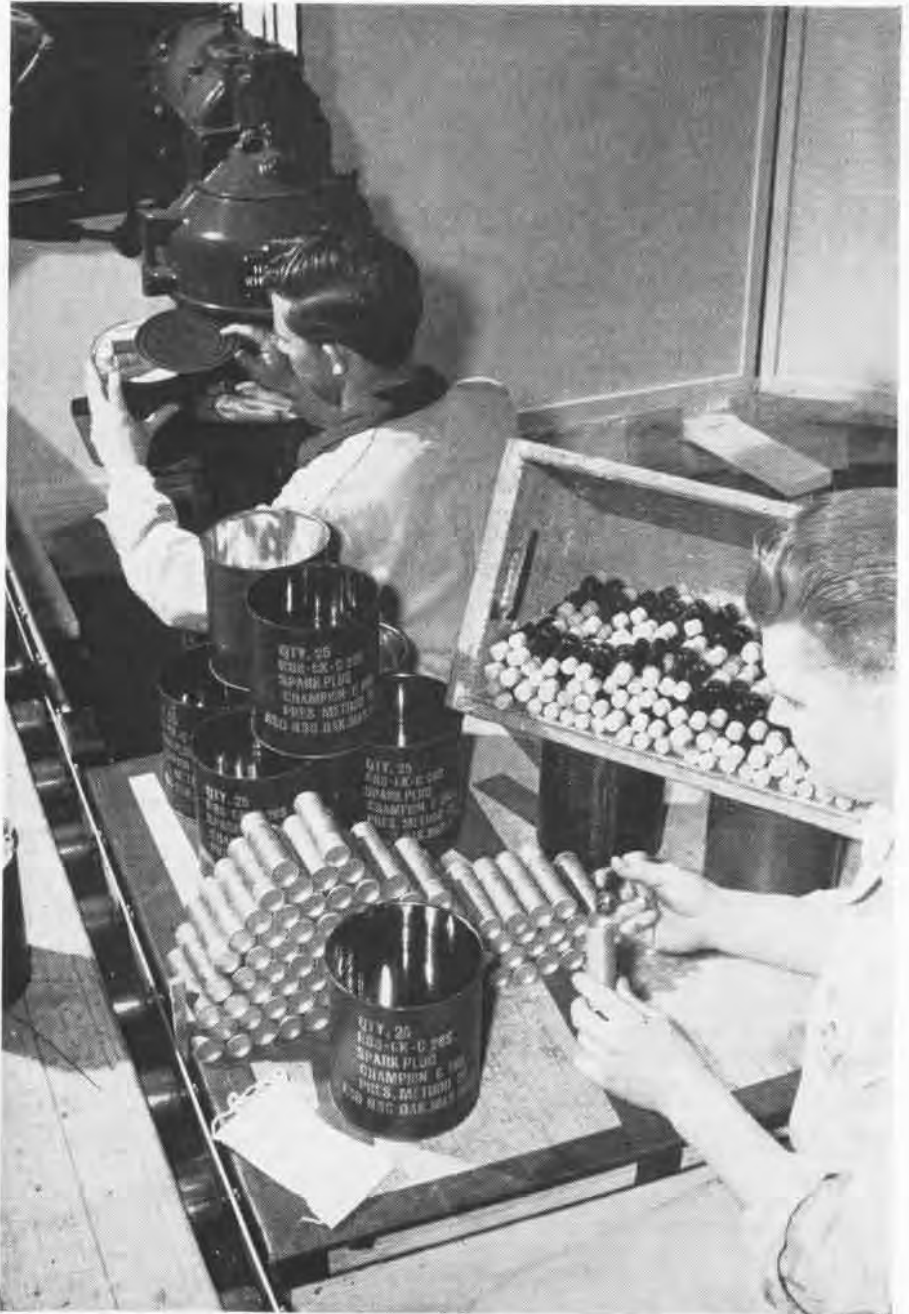
Spark plugs are expensive and subject to rapid deterioration but canning protects them; note stock numbers and other data printed on cans for ready identification
