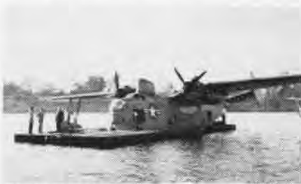
NYLON PONTOONS WILL MAKE A PORTABLE SLIP wide on both sides of the plane and about 18'x25' at the bow of the plane.
