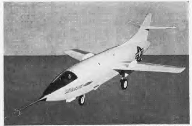
AIRSCOOPS CAN BE CLOSED FOR EVEN MORE STREAMLINING IF DESIRED
