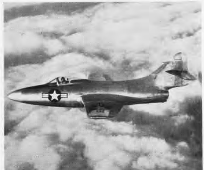
GRUMANN XF9F-2 IS NEWEST IN NAVY JET FIGHTER LINE, HAS NENE ENGINE
