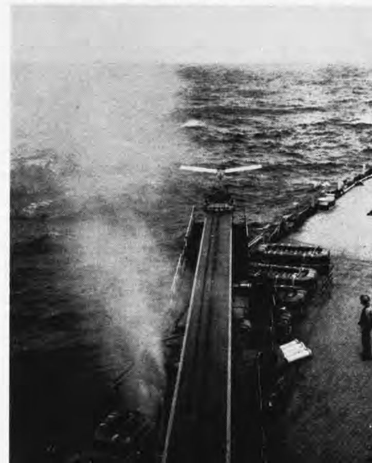
Catapult launches a TDD for gunnery work-out. Drones require a naval aviator to operate the remote control "stick"
