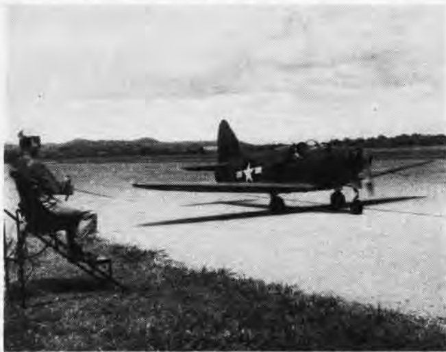
FOX CONTROL AND TD2C DRONE; PILOT 'RIDES' ON PRELIMINARY TESTS
