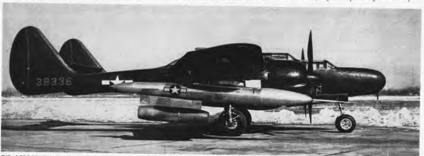
THE GORGON IV IS LAUNCHED AT A FLIGHT SPEED OF MACH .5 AT WHICH SPEED THE RAM-JET HAS SUFFICIENT THRUST TO ACCELERATE MISSILE
