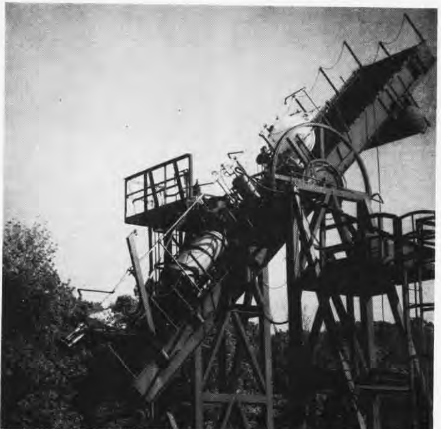
A6000C4 ROCKET MOTOR COMPLETE WITH PROPELLANT TANKS MOUNTED ON MOVABLE TEST STAND
