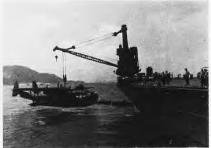
AN AVP PUTS MARINER BACK IN THE WATER AFTER REPAIRING HER HULL
