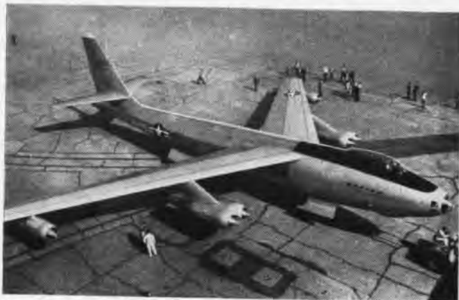
XB-47 —Swept-back wing and tail surfaces make this slim jet Boeing bomber easy to spot, as does 6-jet engine placement
