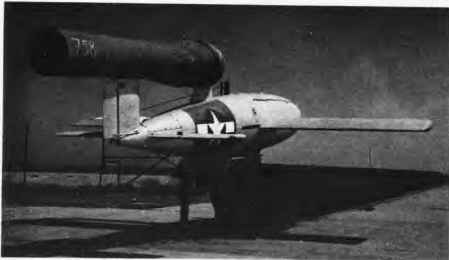
LOON GUIDED MISSILE, PATTERNED AFTER V-1 BOMB, READY TO LAUNCH ON XM-1 AT PT. MUGU
