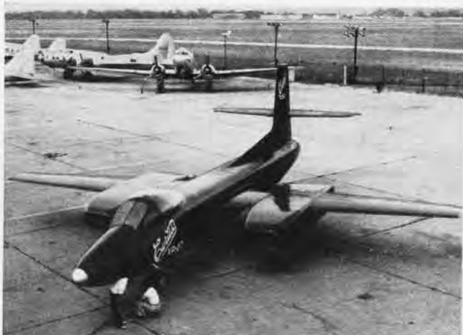
XP-87 —First four-jet fighter is this Curtiss plane with 60-foot span. Two-man craft designed for extreme weather work
