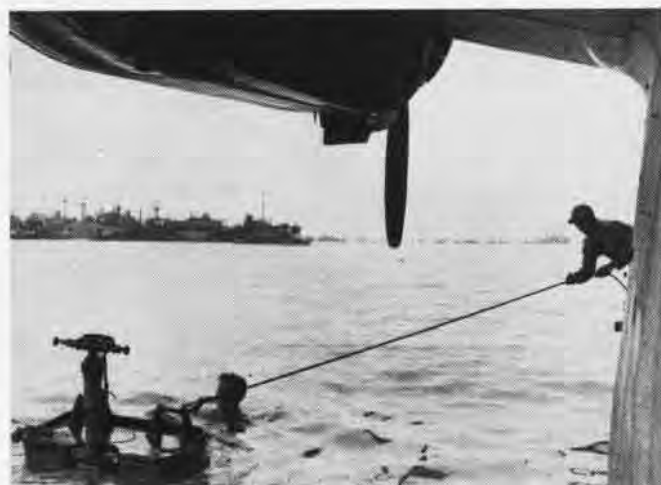
BUOYANCY CHAMBERS KEEP SIDE-MOUNT AFLOAT WHILE BEING MOUNTED
