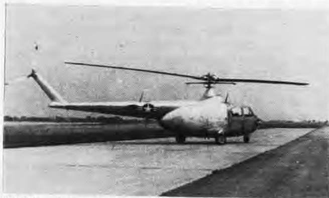
XR-12 —A five-place helicopter by Bell, capable of 105 mph top speed. It has 300-mile range, climbs 450 feet a minute
