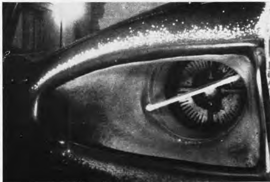
ICE COAT NEARLY BLOCKS AIR INTAKES ON VANES OF ENGINE AFTER IT HAD RUN 23 MINUTES
