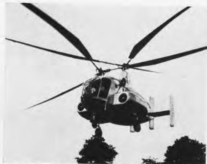
XR-10 —This odd-looking helicopter can carry 10 persons; its two rotors intermesh, each powered by separate engine
