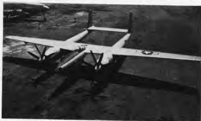
XF-11 —This Howard Hughes reconnaissance plane looks like a king-size P-38, carries six cameras in nose and booms
