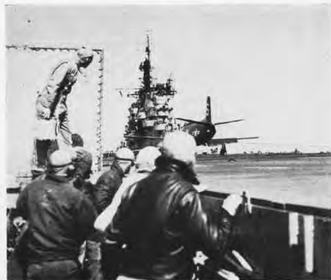
LSO and his assistants peer to see the Fury catch second wire during its qualification landings aboard the CV Boxer
