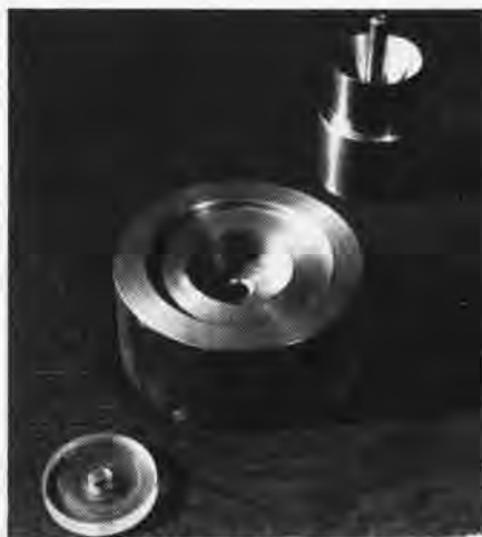
GAUGE, CUTTING TOOL FOR OFF-SIZE GASKETS
