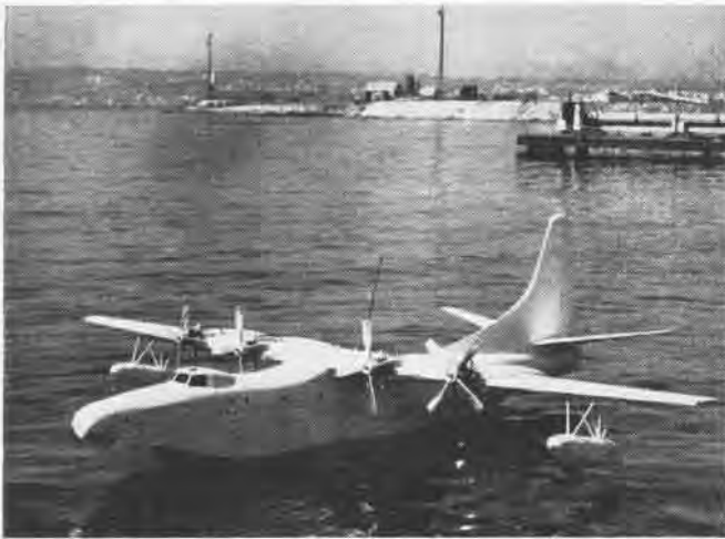
FOUR TWO-HP ENGINES DRIVE THIS SLEEK EXPERIMENTAL PLANE MODEL
