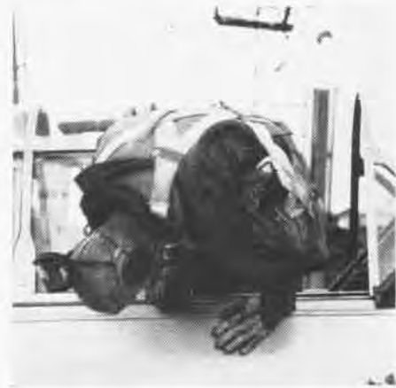
THIS PILOT HAS CORRECT METHOD OF BAILOUT
