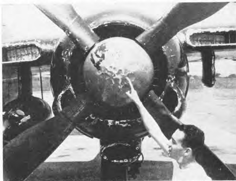
PROPELLER HUB SHOWS WHY HAIL WAS MAINTENANCE BOTHER ALTHOUGH NOT TOO HAZARDOUS
