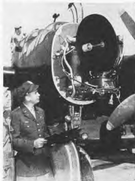
RADAR GEAR IS HOUSED IN NOSE OF THE PLANE
