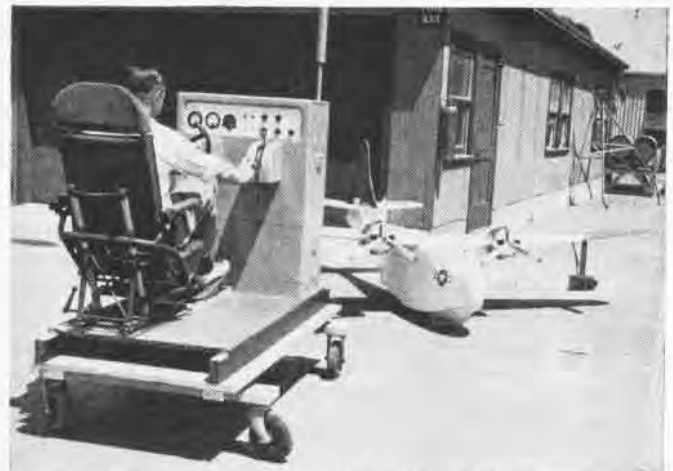
SEVEN-CHANNEL RADIO CONTROL PANEL HANDLES PLANE WHILE IN AIR
