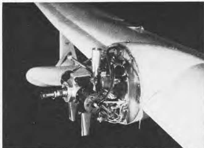
TWO HP ENGINE ATTACHES TO NACELLE JUST LIKE ON A BIG PLANE
