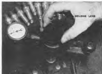
LENS CUTS DOWN ON INTENSITY OF PLUG SPARK
