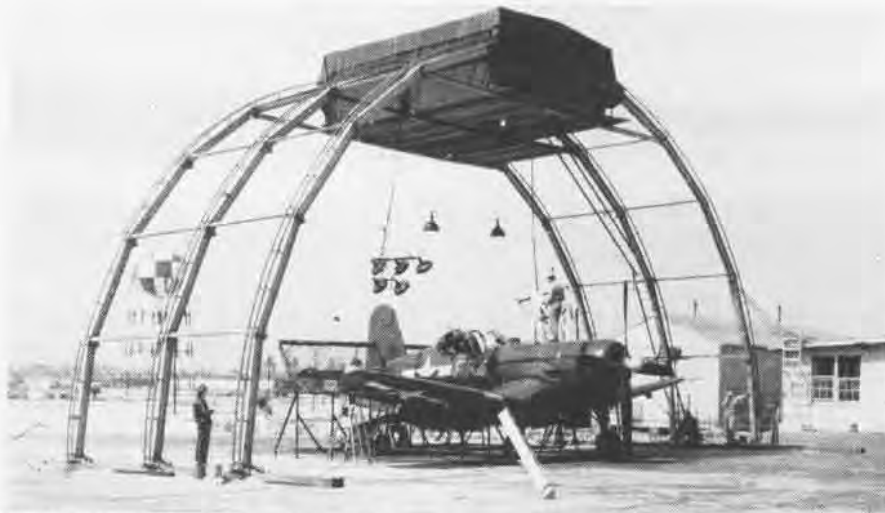
CORSAIR ANCHORED UNDER FLOODLIGHTS FOR TESTS; CAMERAS WERE INSTALLED ON TOP HANGAR
