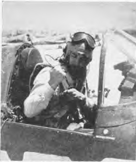
DISCONNECT EARPHONE CORD TO PREVENT JERK
