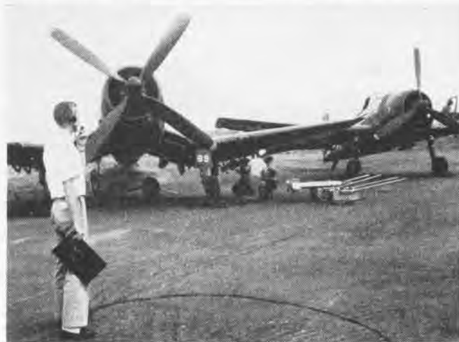
Ordnancemen demonstrate arming of rockets on Corsair while assistant producer Paul Birthgrath describes operation
