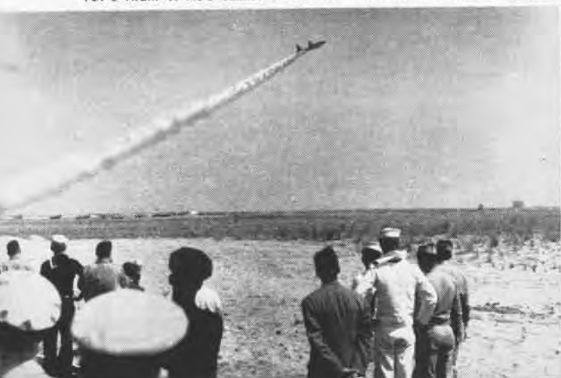
P2V-2 FROM VP-ML-8 CLIMBS STEEPLY OVER IDLEWILD BY USE OF JATO
