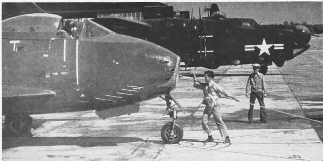
'GUINEA PIG' AT PATUXENT, SECURED BY ANCHOR LINE AND CHUTE HARNESS, TESTS 38-KNOT SUCTION TWO FEET AHEAD OF FJ-1 JET INTAKE
