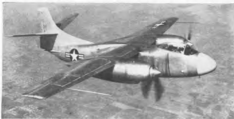
XAJ-1, NAVY'S BIGGEST CARRIER-TYPE PLANE, HAS TWO CONVENTIONAL ENGINES, JET IN TAIL
