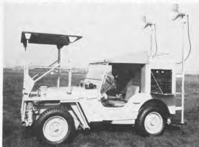
TYPE 'E' ALL-PURPOSE JEEP HAS HYDRAULICALLY OPERATED WORK STAND
