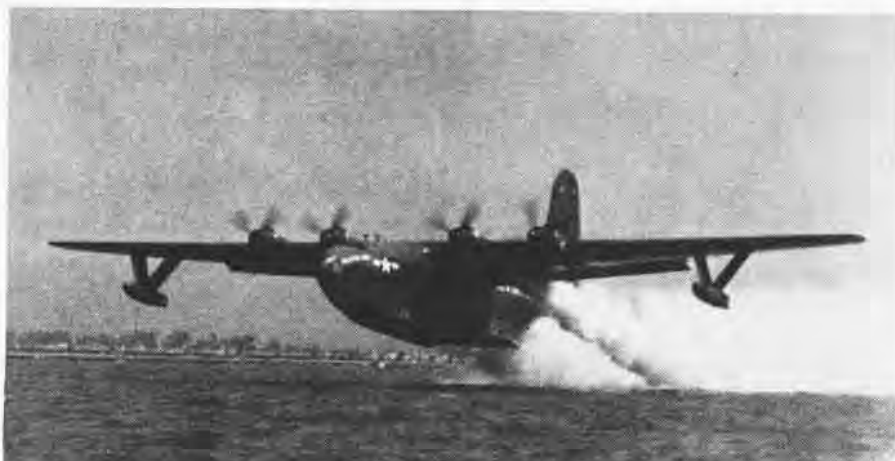
JRM MARS HAD BEST HYDRODYNAMIC PERFORMANCE OF THE THREE FLYING BOATS TESTED
