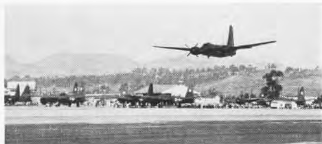
One propeller feathered, with less than 100 feet altitude, a P2V-2 demonstrates its single-engine performance at Miramar
