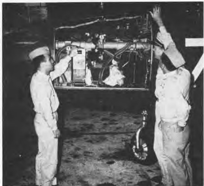
Recorder installed in Phantom's nose helps keep data on the plane in flight; students fly planes as well as study books
