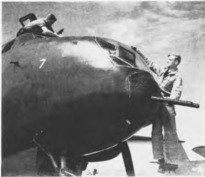
Blunt-nosed P2V-1 with twin .50 cal guns is being prepared for flight by W. E. Williams, AL2, and I. W. Peters, ALC
