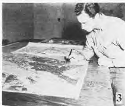
Pictures show steps in making the relief map at NAS DENVER—First S. Slocum and Lt. Lanisus discuss patterns to be traced from the basic map. Next Slocum carefully cuts out the patterns which have been copied onto the wax. In picture three, he melts down the layers of wax to form mountains and ridges. Finally Slocum and D. Maddox even up the contours on the map, as Captain H. L. Hoerner, commanding officer of the naval air station, looks on approvingly.
