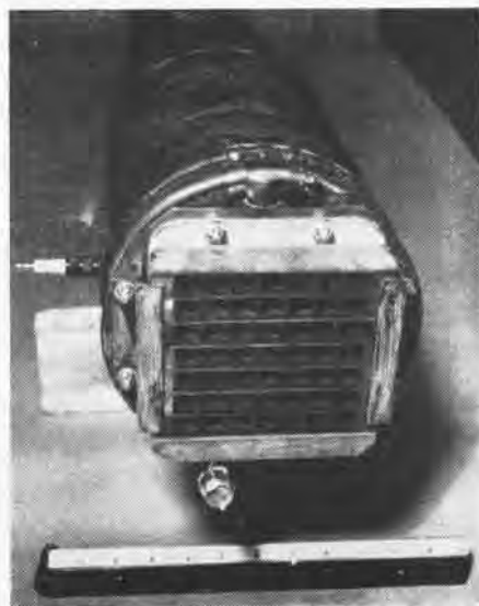
VALVE BANK OF MCDONNELL 8-INCH PULSEJET
