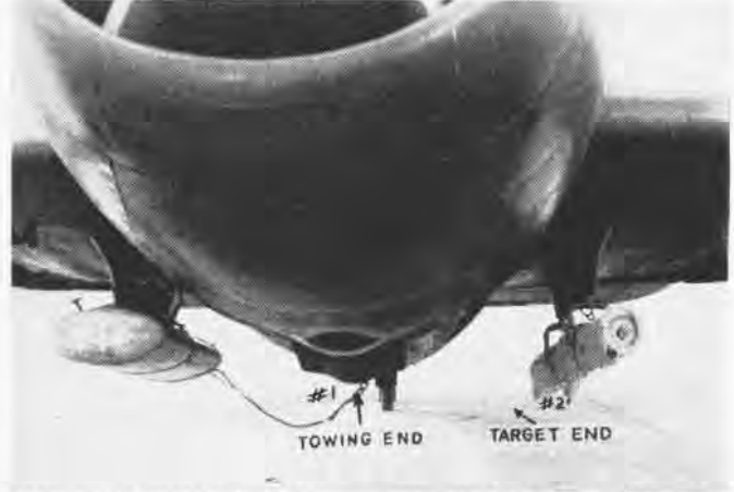
CAN ON LEFT HOLDS TOW CABLE, WITH BANNER ROLLED IN BRACES, RIGHT
