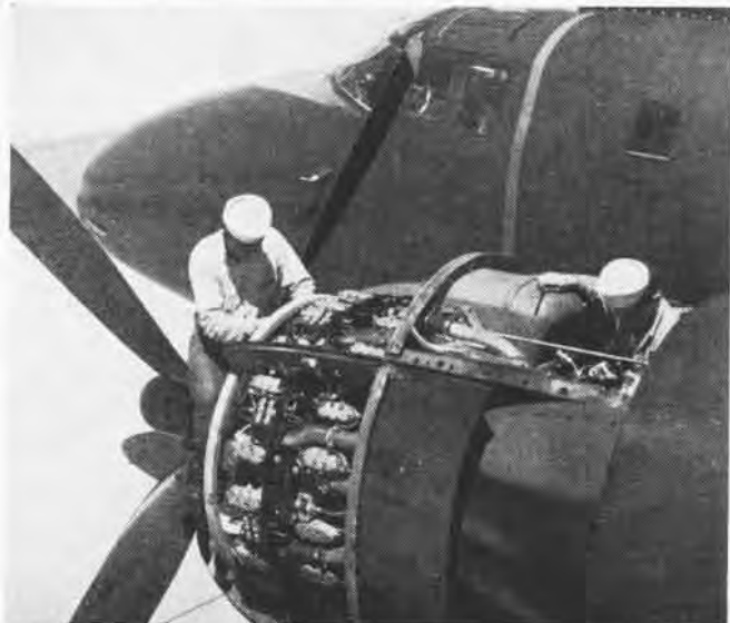
Propeller governor adjustment is made by Angelicchio, AD2, ML-4 as Moreau, AD3, gets inside nacelle to fix carburetor
