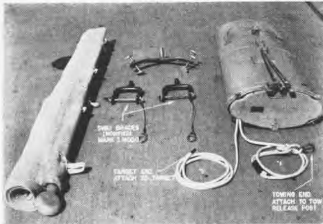
THESE MATERIALS MAKE UP NEW BANNER LAUNCH SYSTEM ON CV PLANES
