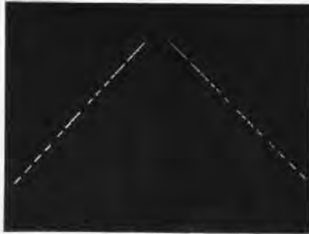
ON TOO HIGH APPROACH LINES ARE BROKEN
