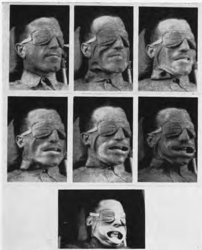
What slipstream from 275 to 310 mph does to a pilot's face is shown by test photos by NAMC PHILADELPHIA photo lab
