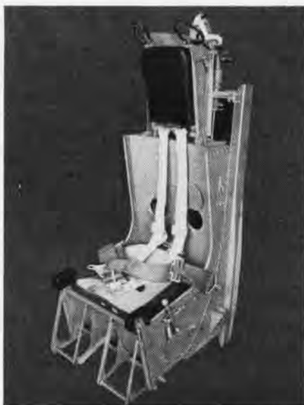
Grumman—This ejection seat will be put in F9F Panther for emergency use
