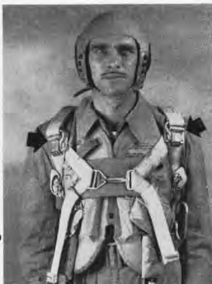
QUICK-DETACHABLE CANOPY RELEASE ON PILOT
