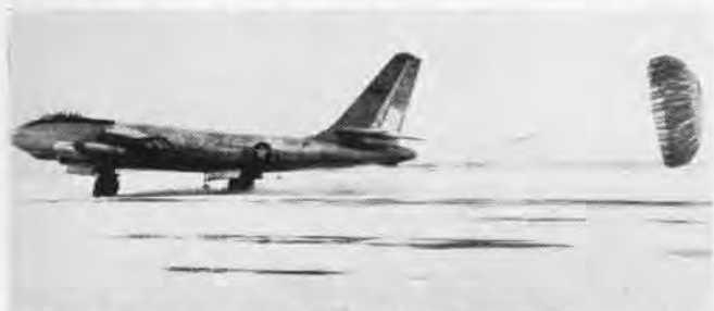
BOEING XB-47 USES 30-FOOT DROGUE CHUTE TO SLOW LANDING SPEED
