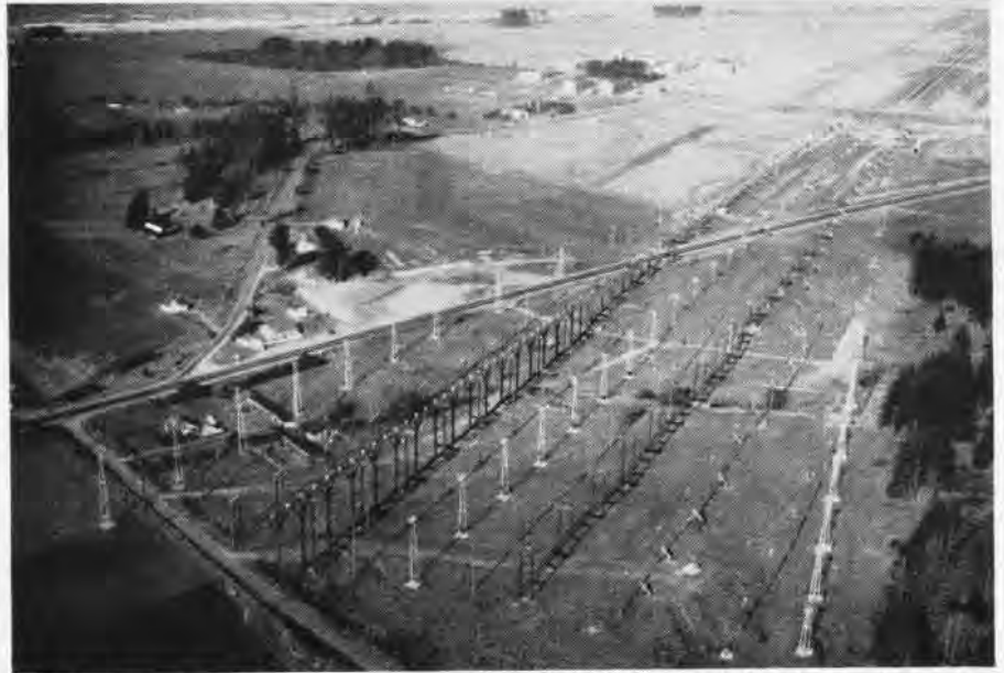
APPROACH LANE AT ARCATA IS CLUTTERED WITH VARIETY OF LIGHTING SYSTEMS UNDER TEST
