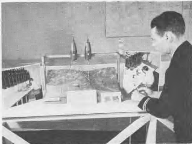
BAUSCH AND LOMB MULTIPLEX PROJECTOR PLOTS ELEVATED LAND
