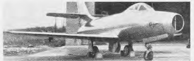
FRENCH MD 450 OURAGON FEATURES CLEAN DESIGN, HAS NENE ENGINE
