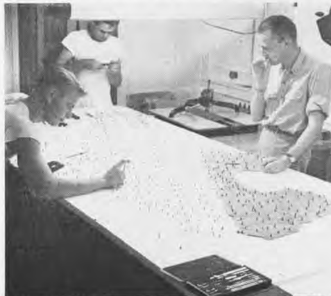
SLOTTED TEMPLATES ARE USED TO LOCATE LANDMARKS ACCURATELY
