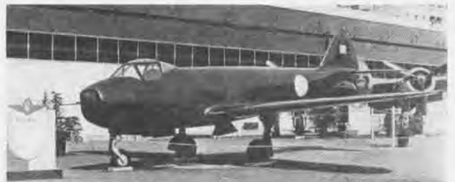
SMALL, HIGH TAIL, HOG-NOSE AIRSCOOP FEATURE ARGENTINE PULQUI
