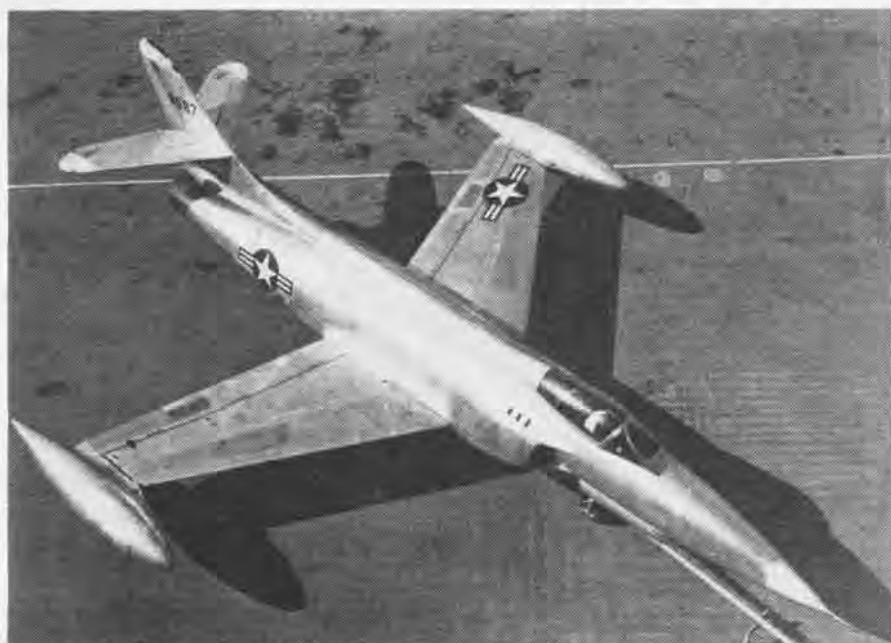
LONG-NOSED LOCKHEED PENETRATION FIGHTER, XF-90, HAS AFT-LOCATED TWIN JET ENGINES
