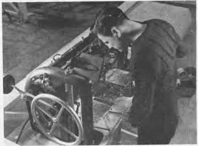
LEAST EXPENSIVE MACHINE FOR PLOTTING CONTOURS IS THE KEK
