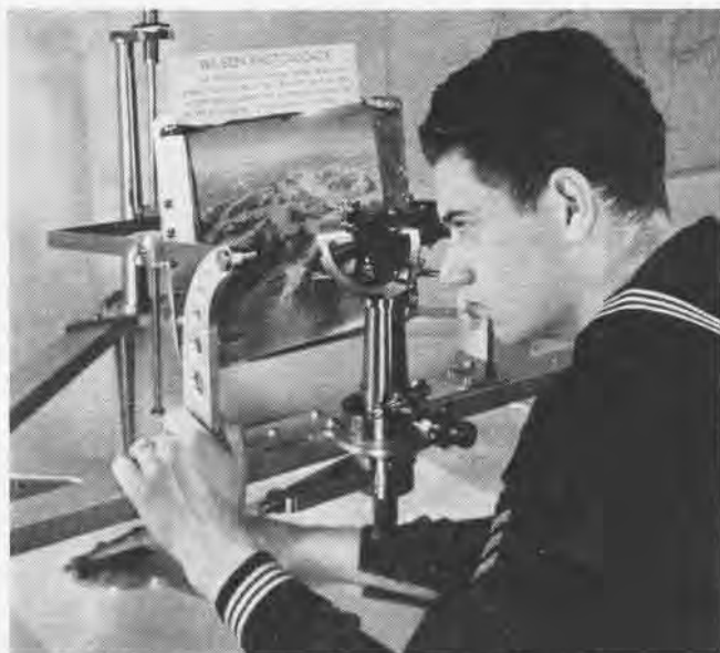
PHOTOALIDADE GETS DIRECTION AND ELEVATION FROM OBLIQUE PHOTOS
