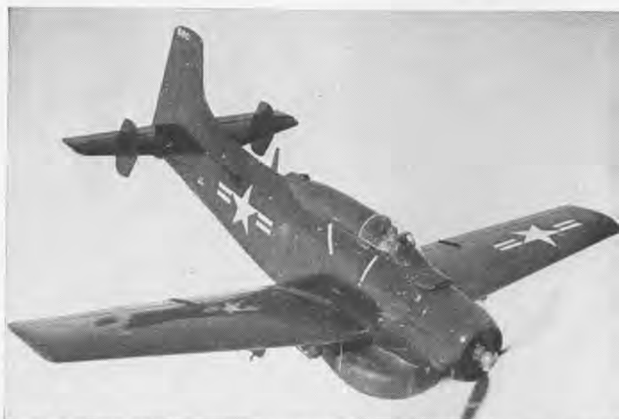
Hardly recognizable as the famous Douglas Skyraider is the strange-looking plane above with the three tails, odd canopy and bulbous radar guppy on its belly. This AD-3W version of the Skyraider, in production at El Segundo the past three years, carries the new look in airplanes to a new extreme. Extra rudders help give the plane more flying stability.
