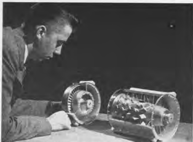
SUPERSONIC COMPRESSOR ON LEFT EQUALS PRESSURE RATIO OF OTHER
