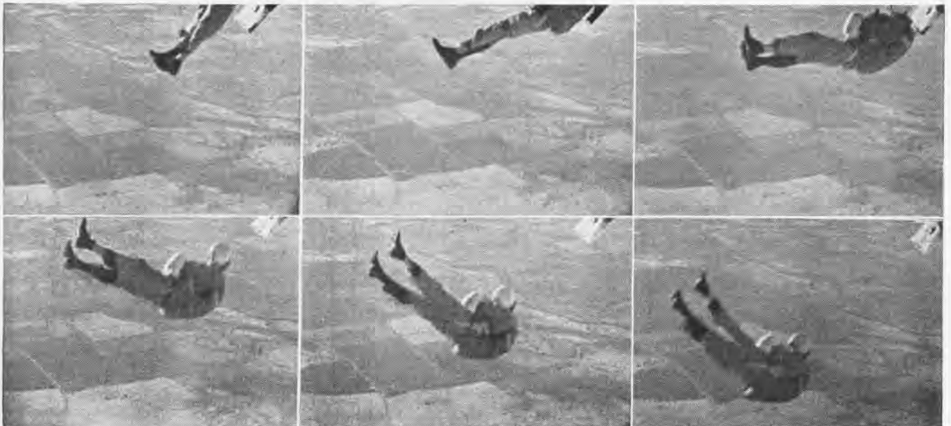
SEQUENCE OF PICTURES TAKEN FROM CAMERA LOCATED IN WING OF XF3D SHOWS JUMPER AND AUTOMATIC SLIPSTREAM SHIELD AT BOTTOM OF CHUTE
