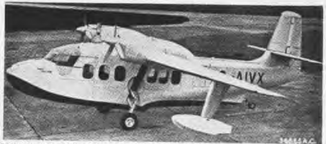
BRITISH SEALAND DESIGNED FOR USE ON SMALL LAKES OR AIRFIELDS
