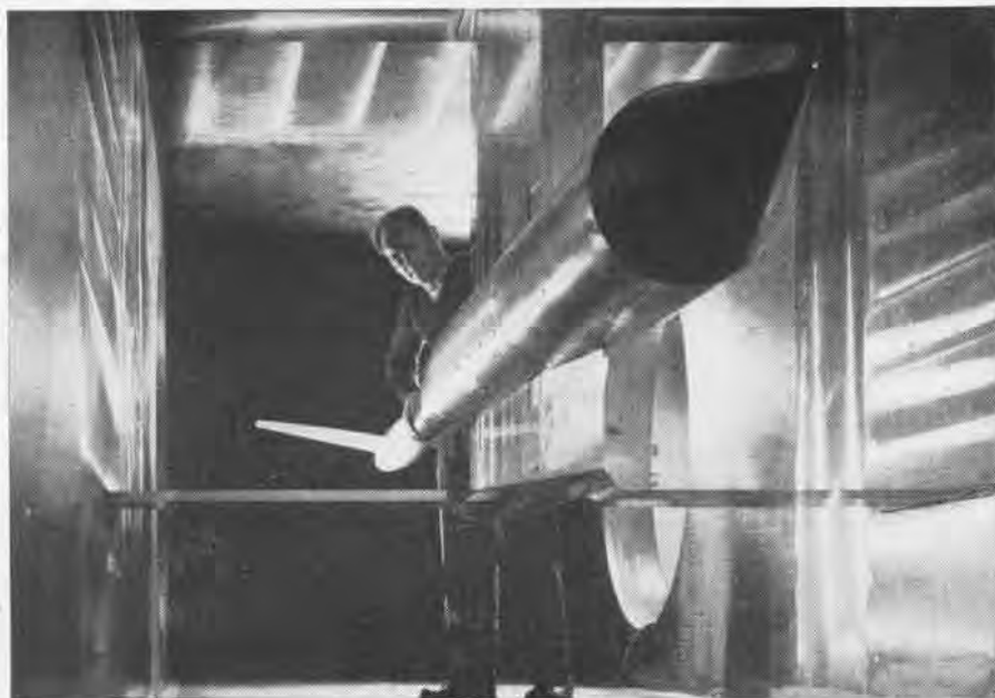
NOT A NEW DESIGN BUT A REAR VIEW OF A MODEL SUPPORT IN THE SUPERSONIC WIND TUNNEL
