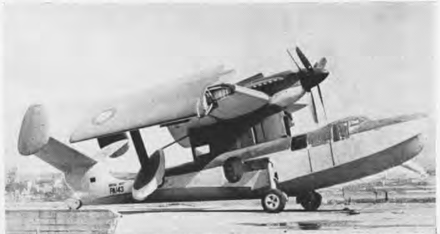
BRITISH SEAGULL UNIQUE AMONG AMPHIBIANS WITH FOLDING WINGS, COUNTER-ROTATING PROPS
