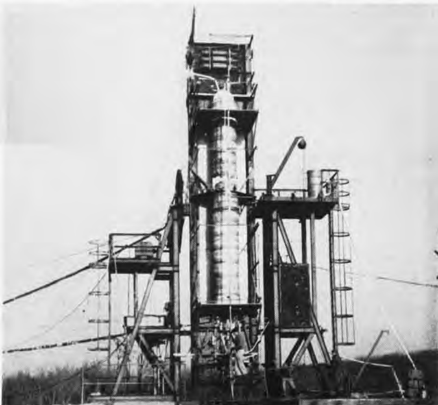
REACTION MOTORS TEST PLATFORM TRIES OUT ROCKET ENGINE WHICH WILL DRIVE NAVY'S VIKING
