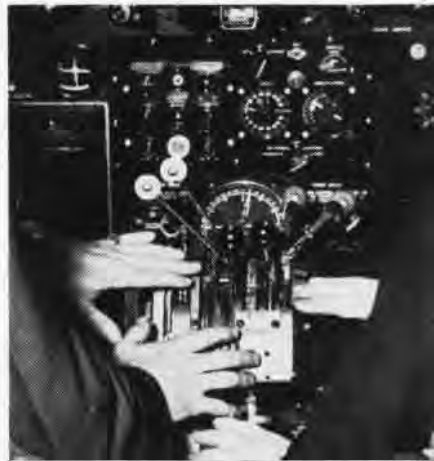
AUTO PILOT ADDS 140 LBS. TO PLANE WEIGHT
