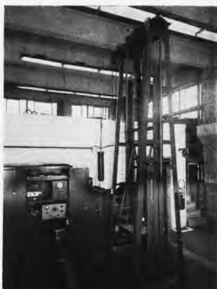
IMPACT MACHINE SIMULATES SHOCK OF CRASH
