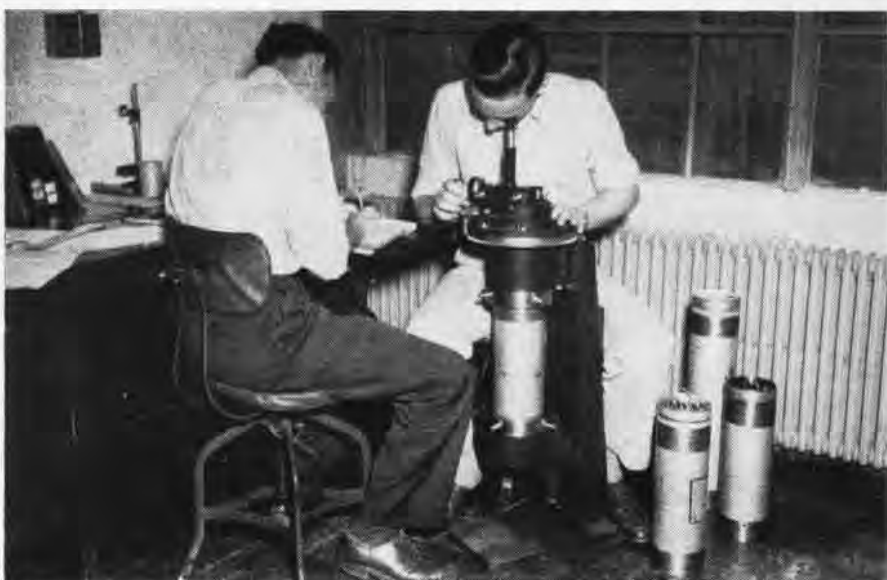
TECHNICIANS AT THE NAVAL GUN FACTORY CHECK ROCKET MOTORS WITH A MALALIGNMENT GAGE
