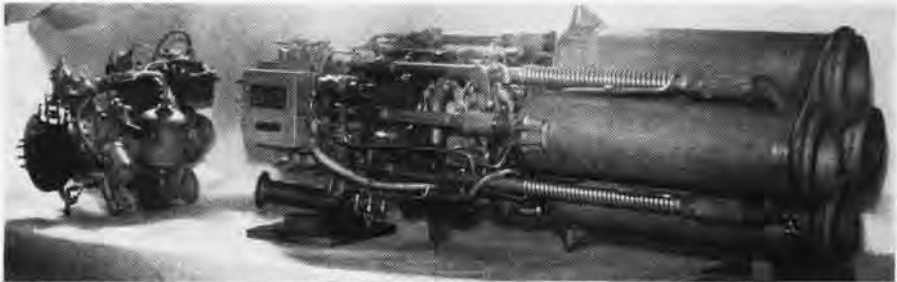
GERMAN ENGINE ABOVE USED PRESSURE FEED SYSTEM; AMERICAN A6000C4 USES NEW FUEL PUMP
