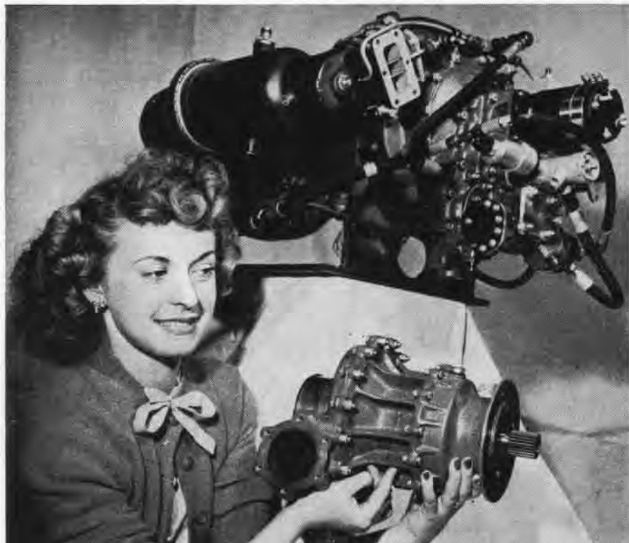
AIRESEARCH WORKER HOLDS PART OF 88-POUND SELF-STARTER FOR JET ENGINES IN NAVY PLANES
