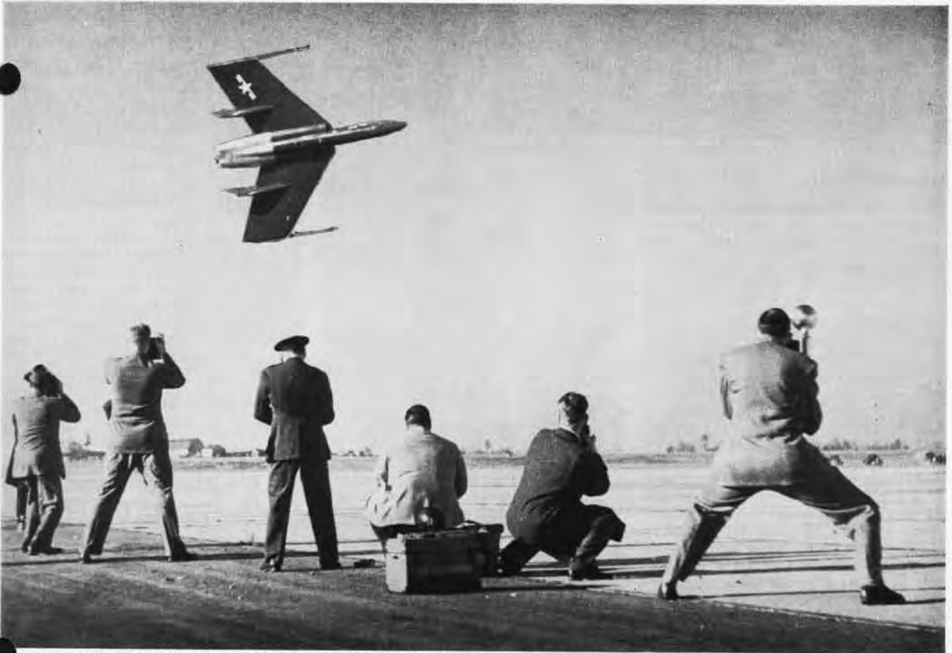
IN JETS, LONG PITOT TUBES AND WHEEL WELLS IN RUDDERS PLAINLY VISIBLE IN THIS SHOT OF F7U-1 FLYING PAST NEWSPAPER PHOTOGRAPHERS
