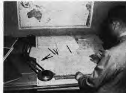
Data from Sofar receivers are plotted to obtain fix on location of explosion
