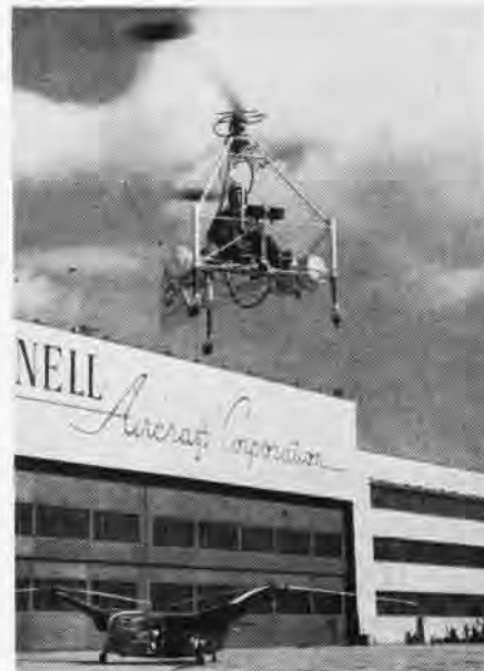
Hovering over the Navy XHJD-1 helicopter in front of McDonnell Aircraft plant in St. Louis is the Air Force's "flying test stand," the world's first ramjet helicopter, Little Henry. The HJD, still in the manufacturer's hands, is the first two-engined helicopter, either of which can drive both rotor blades if needed
