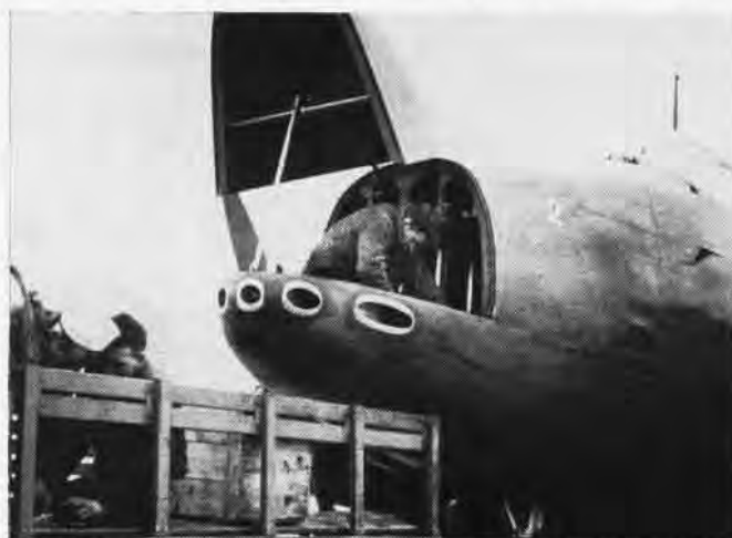
P2V-2 HAS SIX 20 MM. CANNON IN FIXED NOSE INSTALLATION TO STRAFE
