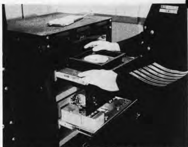
CHRONOMETER TIMES SOFAR IMPULSES ON TAPE TO GIVE BLAST DISTANCE
