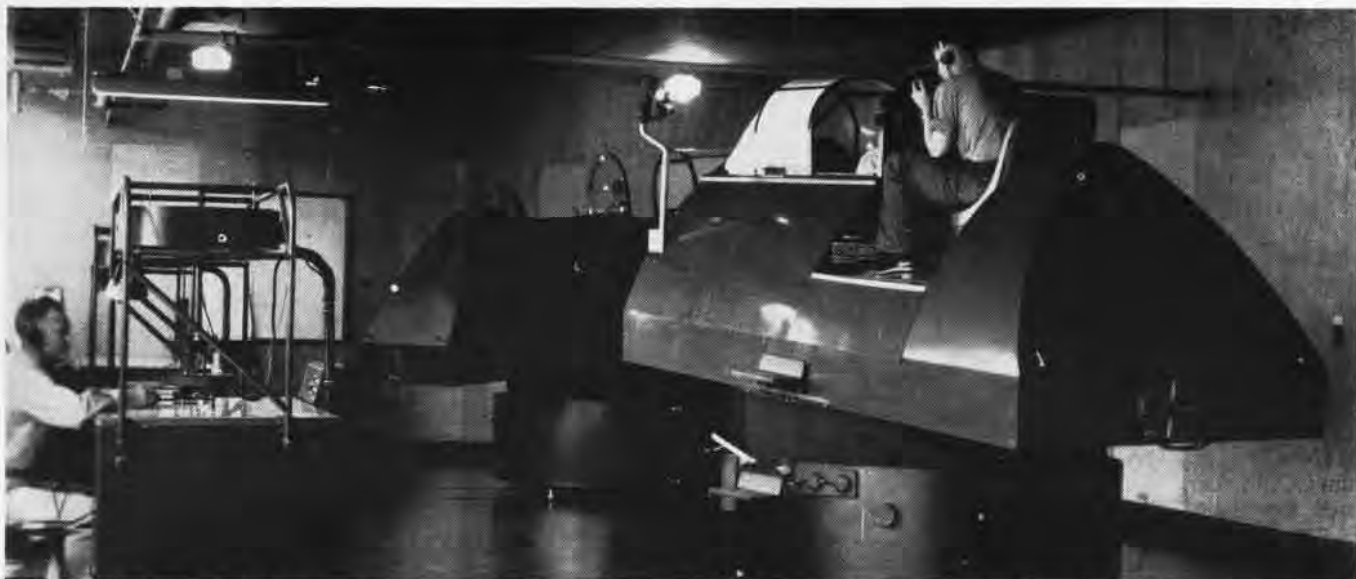
F8F FIGHTER TRAINER AT NAS ALAMEDA IS USED TO TEACH PILOT HOW TO NAVIGATE ON INSTRUMENTS; 'CRAB' ON LEFT PLOTS HIS MANEUVERS
