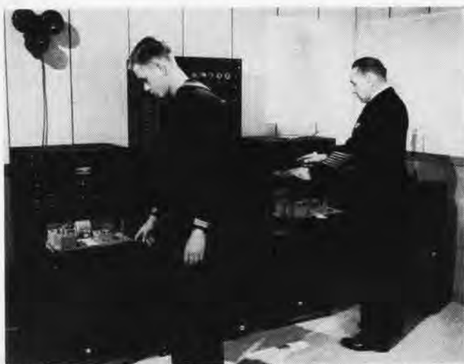
INCOMING SOFAR SIGNAL RECORDS ON PAPER TAPE AT MONTEREY STATION
