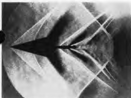
AIRFOIL PHOTOGRAPHED IN SUPERSONIC TUNNEL
