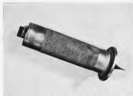
NEW PORTABLE TESTER FOR AIRCRAFT FABRIC
