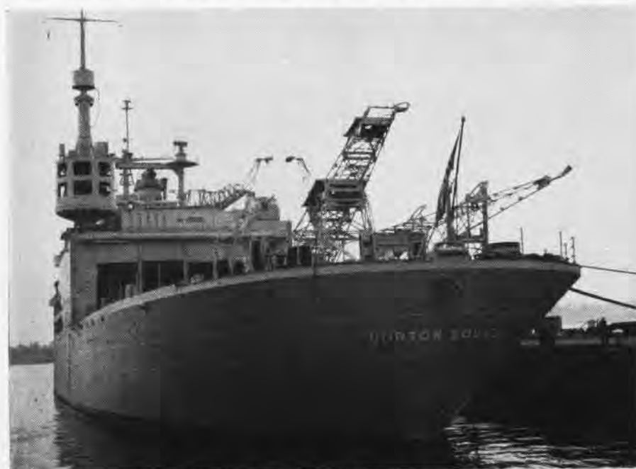
JUMBLE OF EQUIPMENT ON FANTAIL OF NORTON SOUND IS FOR LAUNCHING VARIOUS MISSILES
