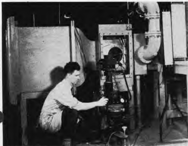
SCHLIEN PHOTOGRAPHIC SET-UP WITH SMALL SUBSONIC WIND TUNNEL
