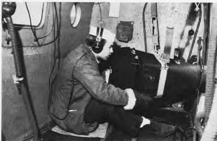
PHOTOGRAPHER L. E. LEONARD SWINGS K-18 CAMERA AT SNB DOOR TO SHOOT OBLIQUE PHOTOS
