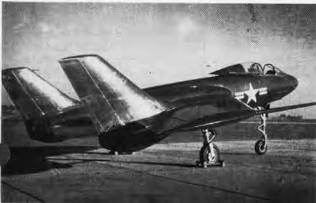
BIG TWIN RUDDERS IN WINGS OF THIS TAILLESS JET CARRIER FIGHTER
