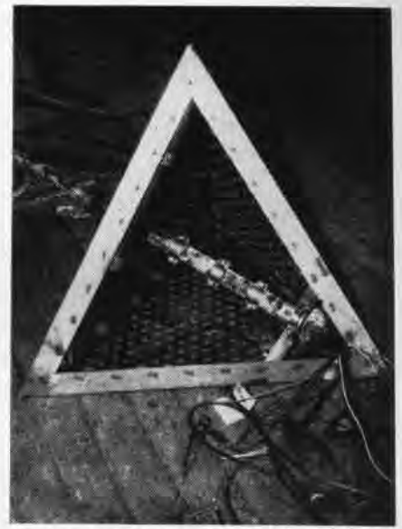
Underwater cage of hydrophone shows location of listening devices and cables
