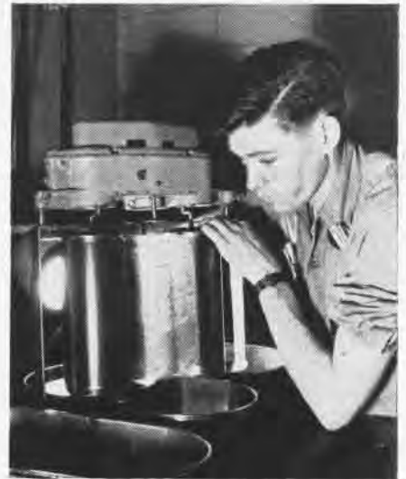
Rugged B5 roller tank handles 50 & 100 ft. rolls; L. J. Allen, AF3, develops.
