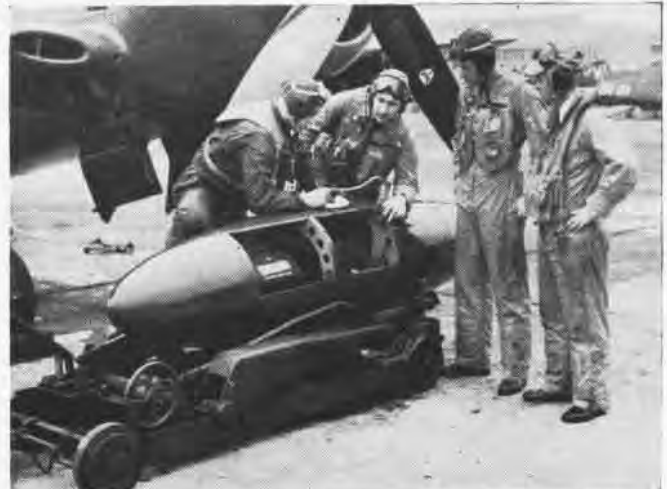
Capsule for trimetrogon camera is examined by Lt. (jg) J. A. March, Lt. (jg) R. C. Bridges, Lt. (jg) Ross, Lt. (jg) Elliot.
