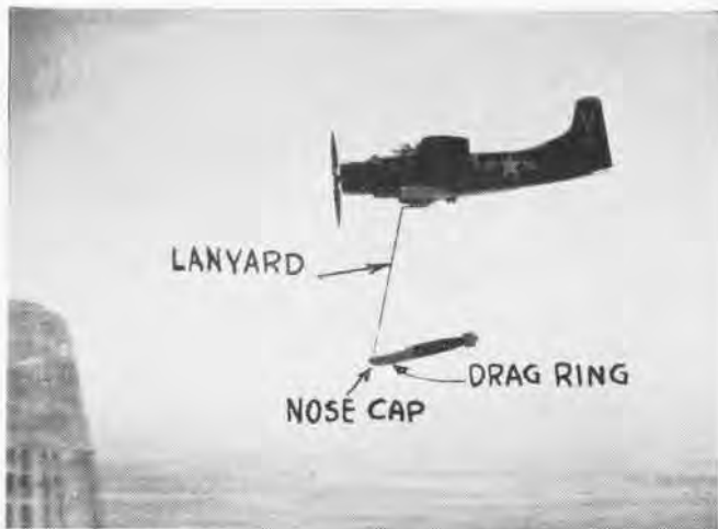
LANYARD PAYS OUT 26', THEN JERKS THE NOSE CAP FROM THE TORPEDO
