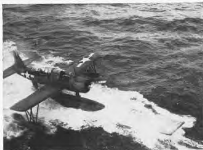
NET TRAILING SLED SHOWS WHERE HOOK ON OS2U FLOAT WILL ENGAGE
