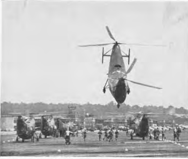
WEIRD FLIGHT ATTITUDE OF HELICOPTER AS IT STARTS TO GO AHEAD
