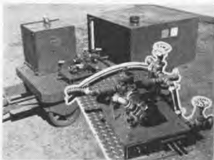
DISPENSER EQUIPMENT AND CLOSE-UP OF PUMP with a booster pump which is powered by a 24 volt battery cart. (The battery cart is the one in daily use on the line.)
