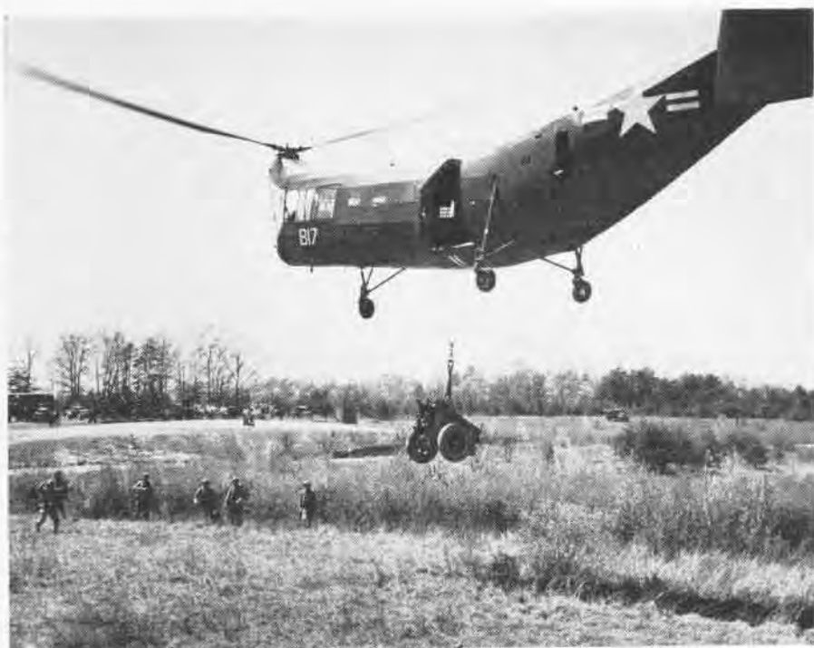
TRANSPORT HELICOPTER HOVERS WITH 75 MM. HOWITZER TO GIVE GROUND TROOPS FIREPOWER
