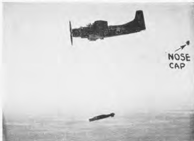
FREE OF NOSE CAP, TORPEDO WITH DRAG RING HEADS FOR ITS TARGET
