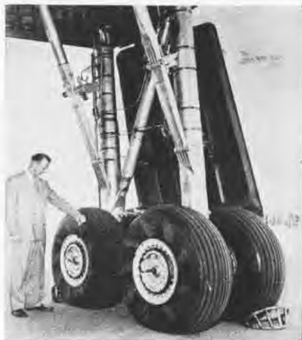
FLAPS, MOTORS PREROTATE TIRES ON THE R60
