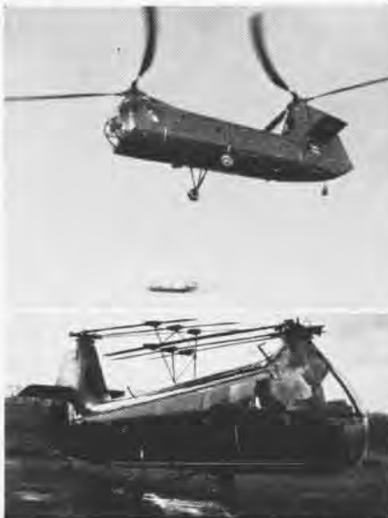
SEVEN-MAN PIASECKI FEATURES FOLDING ROTOR
