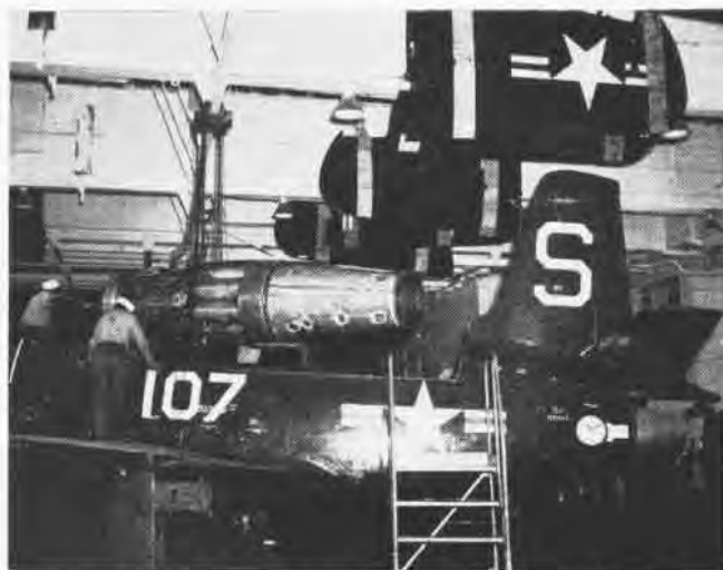
ENGINE CHANGE IN A JET SIMPLE OPERATION ON CVE HANGAR DECK
