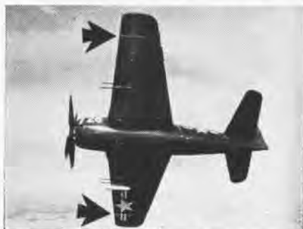
ARROWS MARK SHEAR LINE OF WING JETTISON
