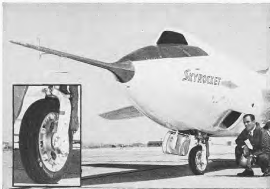
SKYROCKET'S SMALL NOSE WHEEL CARRIES TINY TIRE WITH HIGH PRESSURE FOR FAST LANDING
