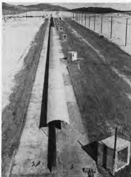
1500-FOOT RAIL TESTS HIGH SPEED ROCKETS
