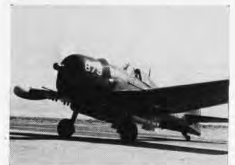
TWO TINY TIM ROCKETS RIDE ON F6F'S BELLY
