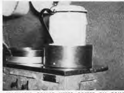
DETACHABLE COLLAR KEEPS COFFEE ON COILS
