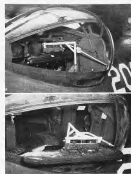
RACK SWINGS IN FOR REARMING, OUT FOR USE
