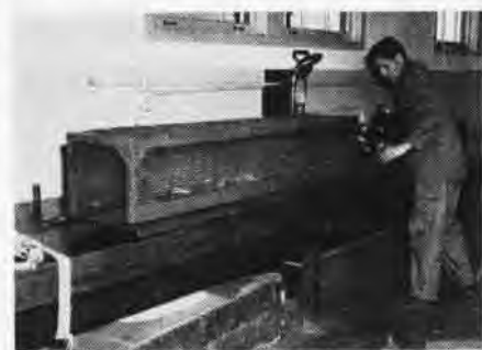
WIRE CAGE COVERS CHUTE BELT BEING TESTED
