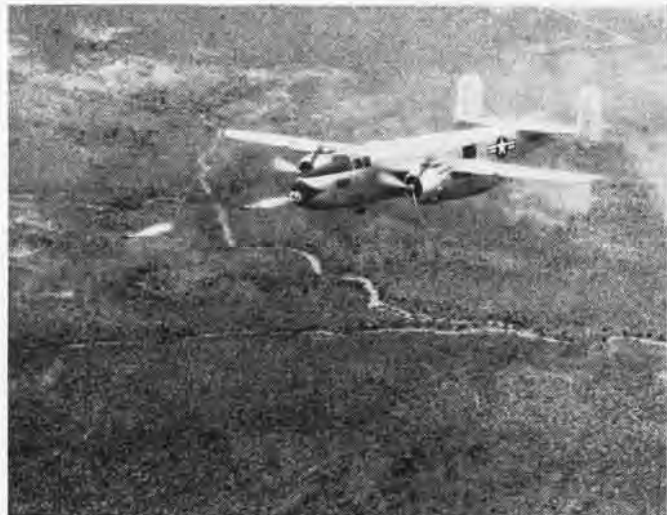
PBJ FIRES SPIN-STABILIZED 5" ROCKETS FROM TUBES IN PLANE NOSE
