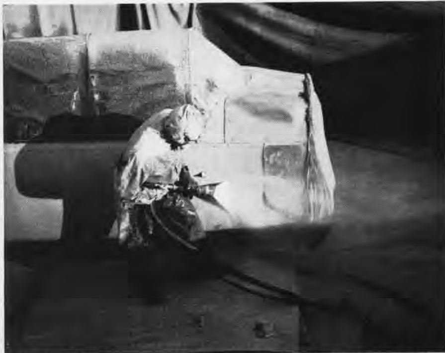
VAPOR BLAST PROCESS BEING USED ON SNJ AIRCRAFT AT ALAMEDA; NOTE PROTECTIVE MASKING
