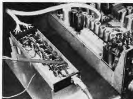
SIGNAL TRACER HELPS FIND DEFECTIVE PARTS
