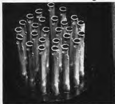
DEFECTIVE TERMINALS LACK RETAINING CLIPS
