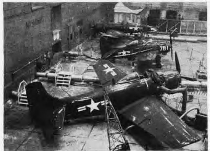
F4U, F8F, AD READY FOR TESTS; NOTE DUCTS TO CARRY OFF EXHAUST
