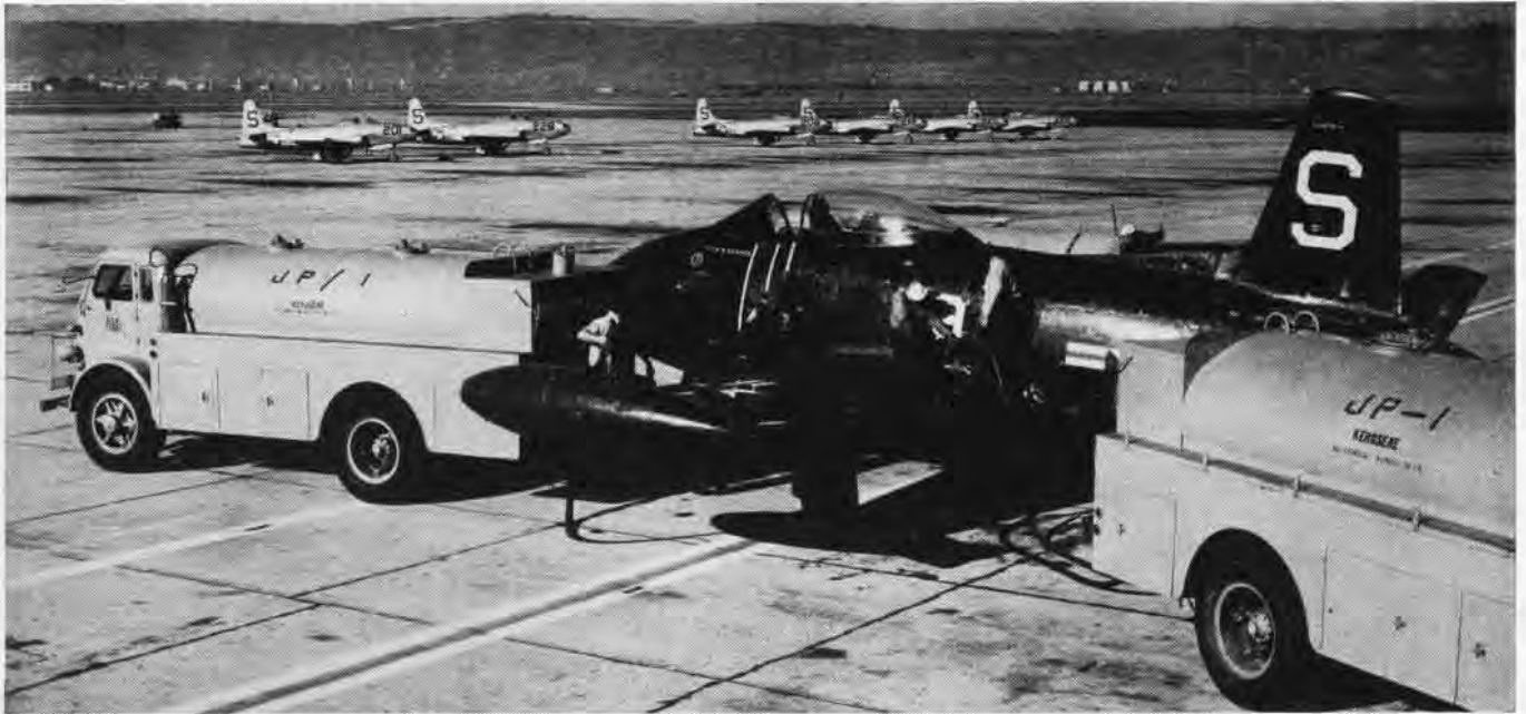
IT TAKES THREE GAS TRUCKS TO SIMULTANEOUSLY FILL ALL TANKS ON THE FJ-1 WHOSE ENGINES IN THIS CASE ARE BURNING JP-1 KEROSENE
