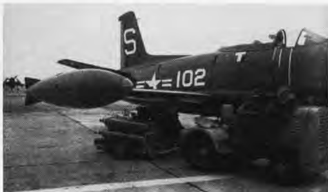
PORTABLE OXYGEN UNIT ON TRAILER NOW SERVICES BOTTLE IN FURY
