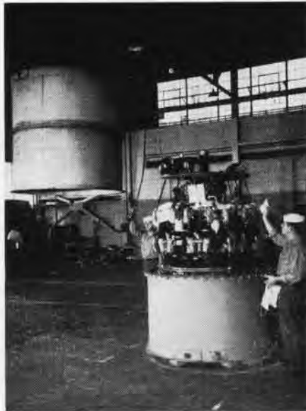
INSPECTION BEFORE ADDING ACCESSORY BOARD
