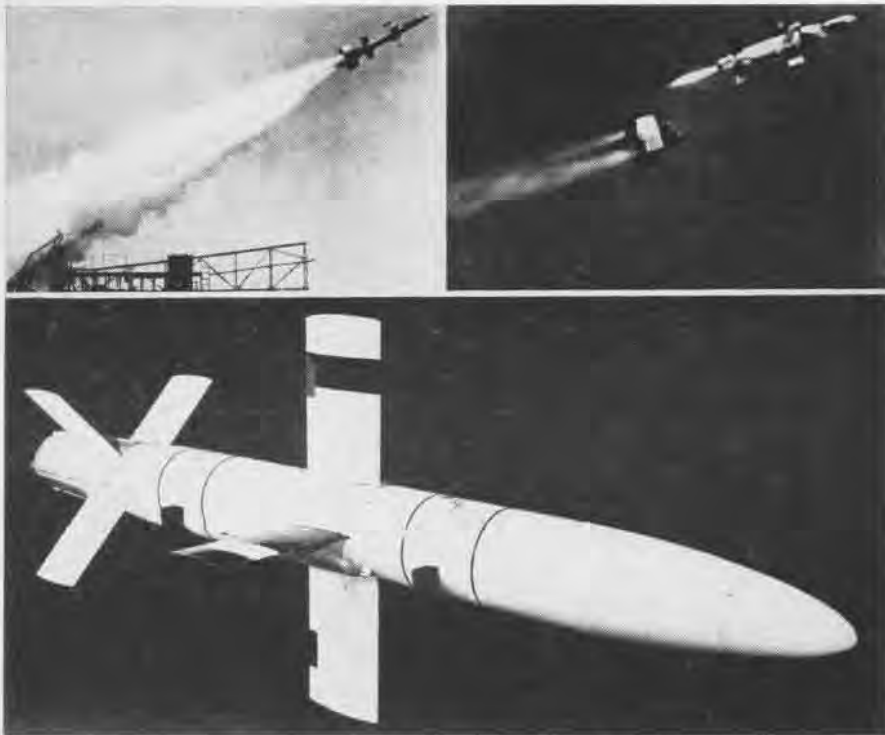
Aimed at such aerial adversaries as Kamikazes, the Navy's Lark guided missile shows itself in three phases in these newly-released photographs. Officially called the XSAM-N-4, the Lark is designed to intercept and destroy enemy aircraft before ship or shore targets can be attacked. It is liquid rocket fuel powered and has a twin-rocket booster assembly which separates in early flight, (upper right photo). The Consolidated Vultee missile has remote automatic control during flight.
