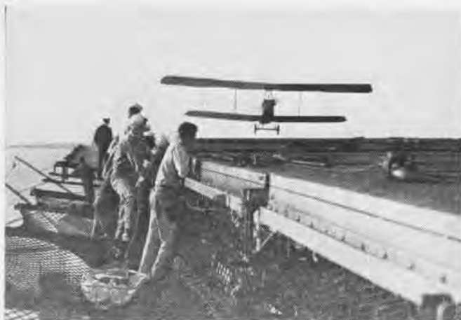
AEROMARINE WITH HOOKS ON UNDERCARRIAGE LANDS ON LANGLEY DECK
