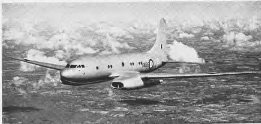
TUDOR 8, A DISTANT RELATIVE OF LANCASTER, IS WORLD'S FIRST 4 JET-ENGINEED TRANSPORT
