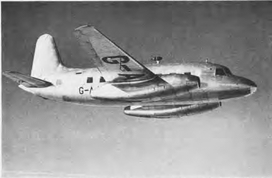
VICKERS VIKING WITH 2 ROLLS-ROYCE NENE ENGINES WORLD'S FIRST JET-POWERED TRANSPORT
