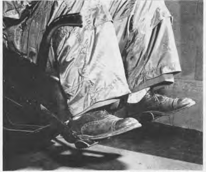
2 Next, the pilot puts both feet backward in stirrups so his toes will avoid cockpit edge as seat goes up
