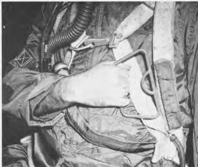
8 Now in free fall, pilot pulls on his parachute D-ring to unfurl his personal chute and float down
