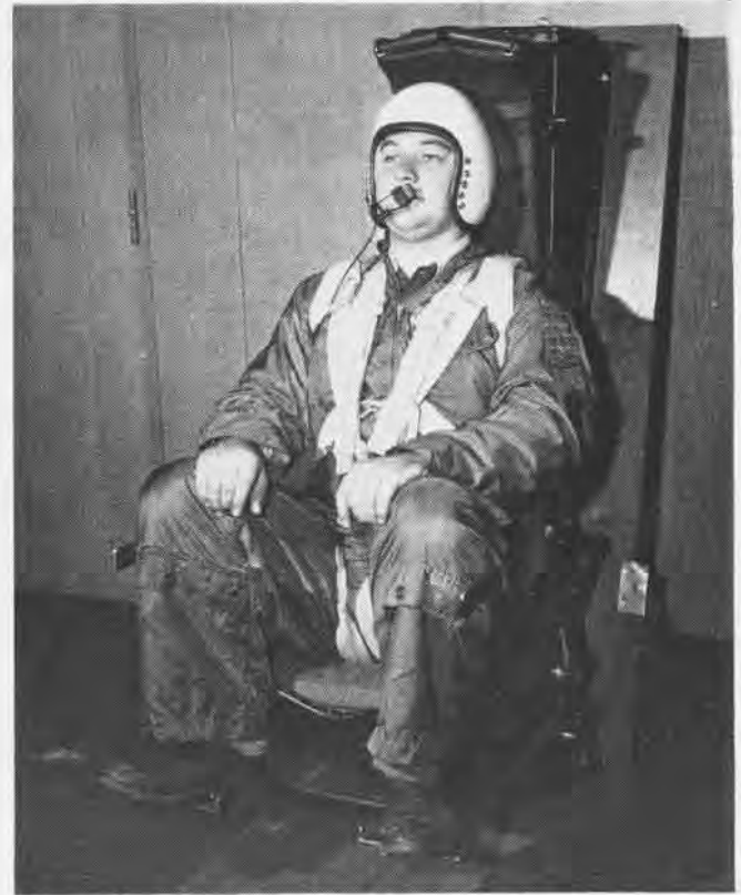
4 Head back, feet back in stirrups, the pilot is now in correct position to be ejected from his aircraft
