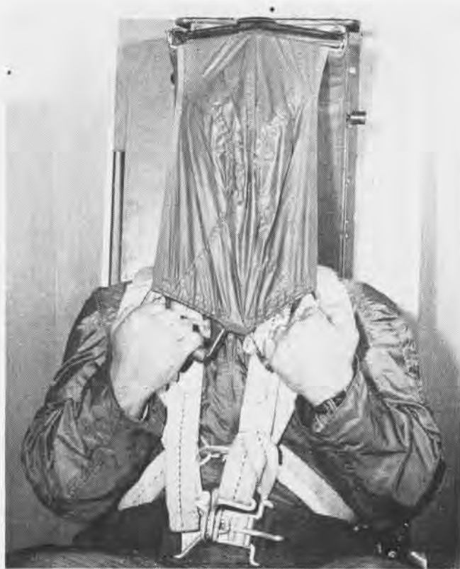
6 When face curtain reaches bottom of travel, cannon in seat fires; shaped curtain protects from blast
