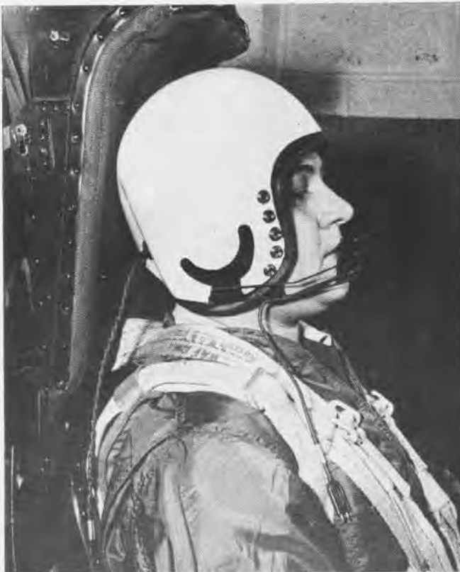
3 Pushing head firmly against the rest assures correct positioning of spine prior to firing catapult
