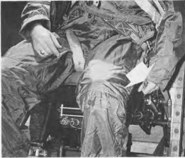
1 Pilot pulls pre-ejection lever to decompress cockpit and jettison the canopy so he can be catapulted
