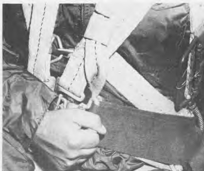
7 Once in midair, the pilot rides his seat for short time then jettisons it by pulling safety belt catch
