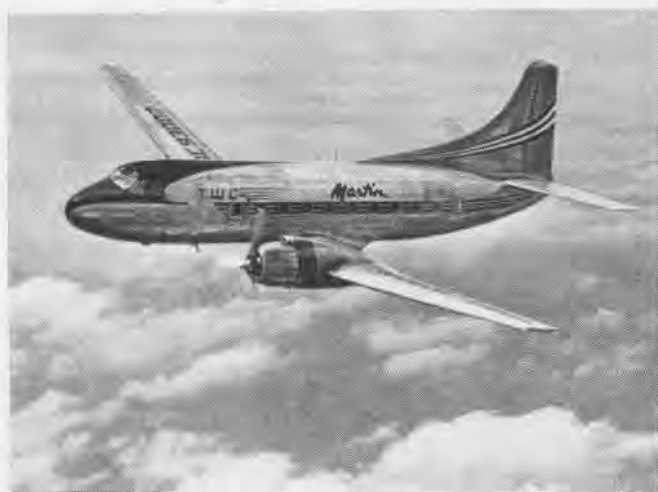
FAT FUSELAGE AND HIGH, FAIRED TAIL FEATURE FAST MARTIN 2-0-2
