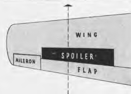
SPOILER RAISES UP TO DESTROY LIFT OF WING
