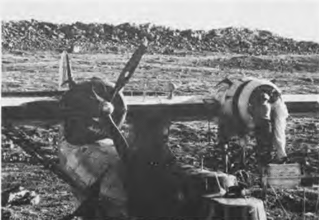
RCAF PHOTO PLANE LOST PROP IN ARCTIC, REPAIRED ON THE BEACH
