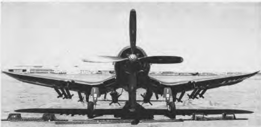
CORSAIR FIGHTER CARRIES TWO TINY TIMS, 5" ROCKETS, MANY ROUNDS OF 20 MM CARTRIDGES
