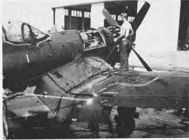
PLANES ARE WASHED BY SOLVENT MIXED WITH WATER UNDER PRESSURE
