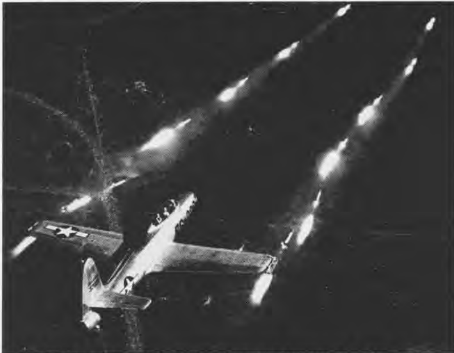
AN EVEN DOZEN 5" HVAR'S STREAK TOWARD TARGET: NOTE DISPERSAL OF ROUNDS ON THE WAY
