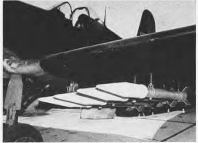
NEW NAVY 6.5" RAM HAS SHAPED CHARGE IN NOSE TO KILL OFF TANKS
