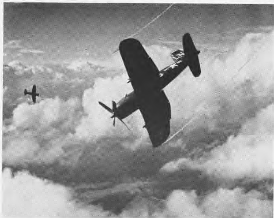
ROLLING PULLOUT FROM DIVE PUTS HEAVY STRAIN ON ONE WING OF FIGHTERS OR ATTACK PLANES
