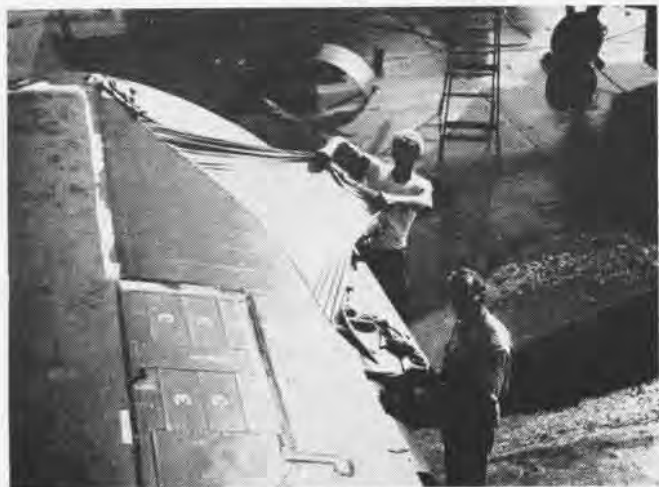
MEN REMOVE LIQUID ENVELOPE FROM PLANE WING AT LITCHFIELD PARK
