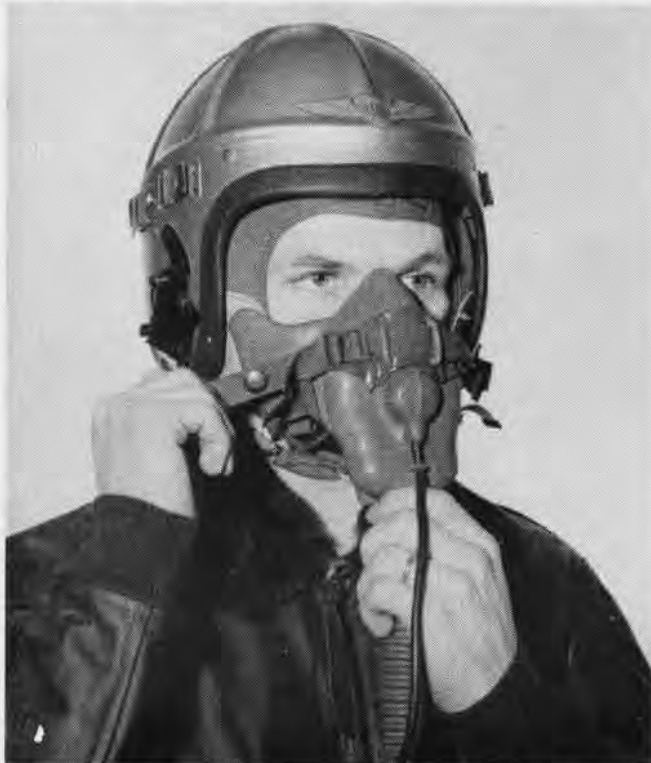
PILOTS PROTECTIVE helmet, inner helmet and A13A oxygen mask in place; mask has built-in lip mike so helmet boom is removed
