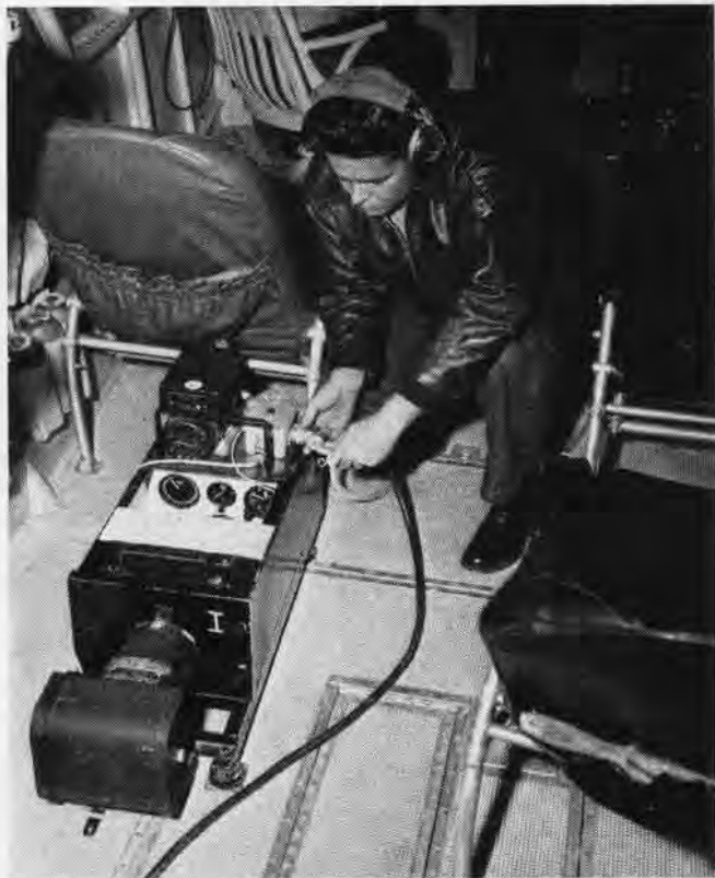
THIS IS THE FINISHED CAMERA UNIT INSTALLED IN AIRSHIP CABIN
