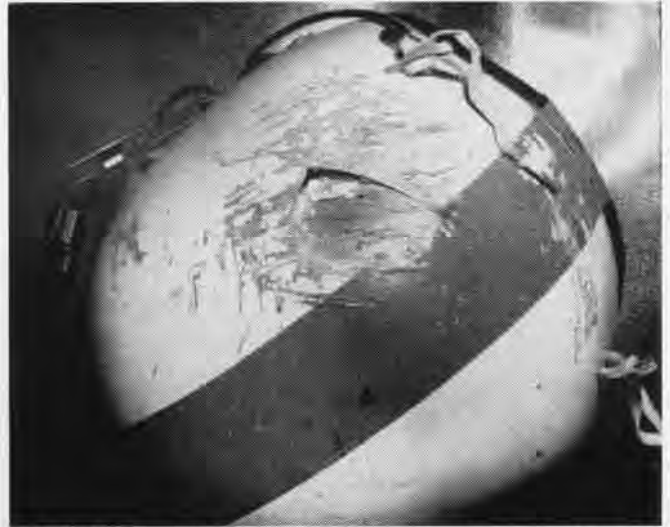
THIS HELMET saved the pilot's life in the plane opposite; gash in helmet might have been in his skull if he lacked the helmet
