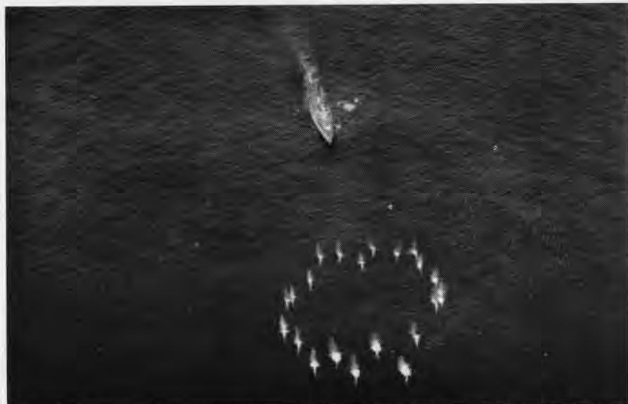
CAMERA ON BLIMP RECORDS HEDGEHOG PATTERN OF DEPTH CHARGES THROWN AHEAD BY DESTROYER
