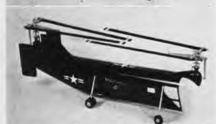
DRAWING OF BELL XHSL-1 ABOVE, MODEL BELOW Details Of Bell XHSL-1 Shown Tandem Rotors Mark ASW Helicopter
