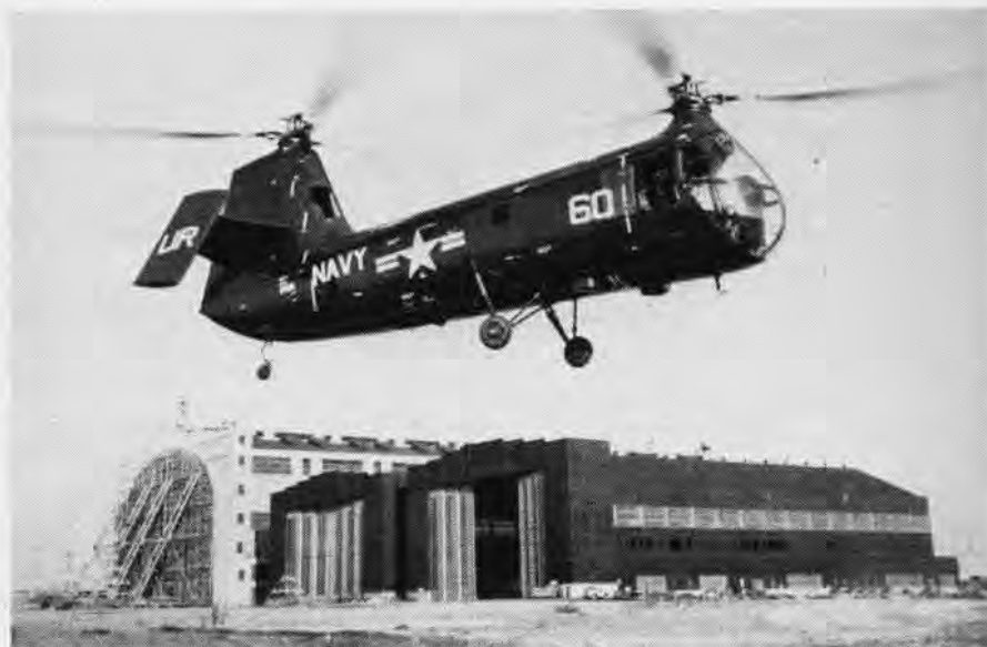
THE NAVY'S newest operational helicopter is the HUP-1, shown here making its first service flight with pilots of HU-2 at NAS Lakehurst. This shipboard helicopter has folding twin rotor blades. A number of them are being built for the Navy by Piasecki Helicopter Co.
