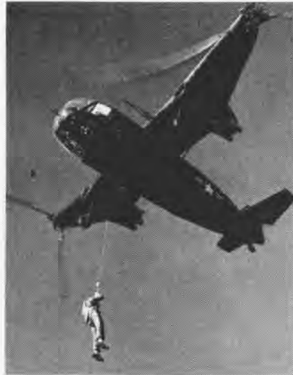
McDONNELL XHJD-1 , first twin rotored Navy helicopter, shows use of hydraulic hoist
