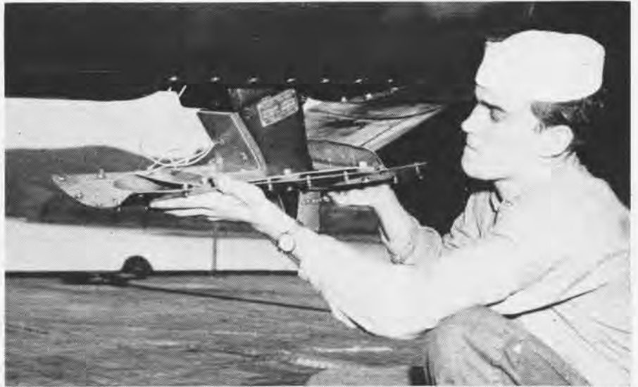
K-25 CAMERA AND MOUNT BEING INSTALLED IN CORSAIR BELLY BY L. C. MILLER ON BATAAN
