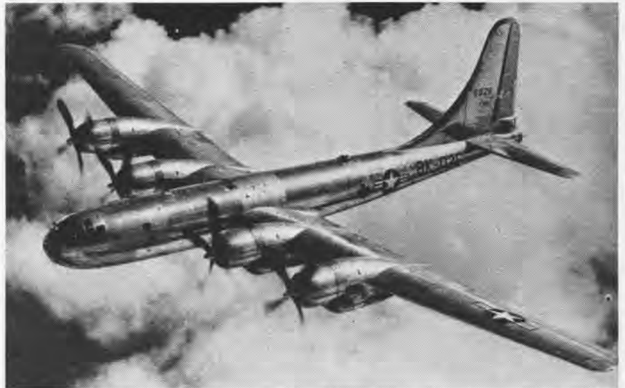
THE B-50 resembles the B-29 except that the vertical tail surfaces are taller than on earlier Superfortresses. This distinguishes it from B-29's Soviet copy, TU-4
