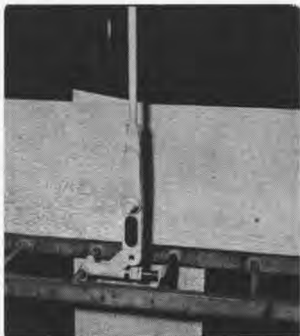
THIS JACK METHOD OF TESTING RUNS IS SAFE
