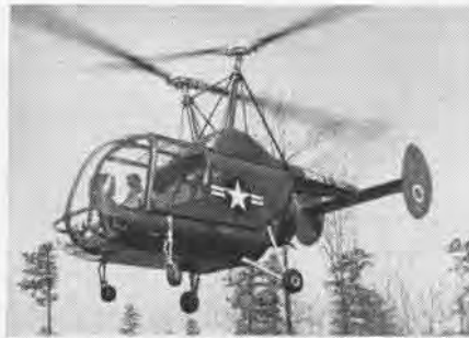
TRUE "eggbeater" is this HTK-1 Kaman built trainer, produced at Windsor Locks, Conn.
