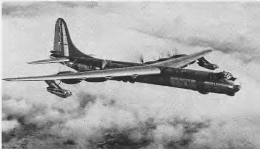
BIGGEST of the Air Force's strategic bombers, the B-36 has wings set high about midway between nose and tail. Six piston-driven propellers are supplemented on D version by two pairs of jet engines protruding forward of sweptback leading edge
