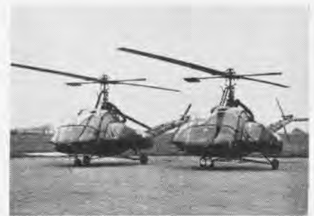
THIS HILLER helicopter features built-in litter carriers, ideal for Korean war zone
