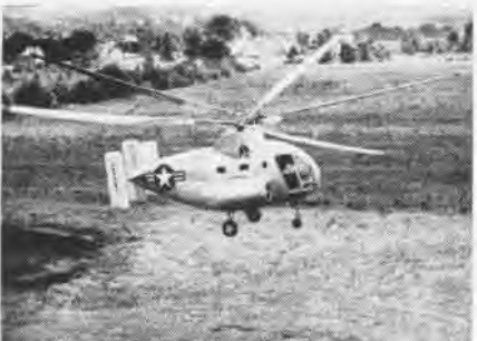
OF INTERMESHING rotor design is the Kellett XH-10; company pioneered in autogiro field
