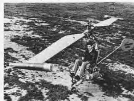
THE ROAR these pulse jets make on American Helicopter Co.'s XA-6 belie its tiny size
