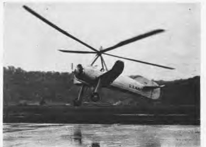
THE XOP-1 autogyro, although it resembles a helicopter, has no power applied to rotor, which rotates automatically and freely
