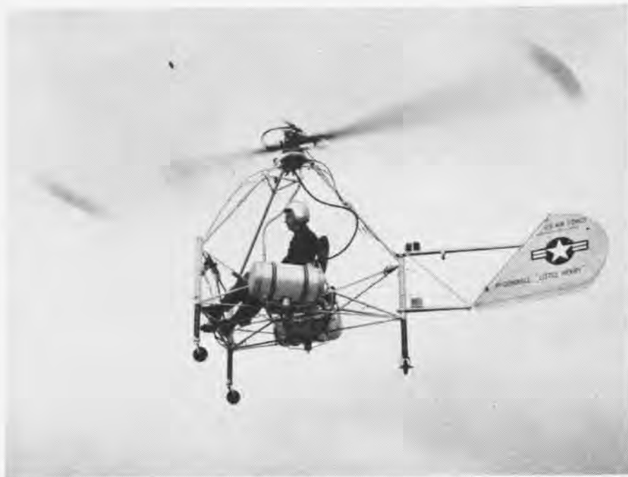
NOT MUCH more metal than an old fashioned bedstead makes up the diminutive McDonnell "Little Henry" which is powered by ram jet engines on the tips of each of the rotors
