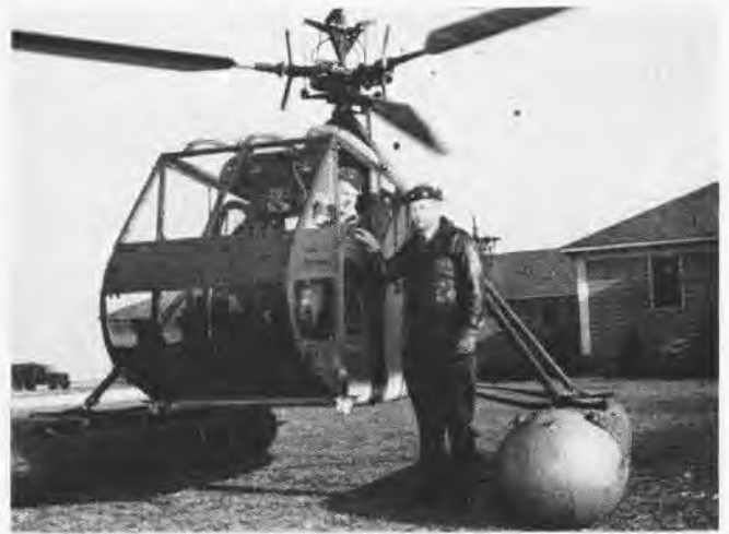
AMERICAN MILITARY pioneer in helicopters, Coast Guard Cdr. Erickson shown here standing beside an early HOS-1 with flotation gear
