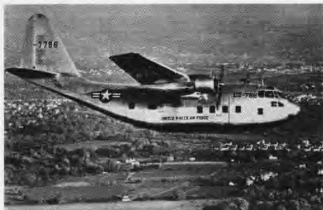
CHASE XC-123 IS AIR FORCE GLIDER WITH ENGINES, TAIL UPSWEEP
