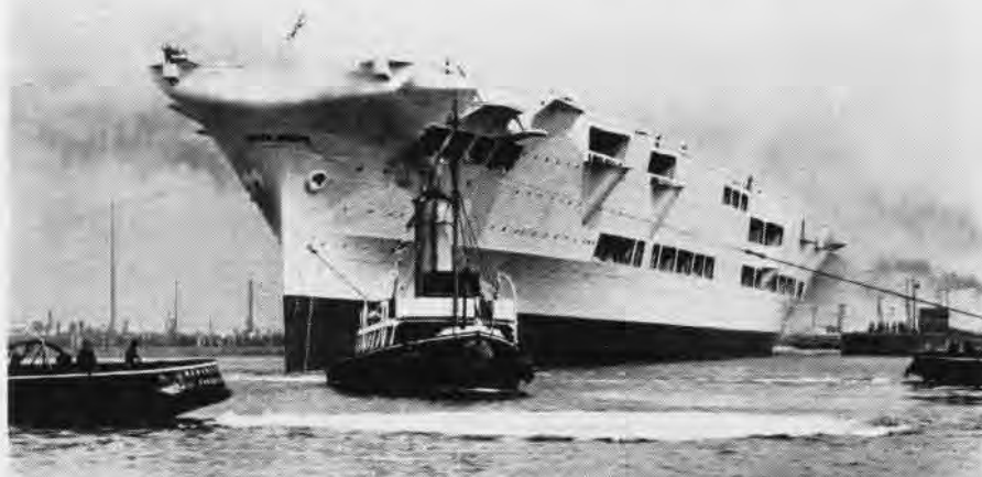
ARK ROYAL AFTER LAUNCHING AND BEFORE ISLAND WAS INSTALLED, DIFFERS WIDELY FROM OURS
