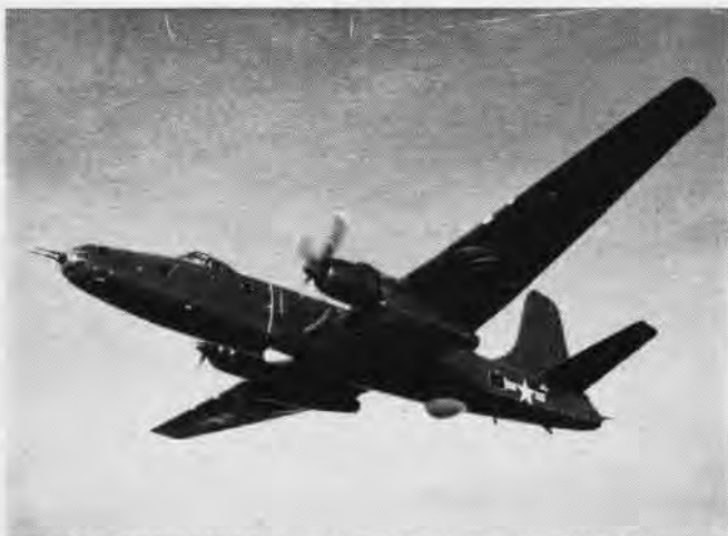
P4M HAS TRICYCLE LANDING GEAR, MUCH ELECTRONIC, RADIO EQUIPMENT
