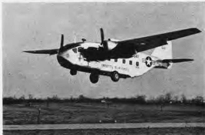
EARLIER MODEL CHASE C-122 WAS SMALLER GLIDER EQUIPPED TO FLY
