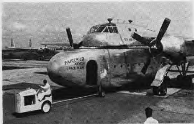
CARGO-CARRYING FUSELAGE DETACHES FROM AIR FORCE'S PACK PLANE
