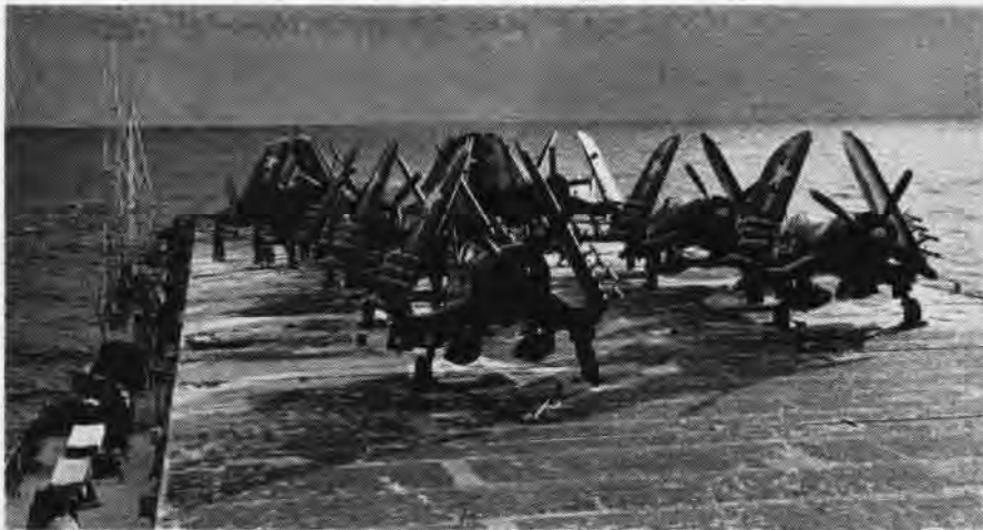
SNOW-SWEPT AND icy are the decks of the CVE Badoeng Strait, operating off Northern Korea shores. Poised on the deck are a Marine fighter squadron's Corsairs, loaded with eight HVAR rockets each and carrying two belly tanks of gas which give the F4U plenty long range.
