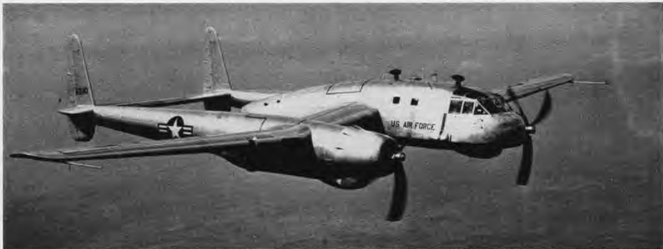
WITHOUT ITS CARGO POD, FAIRCHILD'S NEW PACK PLANE, THE C-121 IS A STRANGE LOOKING CREATURE AS IT FLIES BACK TO GET NEW LOAD
