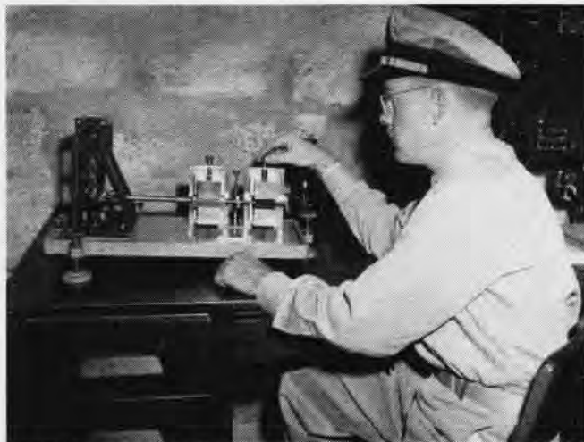
DAMPING MECHANISM ON SEISMOMETER IS ADJUSTED BY LT. (JG) ROUSH
