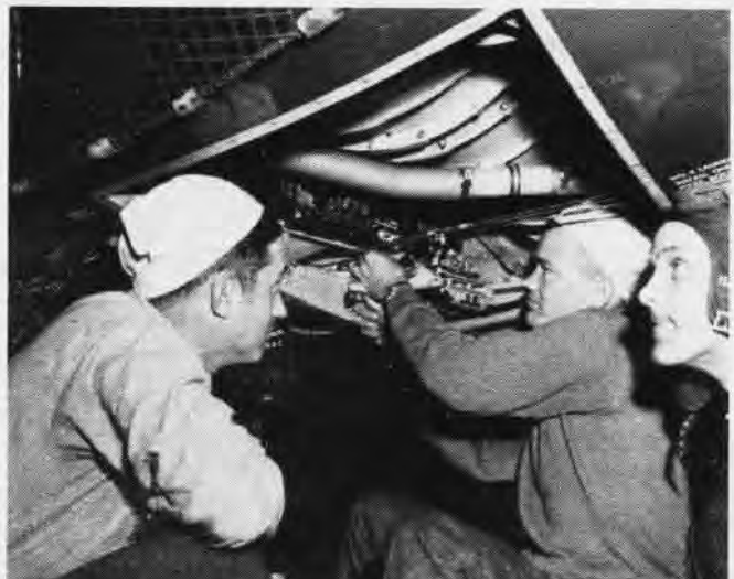
MAINTENANCE MEN of VC-4 work on starter circuit of F2H-2N; R. J. Lang, AE3, W. J. Bowen, AEC and C. B. Noel, AD1, plane captain.
