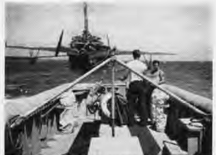
PIPE IN BOAT'S CENTER MAKES TOWING EASIER
