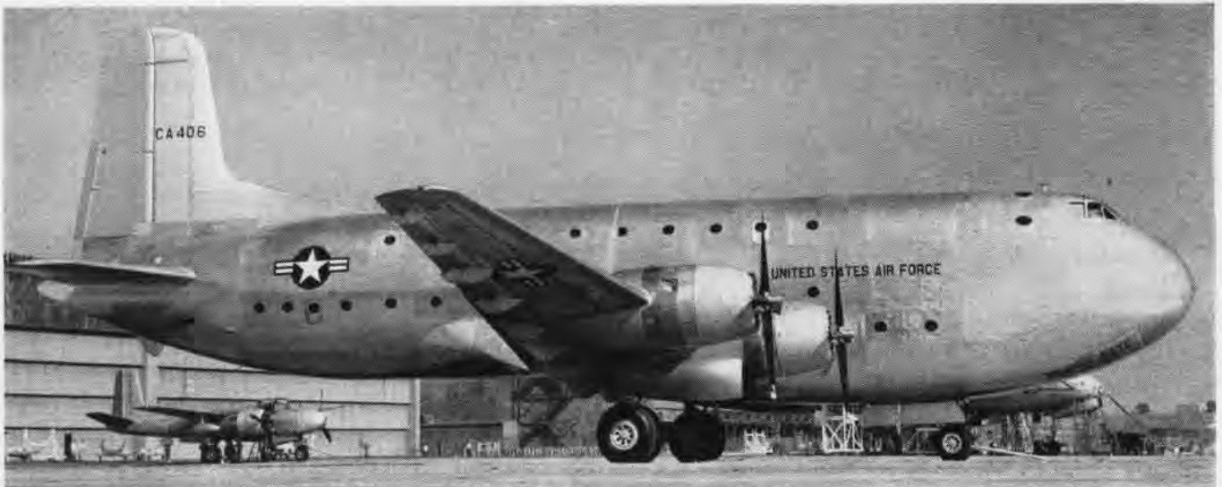
GIANT DOUGLAS GLOBEMASTER II HAS CLAM-SHELL DOORS IN NOSE FOR UNLOADING ITS CARGO; THIS C-124A CAN CARRY 222 COMBAT TROOPS
