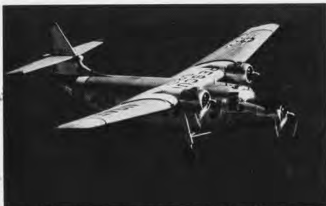
TRI-MOTORED NORTHROP RAIDER HAS FIXED LANDING GEAR, HIGH WING
