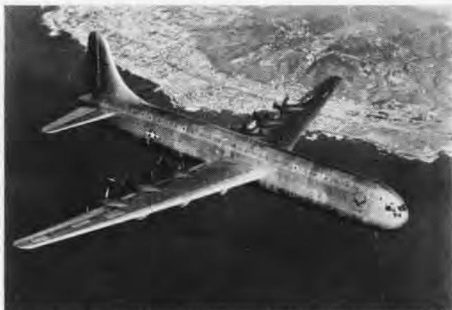
SIX PUSHER PROPELLERS, CIGAR-LIKE FUSELAGE ON CONVAIR'S C-99
