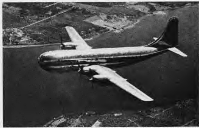
BOEING STRATOFREIGHTER HAS FAT FUSELAGE TAPERED TO HIGH TAIL
