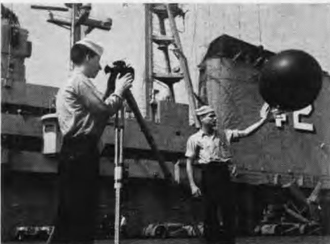
AEROGRAPHER'S MATES are highly trained; here V. L. Zirpoli, AG3, and M. B. Chandler, AG1, prepare to make sounding of upper air.
