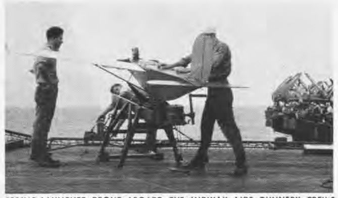
SPRING-LAUNCHED DRONE ABOARD CVB MIDWAY AIDS GUNNERY CREWS
