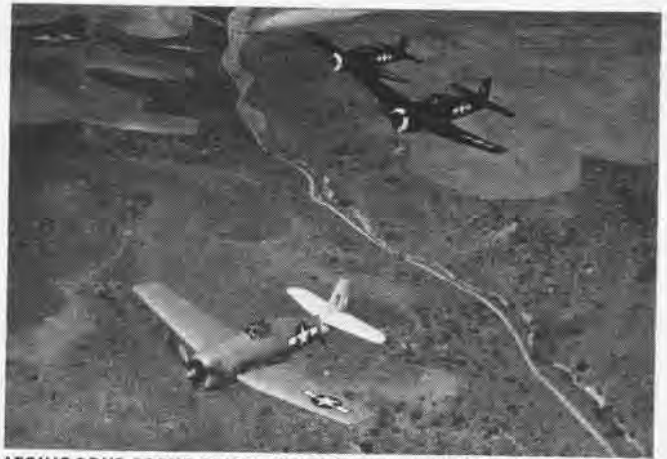
ATOMIC BOMB DRONE GUIDED BY 'QUEEN' PLANE WITH A SPARE ON HAND
