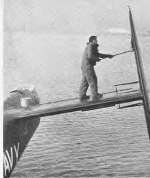
NAVY PBM Mariner operating in Japan gets coat of defrosting fluid on tail surfaces
