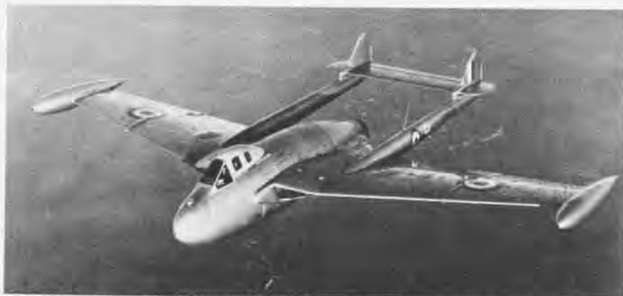
DE HAVILLAND VENOM TWO-SEATER NIGHT FIGHTER HAS GHOST ENGINE; CARRIER VERSION IN MILL
