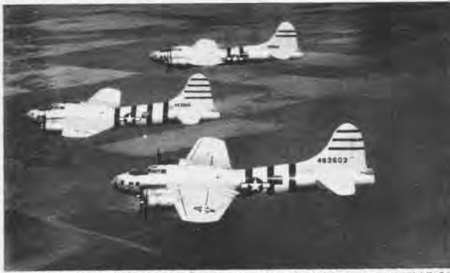
AIR FORCE USES REMOTE CONTROL TO FLY FORTRESSES IN FORMATION
