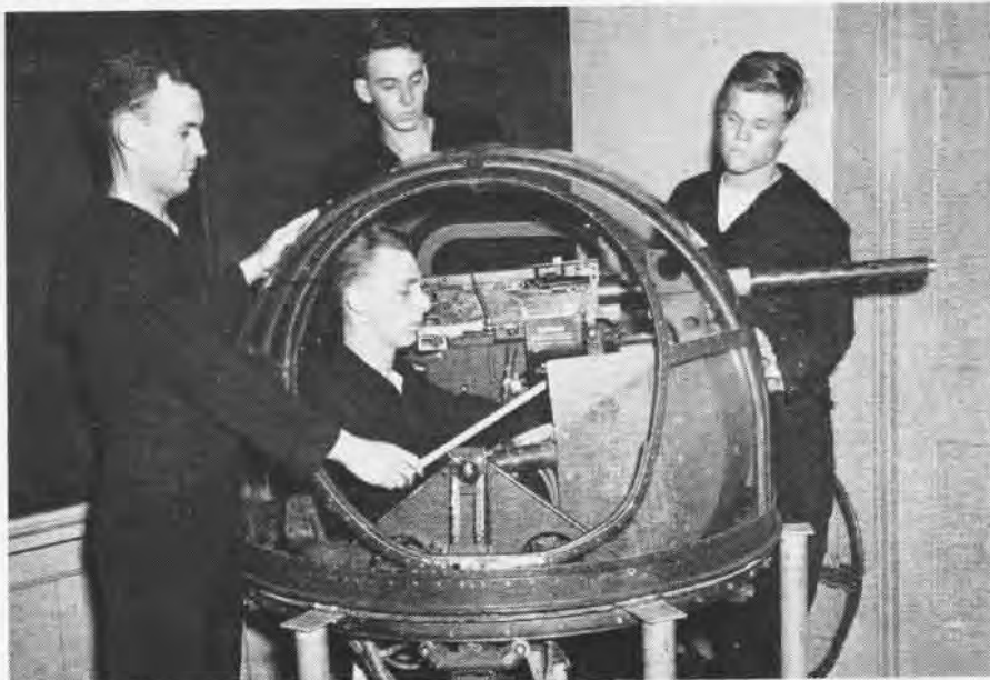
TO MAKE TRAINING COME ALIVE —NAS ATLANTA utilizes many training devices; here ordnanceman Freeman explains Gramman aircraft turret to Cartledge, Davis and Cobb
