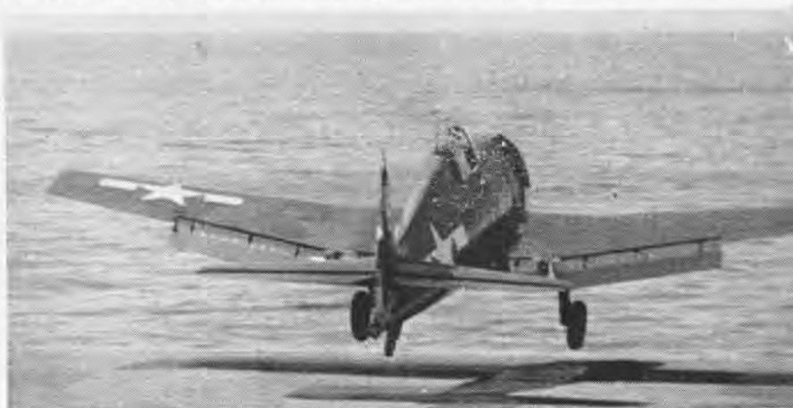
RED HELLCAT DRONE, PILOTLESS AND FLAPS DOWN, TAKES OFF SHANGRI LA AT BIKINI TESTS
