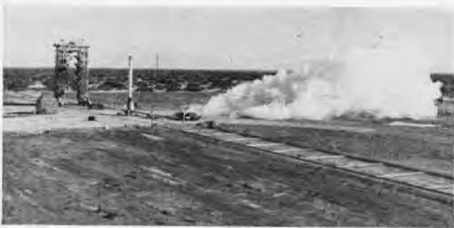
8 STATIC FIRING of engine is done with rocket bolted to platform; flame goes into a water pit, hence the steam
