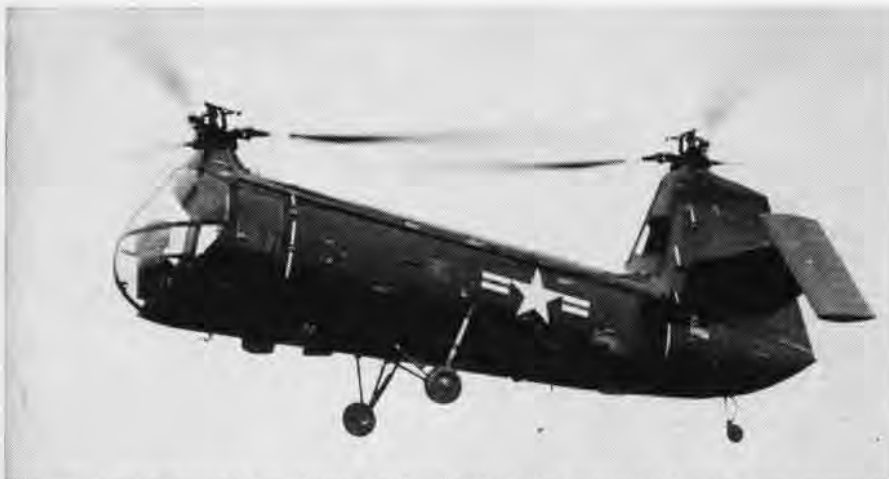
FIRST PRODUCTION models of this carrier-based HUP-1 helicopter by Piasecki are now rolling off the lines at Morton, Pa., to fill a sizeable order by the Navy. This tandem-rotor helicopter with folding blades was designed especially to operate from carriers and can go down the elevator of a CVE-55 class carrier without folding the rotors, if necessary. The helicopter has been clocked at 131 mph, carries five passengers and a crew of two men. Other features are an internal rescue hatch adjacent to the pilot's seat, rotors seven feet above deck for safety reasons. An HUP-1 recently flew with a new Sperry autopilot.
