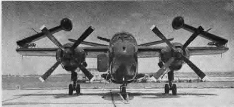
TAKE A LOOK AT that folding rudder, those folding wings, the twin engines and try to guess what this aircraft is. It is the Navy's newest carrier-based attack bomber, the North American AJ-1, which made its first carrier landings in September. The plane made takeoffs from a carrier as early as April. One of the first passengers when the plane did its arrested landings was John F. Floberg, Assistant Secretary of the Navy for Air. Powering this 50,000 pound giant are two R-2800 engines and one jet engine located in the after fuselage. It is the fourth multi-engine type aircraft to land aboard a carrier.
