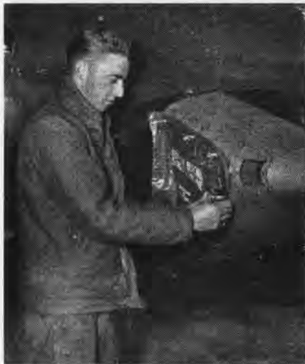
To protect jet engine Counts, AA, of VF-781, places cover over intake of squadron Panther
