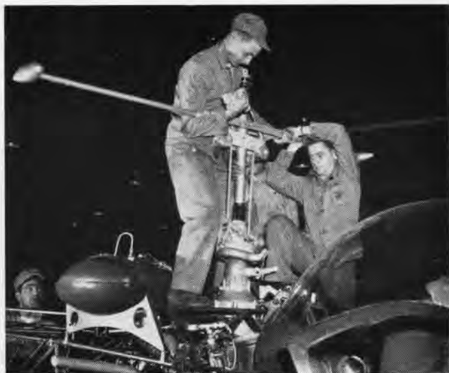
MECHANICS AT Quantico disassemble stabilizer bars on helicopter prior to loading it aboard the transport plane for Orient
