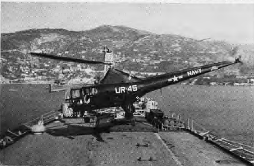
WHERE ONCE powder charges blew OS2U's off the stern end of cruisers is only a flat deck today—a homing ground for helicopters which have replaced the float planes. In this picture Lt. F. D. Richards takes off from the USS Columbus at Villefranch, France, harbor.
