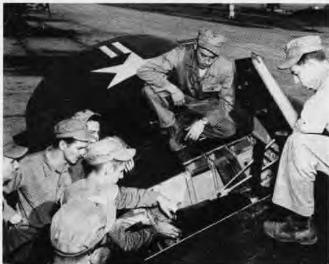
ON-THE-LINE CLASS —VMF-143's Schmidt and Schultz (on wings) watch T/Sgt. Johnson demonstrate how to remove FG wing guns
