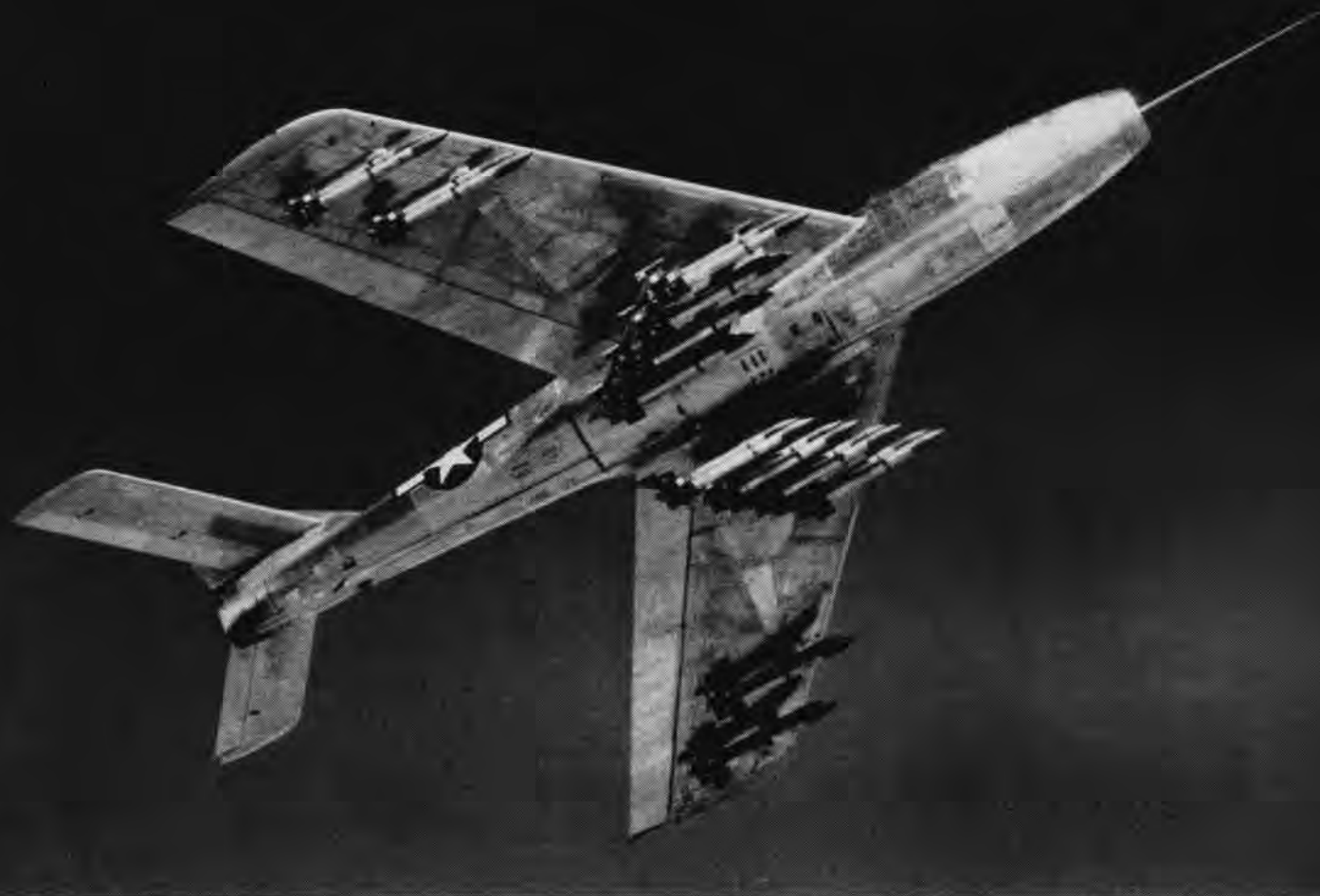
LOADED with 24 HVAR rockets, this swept-wing version of the USAF Thunderjet, the F-84F, claims high speeds and long range;
