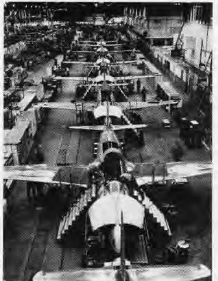
TWO SEATER jet trainers, TO-2's, roll off the assembly line at Lockheed Aircraft's huge plant at Burbank, Calif. This is training version of Air Force F-80 Shooting Star
