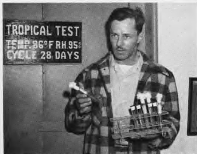
ENGINEER R. H. Powell shows specimens of fungi which are kept under refrigeration until introduced into equipment for tropical tests
