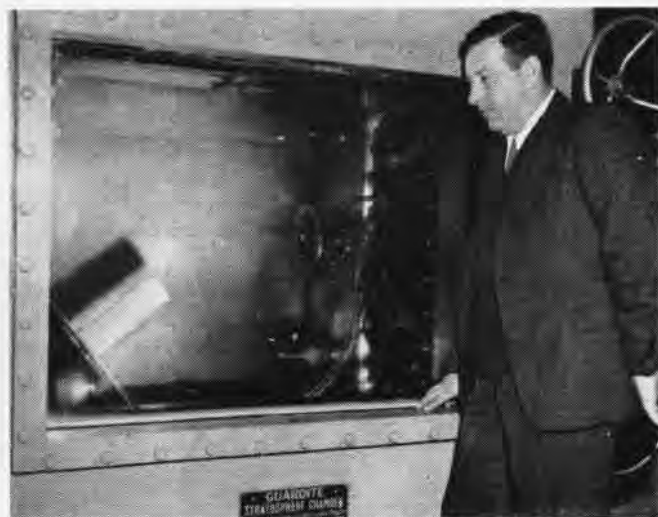
SIMULATED AIR blasts at 50,000 feet are directed at generators and other equipment under the eye of John Fulton, laboratory mechanic
