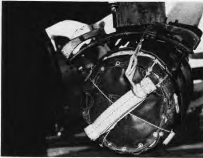
CIRCULAR CAN holds Leyte survival gear on plane; photo shows parachute and static line stowage in MK51 bomb rack of Corsair aircraft
