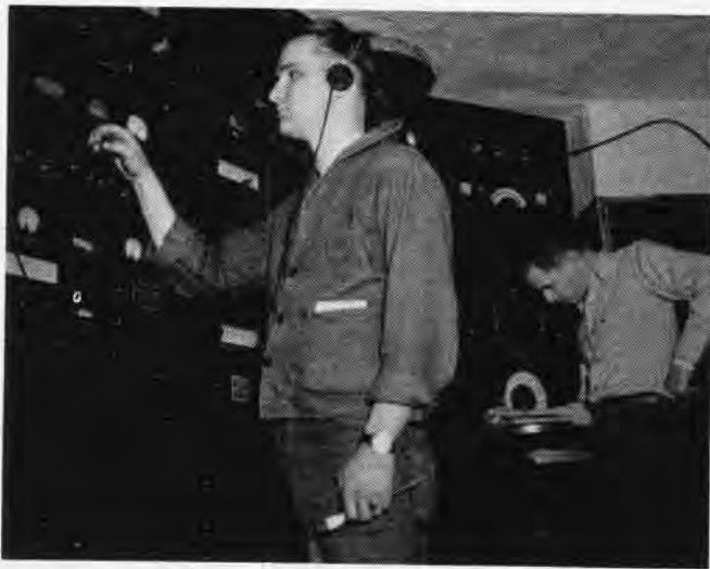
IN COPPER shielded room which almost stops outside interference, W. Marable, AT3, B. D. Walker, lab technician, chart performance
