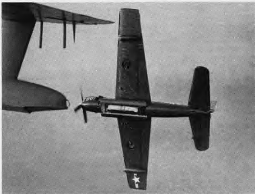
BOMB BAYS are going back on the Navy's planes again, as this aerial shot of the AF-2S indicates. During the war, the TBF's and SB2C had bomb bays, but postwar designers of attack planes like the AD-1 and AM-1 did away with bomb bays and carried torpedoes and bombs externally. Now comes the new AF Guardian with bays again. This photo shows the big antisubmarine attack plane carrying a dummy torpedo. Note searchlight and radome.
