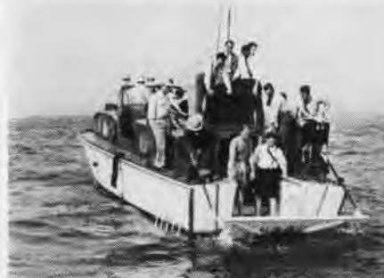
THE NAVY has procured for the Air Force a new crash rescue boat, a 40-foot craft with a stern gate that can be lowered to facilitate pulling pilots out of the water. The gate is 18" under water so a litter can be placed under the survivor. Guards protect him from injury by the boat's spinning propellers.
