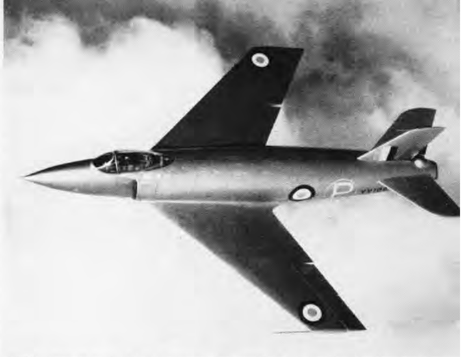
BRITISH Supermarine 510 Swift , a swept-wing version of the earlier Attacker , was the first swept-wing plane to land or take off from carrier; note small horizontal stabilizer
