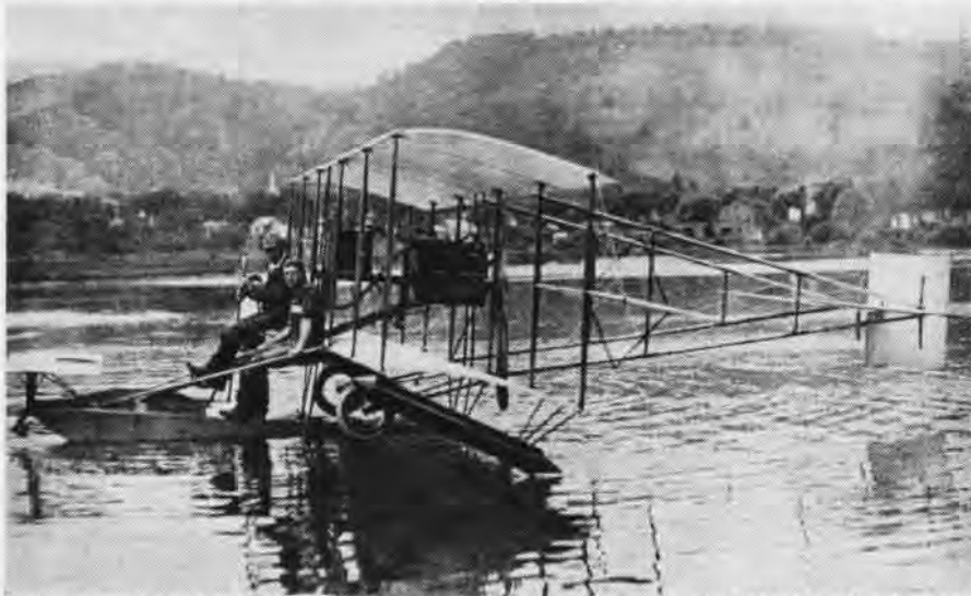
THIS IS THE NAVY'S FIRST AIRPLANE, THE CURTISS TRIAD WITH RETRACTABLE LANDING GEAR
