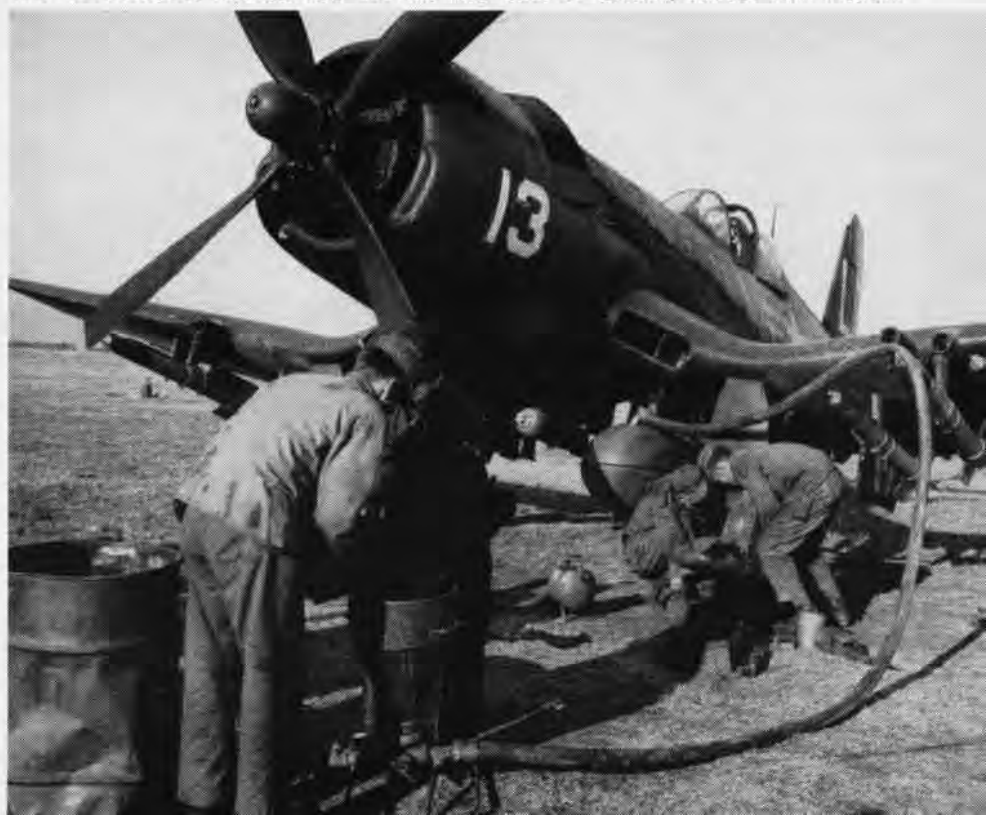
SPEED IS ESSENCE AS MARINES PUMP NAPALM INTO TANK OF CORSAIR, LOADED WITH ROCKETS
