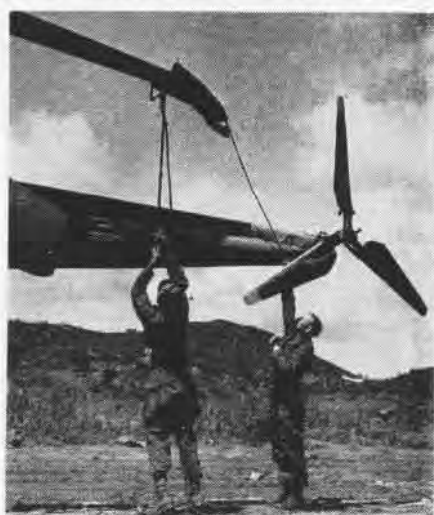
AFTER THE day's work, Saliba and Gerald T. Campbell put restraining boot on the rotor
