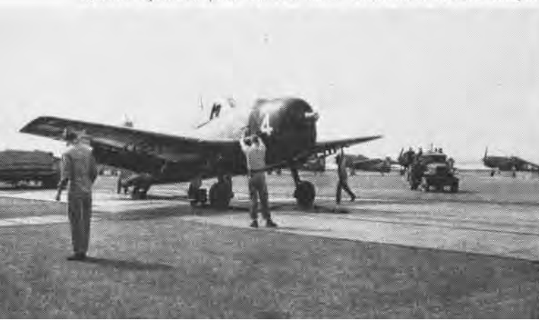
HOOKING UP for catapult shot—To get pre-carrier practice Air Reserve squadron from NAS Willow Grove uses NAMC catapult
