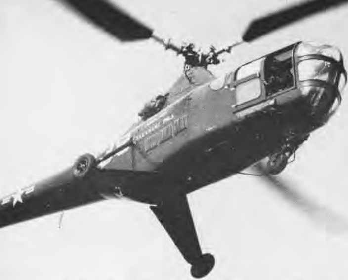
"LOOK NO HANDS"—Pilot Kenison takes life easy as autopilot developed by Aero Instruments Lab controls hovering helicopter
