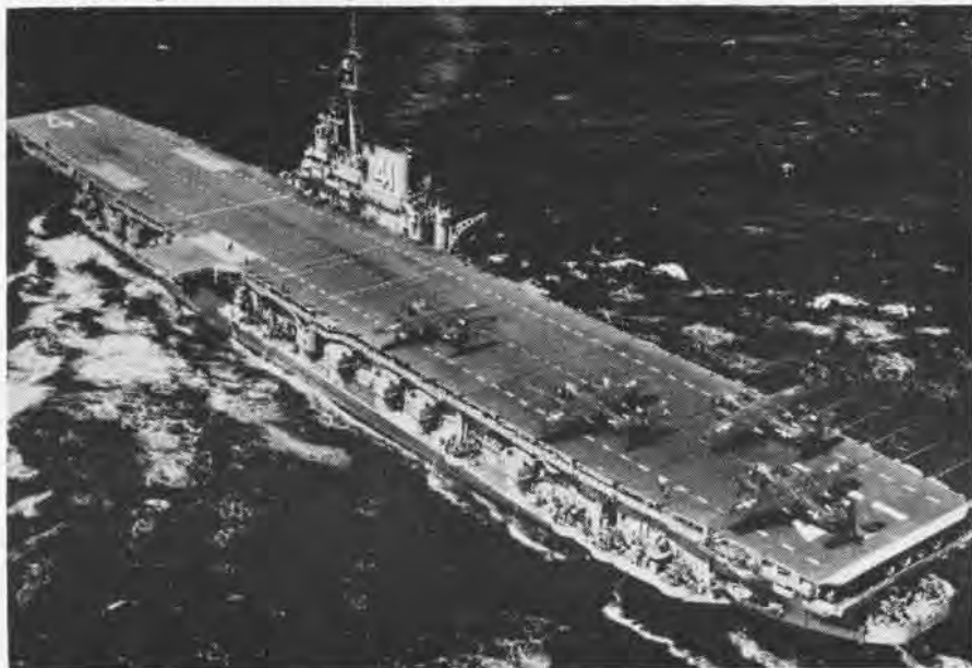
ONE OF the first photos showing more than one AJ-1 on a carrier is this shot sent in by the CVB Midway. Here four of the giant 50,000-pound twin-engined planes, largest built for carrier duty in the world, are posed on the Midway's long flight deck during a break in qualification flights. The AJ-1 is powered by two P&W Double Wasps and a J-33 jet engine.
