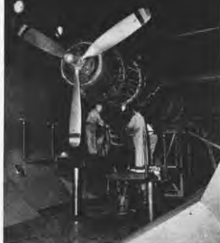
MOUNTING P&W R-2800 engine in test cell for endurance testing at Aero Engine Lab
