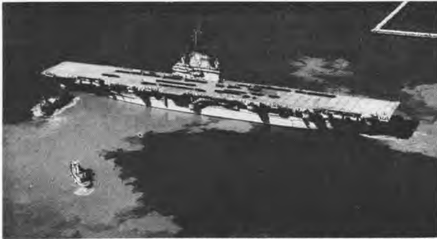
TRIM SUPERSTRUCTURE, LACK OF DECK TURRETS FEATURES 'NEW LOOK' OF FAMOUS OLD ESSEX
