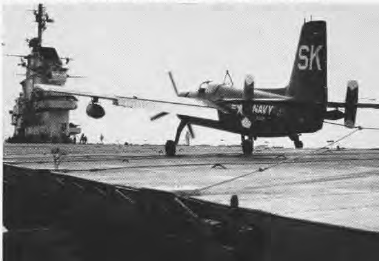
NAF SHIPS' installations developments at work with the Fleet—Here an AF hooks an arresting wire to land aboard the USS Essex
