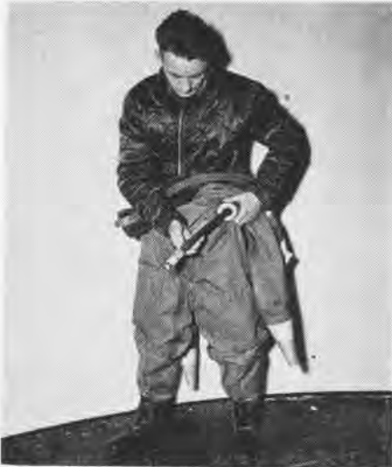
INSERTING G SUIT TUBE; NOTE INNER LINER
