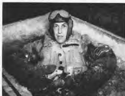
IN -30° ROOM TEMPERATURE, SUIT IS TESTED
