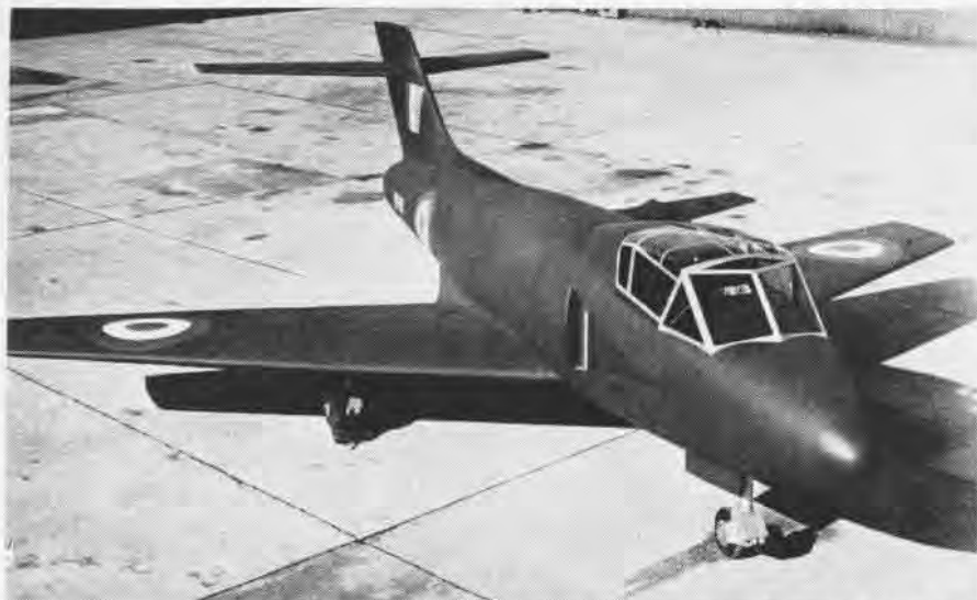
BRITISH BOULTON PAUL JET TRAINER WITH SIDE-BY-SIDE SEATS, POWERED BY ROLLS ROYCE JET
