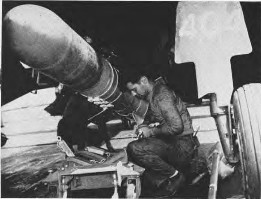
RICHARD R. AIELLO, AOS, ARMS A TINY TIM ROCKET ON CORSAIR DURING MIDWAY'S REFRESHER
