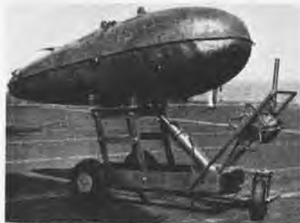
SALVAGED PARTS MAKE UP NAPALM BOMB HOIST
