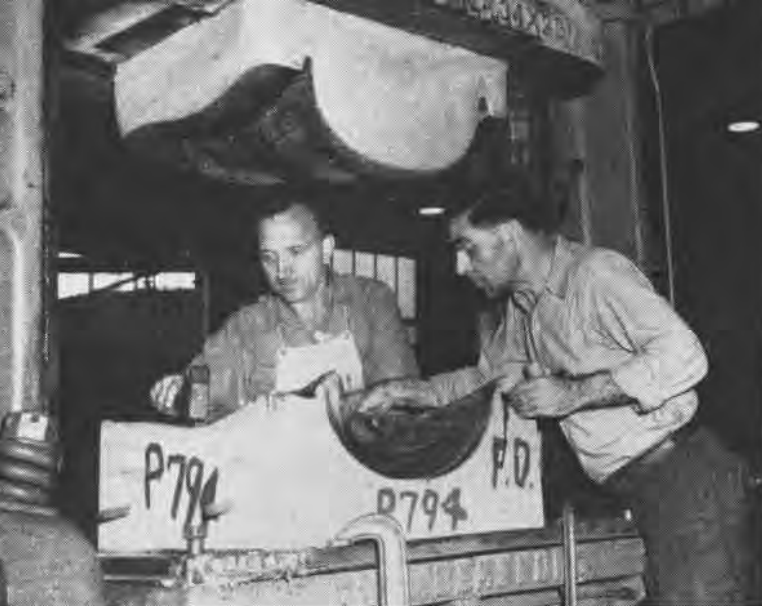
SHEET METAL SHOP —Aviation metalsmiths Bebringer and Wollson work on the back of an R5D seat being formed by drop hammer
