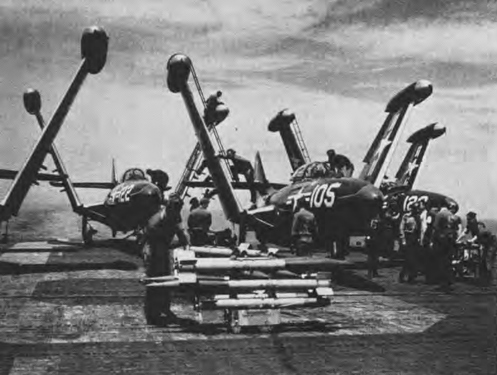
MAINTENANCE crews aboard the Bon Homme Richard refuel Panther jets for another strike as ordnancemen stand by with HVAR's and Ram 5" rockets, the latter for piercing Red tanks
