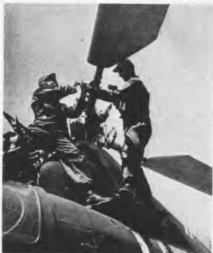
DONNIE Couser, AD3, and John N. Price, airman, tighten helicopter rotor blade bolts
