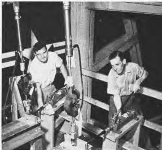
ASL'S DONAGHY and Waugh apply load to airplane wing with hydraulic tension jacks
