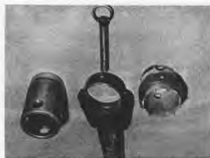
LONG-HANDLED WRENCH LOOSENS PROP NUTS
