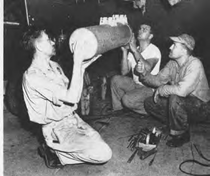
FACTORY ASSEMBLY and Test Shop —Aircraft mechanics Hibbs, Everist and Juriga put JATO installation in F9F Panther wing
