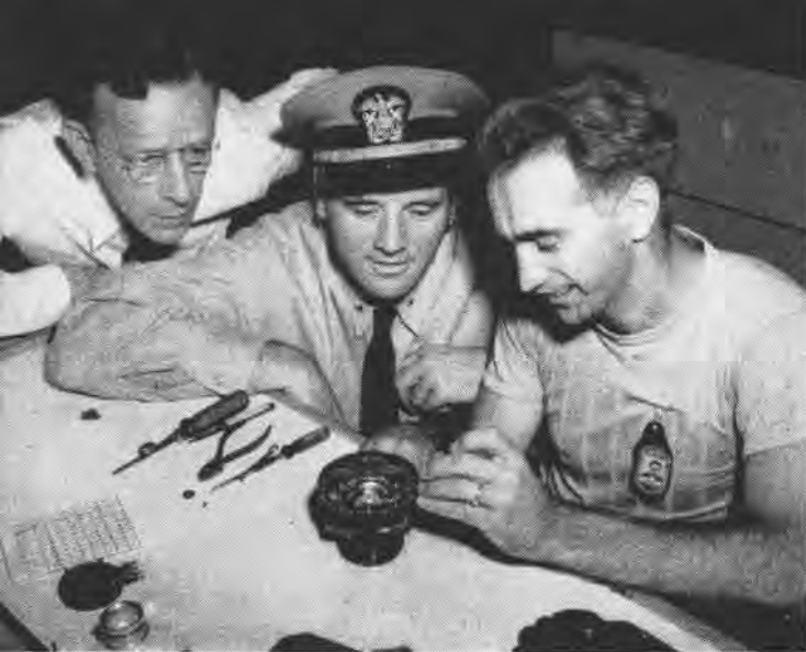
INSTRUMENT SHOP —NAF production officer Laurich and G. Shaefer watch H. Halley check gimbals ring assembly for proper balance
