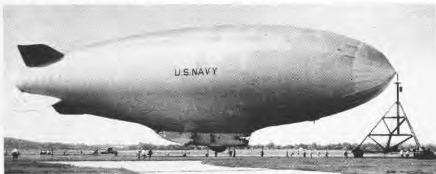
SIDE VIEW OF NEW NAN AIRSHIP SHOWS TAIL SURFACES AT 45° ANGLE INSTEAD OF OLD STYLE
