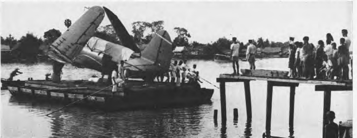
THAI NATIVES POLE SB2C ON BARGE UPSTREAM TO LAND AIR BASES; AT 6 WINGS HAD TO BE REMOVED TO PASS UNDER BRIDGES ON RIVERS
