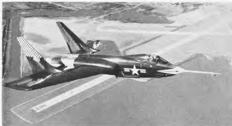
WHEN THE NAVY'S newest jet fighter, the F7U-3 Cutlass, comes off the production line it will look like this. Actually the plane shown here is an F7U-1 with elongated tails installed experimentally for improved stability. The -3 model when it is produced will have the same high horizontal stabilizers. Navy recently announced a number of the new models would be purchased from Chance Vought Aircraft Co. Below the Cutlass in this picture is the newly-elongated runway at Hensley field, NAS Dallas, which accommodates the F7U's.
