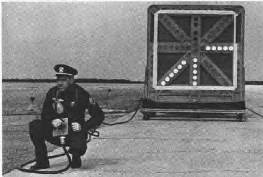
LT. CHAIRES, VX-3, HOLDS CONTROL BOX OF AUTOMATIC LSO PANEL, WHICH SHOWS 'FAST'
