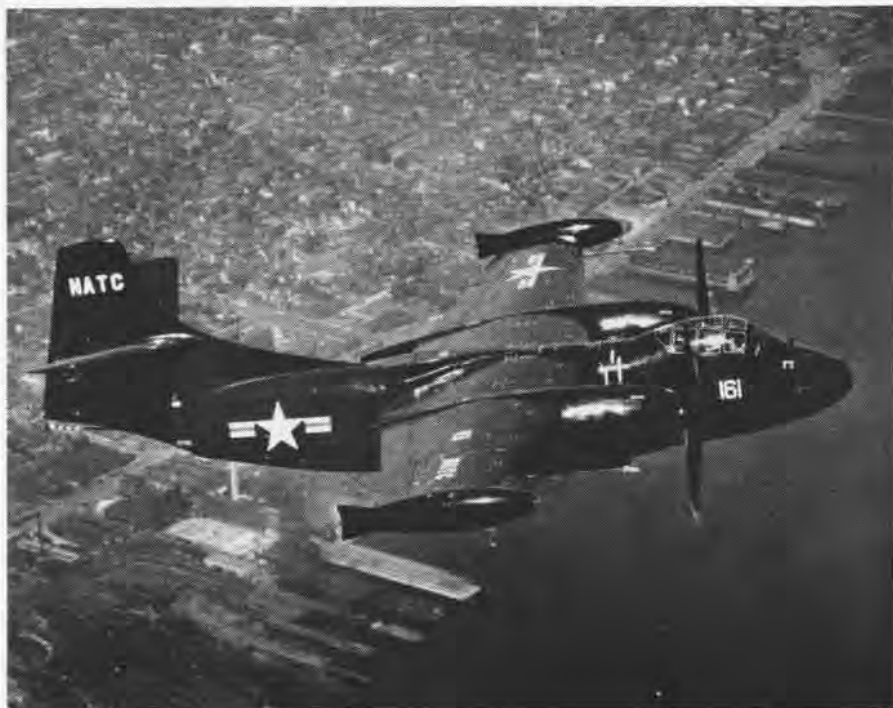
NAVY'S AJ-1 TWO-ENGINE LONG RANGE BOMBER DESIGNED TO OPERATE FROM CARRIER'S DECK
