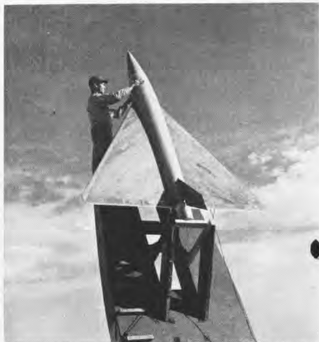
TECHNICIAN READIES DELTA-WING MODEL ON WALLOPS ISLAND LAUNCHER
