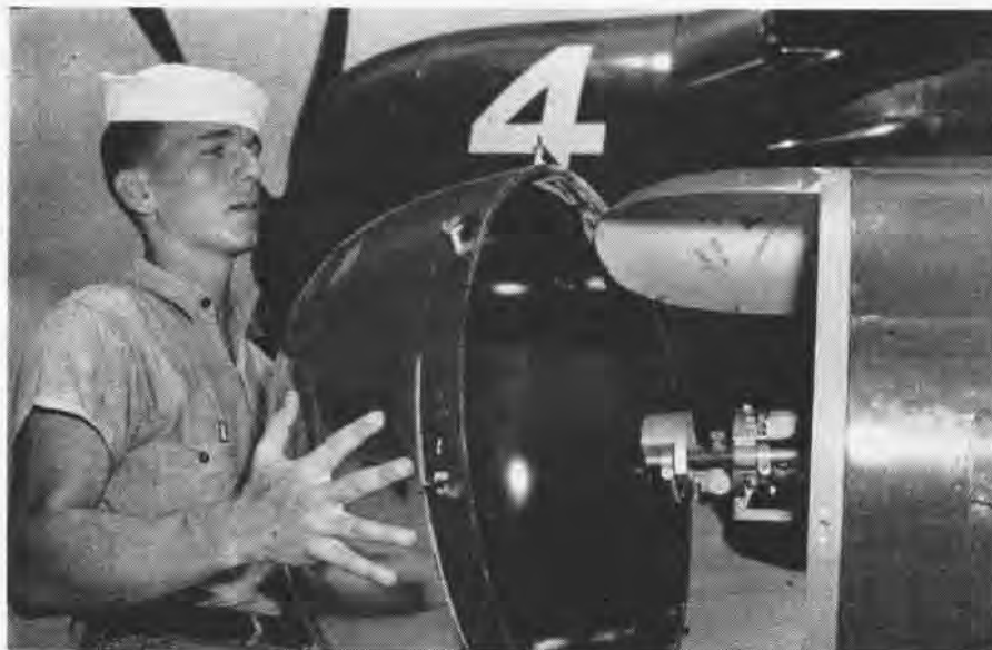
IN PREPARATION , for a night antisubmarine hop, H. S. Bridges, AD2, places plastic dome of 70 million candle power searchlight in place on wing of AD Skyraider attack plane
