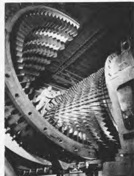
BIG COMPRESSOR POWERS SUPERSONIC TUNNEL
