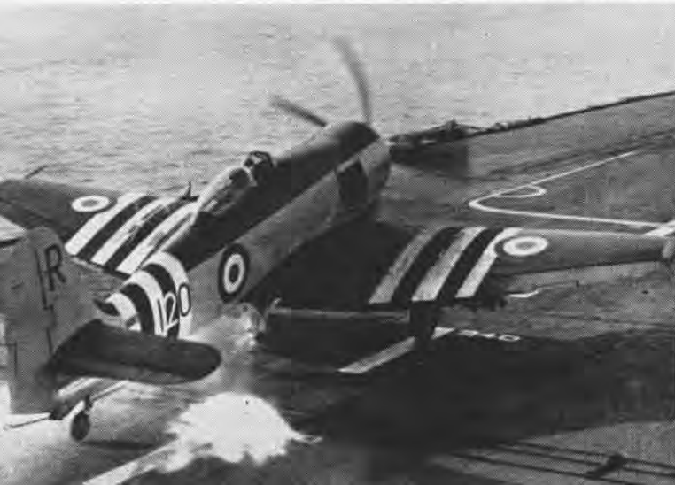
USING JATO for takeoff, a British Sea Fury plane begins running down the deck of light fleet carrier, HMS Glory in Korea waters
