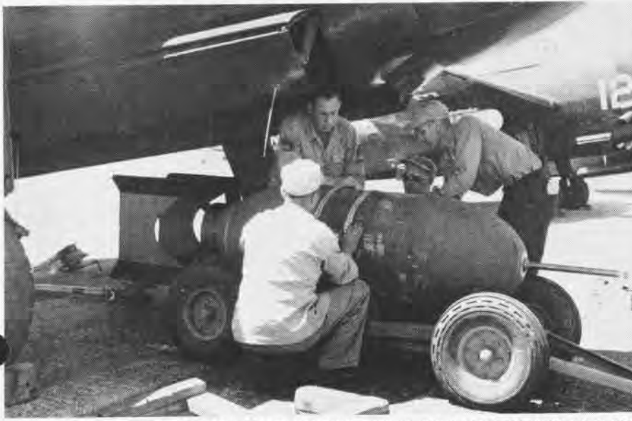
NAS MINNEAPOLIS ORDNANCE CREW STARTS HANGING 2,000 LB. BOMB FROM ITS RACK ON A TBM
