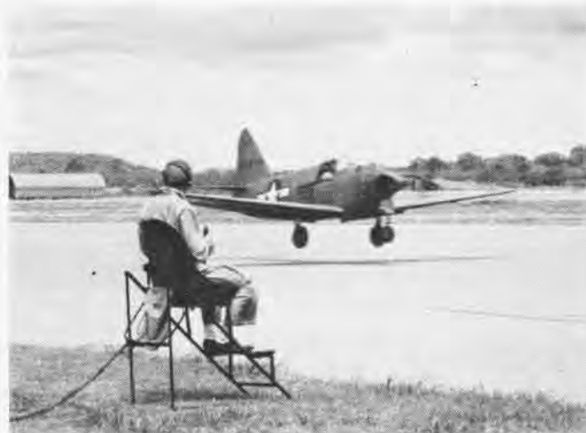
PART OF drone control work at VX-2 involves full-sized airplanes which are controlled from another aircraft, then landed as above
