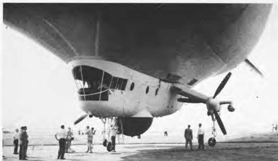
NOTE TRICYCLE LANDING GEAR, RADOME, SEARCHLIGHT ON PROP NACELLE. ENGINES INSIDE CAR
