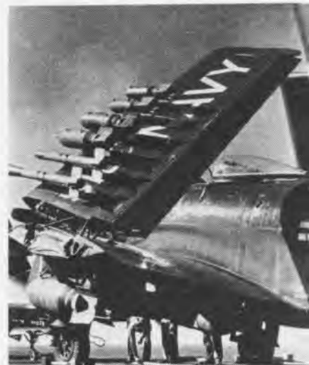
BOMB load equal to that of B-17 is toted by the carrier based Douglas AD Skyraider
