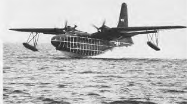
THIS STREAMLINED PBM Mariner has a new bottom. The new underbody, built by the Glenn L. Martin Co. for the Bureau of Aeronautics, is a radical flying boat hull design. The M-270 as it is called, incorporates cleaner aerodynamic lines, redesign of the nose section
