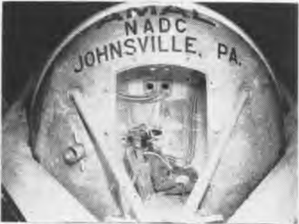
GONDOLA at end of 50 foot arm is movable to simulate dives, pushovers and pullouts
