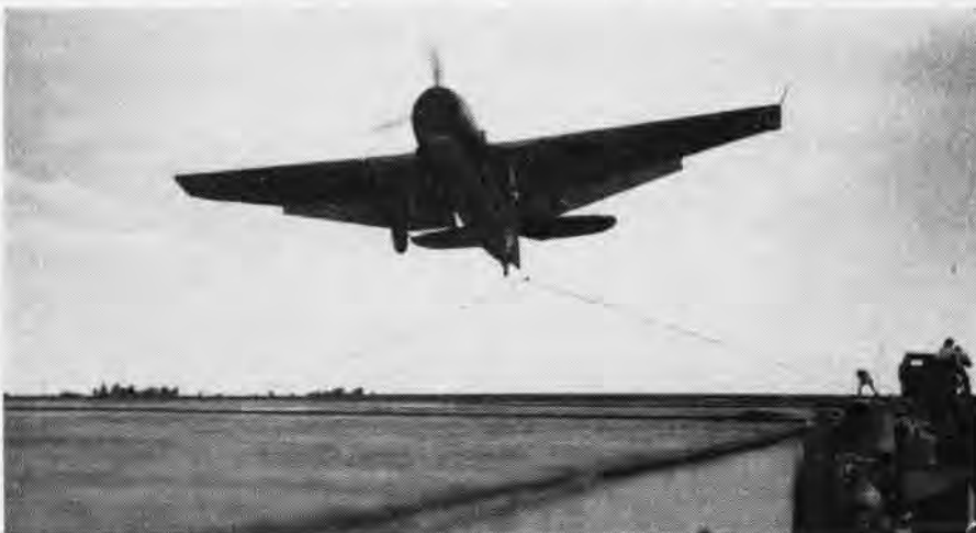
TUG OF WARS between planes and arresting wires frequently make exciting pictures, but probably none more so than this TBF aboard the Yorktown in 1944. Air Group Three with VT-3 was aboard at the time. The plane caught an early wire, bounced and the pilot applied war emergency power. Three or four seconds after the picture was snapped the wheels of this torpedo bomber extended roughly half the normal distance below the plane.
