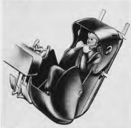
SEAT RETRACTS into capsule, control wheel retracts and doors of 'egg' begin closing
