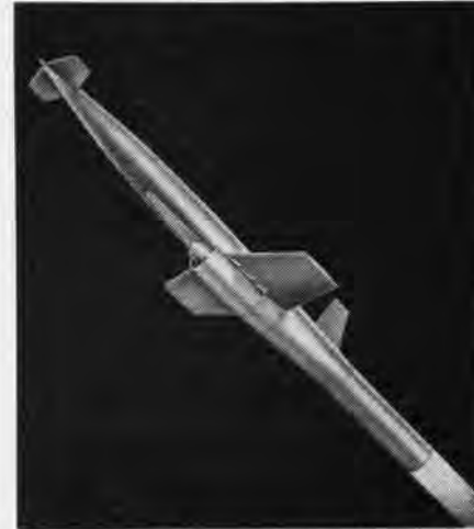
RAMJET in fuselage powers guided missile; note control surfaces on nose of the plane
