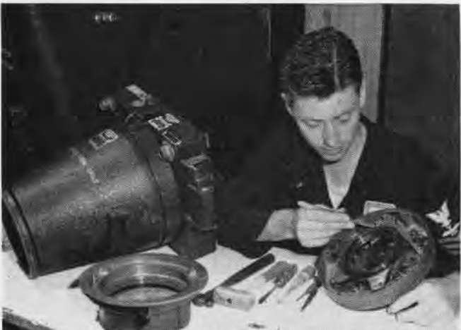
REPAIRMEN MUST BE ABLE TO REPAIR SHUTTER OF ANY AERIAL CAMERA
