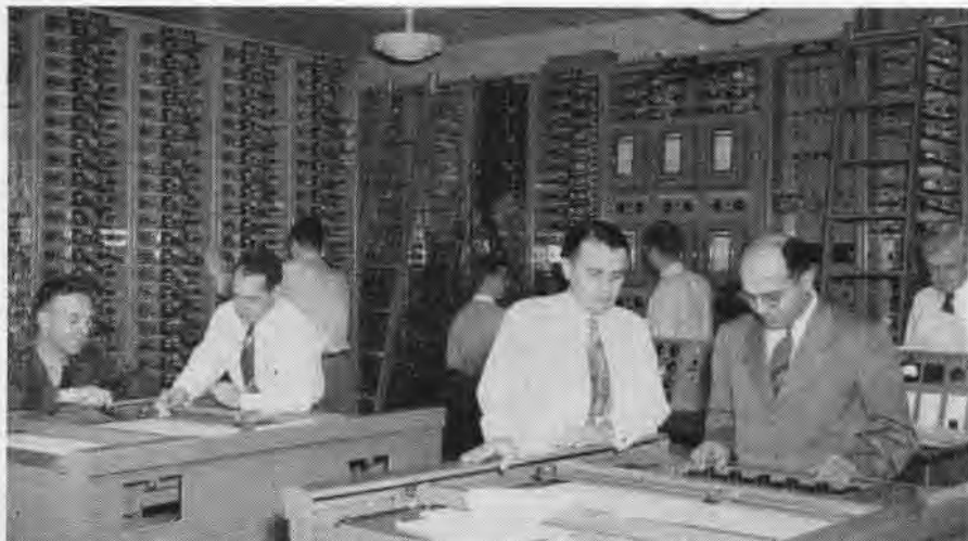
FLIGHT PATH OF A SIMULATED MISSILE PROBLEM IS STUDIED ON TYPHOON PLOTTING BOARDS
