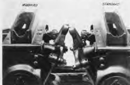
FEEDER MOUTH MODIFICATION CLEARLY SHOWN
