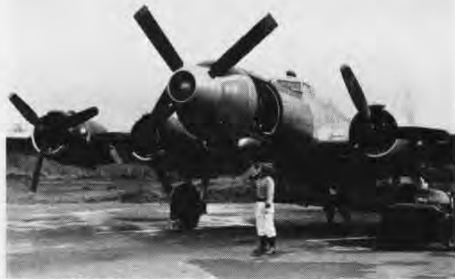
T-34 TURBOPROP HAS BEEN FLYING IN NOSE OF B-17 SINCE LAST SUMMER
