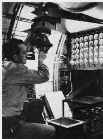
MOVIE CAMERA RECORDS ENGINE TEST READINGS
