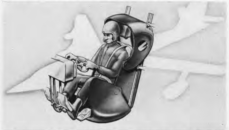
PILOT SITS FORWARD IN NEW ESCAPE CAPSULE WHILE FLYING; SHELL GIVES FLAK PROTECTION
