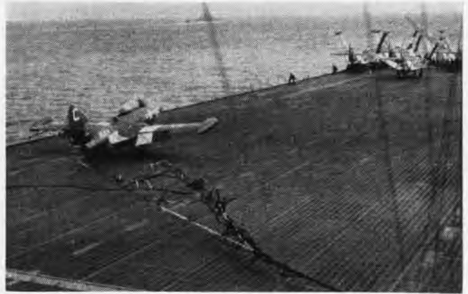
SPEED IS TOO GREAT FOR BARRIERS, SO F9F RIPS THROUGH LAST ONE
