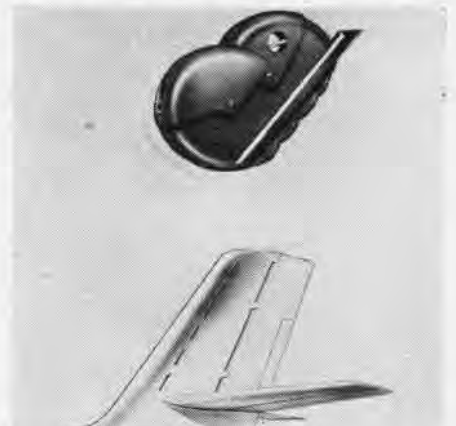
FINNS ON tail of capsule stabilize it, even at supersonic speeds, after it is ejected
