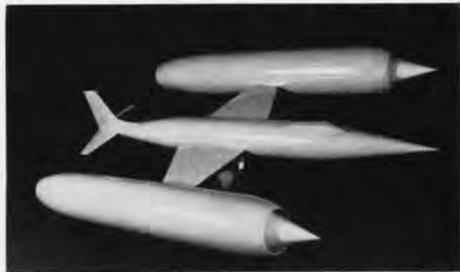
WITHOUT afterburners, the same plane would have to have huge turbojet engines like those shown here to generate same speed
