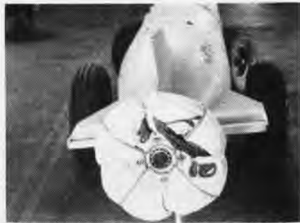
CHUTE REDUCES TORPEDO WATER ENTRY SPEED
