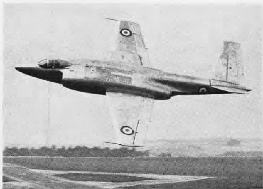
NEW VIEW OF VICKERS SUPERMARINE 508 WITH BUTTERFLY TAIL, POWERED BY TWO AVON ENGINES
