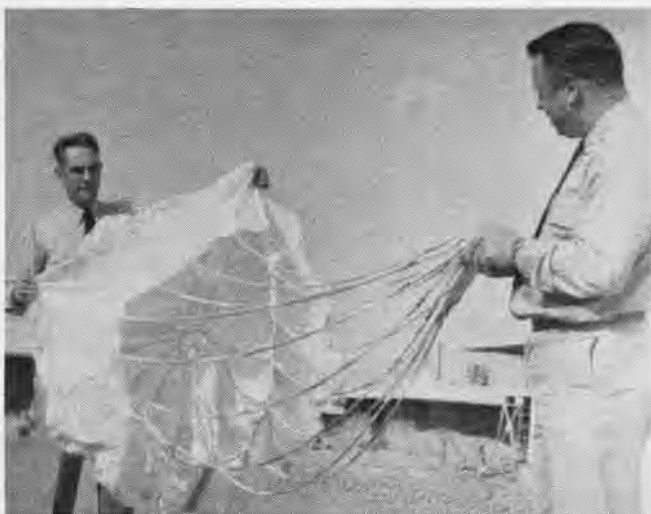
NAVY'S STURDY drogue chute for extreme speeds is held by Lt. William H. Freeman, operations officer, and LCdr. H. L. Tacker
