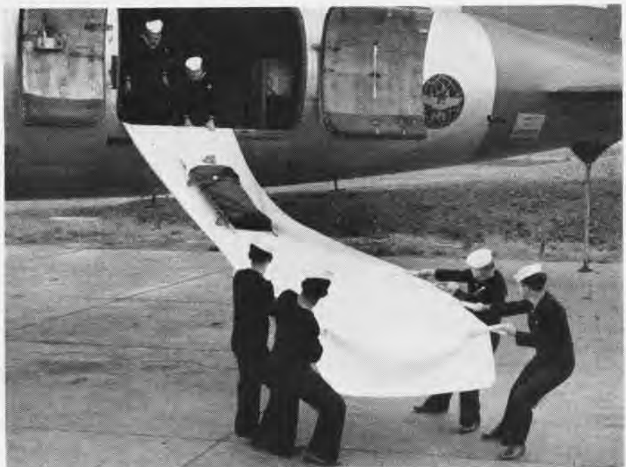
SLIDE OFFERS SAFE EXIT FOR LITTER PATIENTS IN CASE OF TRANSPORT EMERGENCY LANDING
