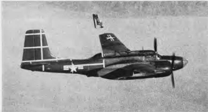
ONE OF toughest jobs at El Centro is live testing of jet fighter ejection seats; here CMach C. E. Storm is blasted out of Unit's JD-1, higher speed tests employ the TO-2 jet plane
