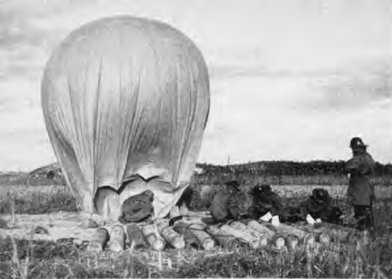
THOSE balloons which warn straying aircraft from truce talk site of Pan Mun Jom look like this; workers protected from hydrogen
