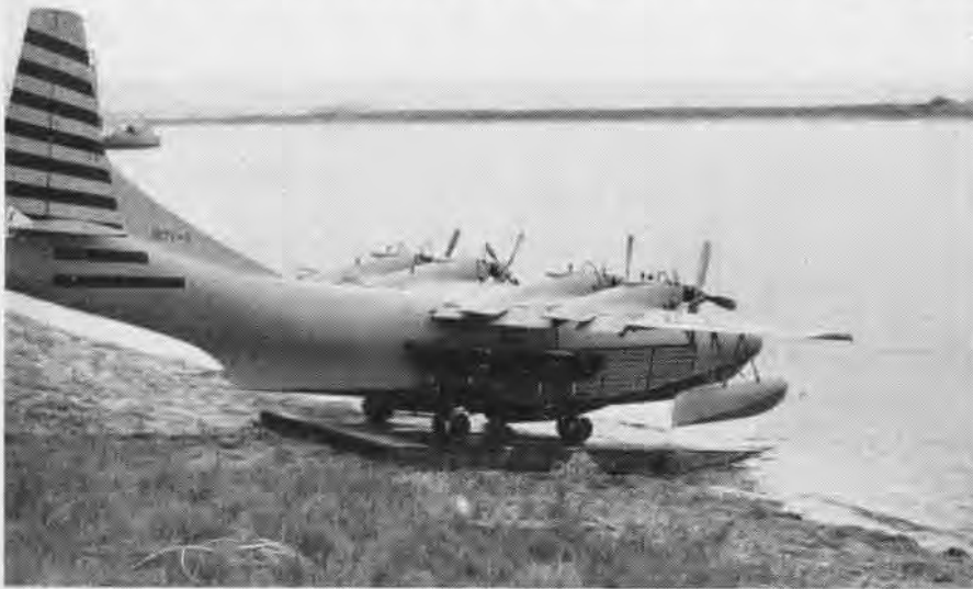
THIS one-tenth scale model of the Convair XP5Y-1 was constructed to test the big flying boat before building the full-sized one; here it tests new beaching cradle
