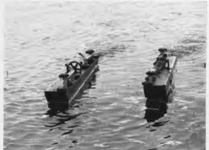
THIS large seaplane beaching cradle is self-propelled by four outboard motors and has an operator placed inside one pontoon
