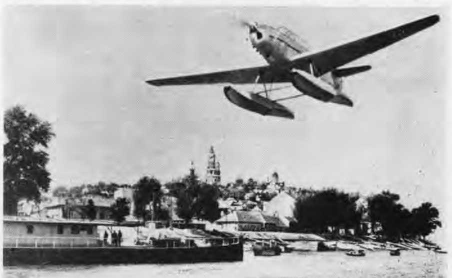
AERO-2H TRAINER IS HYDROPLANE WITH SINGLE STEP FLOATS, BRACED WITH N-TYPE STRUT PLAN
