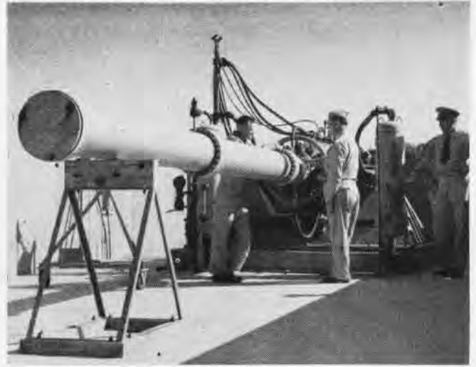
COMPRESSED air projects missile with a parachute attached from this Air Force paragon, being inspected by Navy chutists
