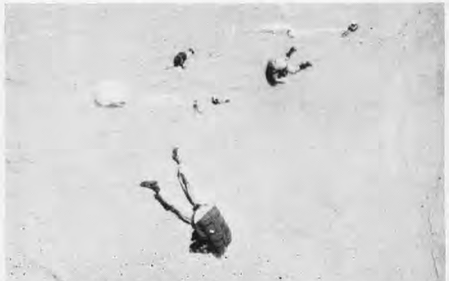
UNUSUAL PHOTO shows five El Centro parachute jumpers in air at one time over desert; some projects call for 1,000 jumps before new chute design or harness is given final approval
