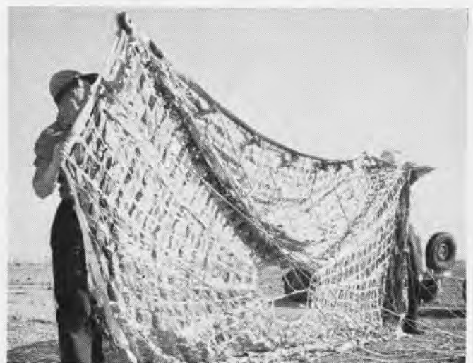
RIBBON-TYPE parachute, patterned after German-developed type, falls too fast for men but used to slow planes, drop supplies
