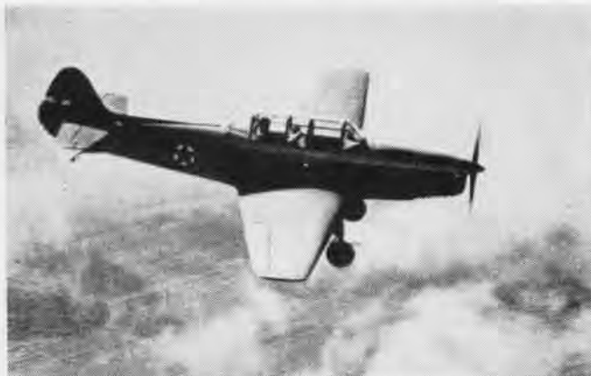
AERO-2 TRAINER IS BUILT IN YUGOSLAVIA, HAS FIXED LANDING GEAR
