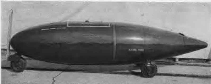
STREAMLINED STORE ENCLOSES AIR COMPRESSOR; CAN BE CARRIED ON WING RACK ON LONG FLIGHT
