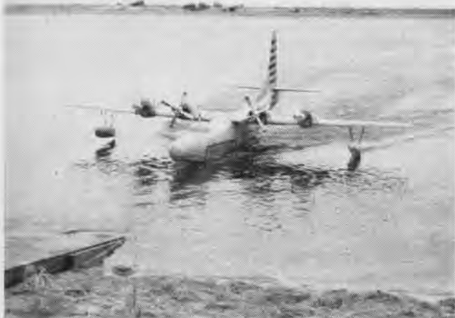
IN PRACTICE the cradle will run out to seaplane, fit on each side of hull, then plane will taxi up ramp to parking space
