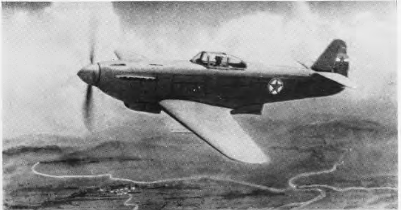
YUGOSLAV AIR FORCE DEVELOPED S-49 FIGHTER WHICH RESEMBLES RUSSIAN YAK, GERMAN ME-109; HAS 330 KNOT SPEED, CARRIES GUNS IN ITS NOSE
