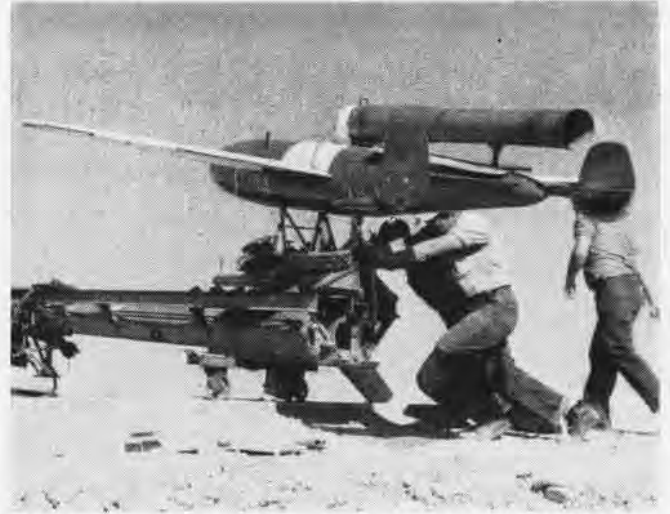
TARGET DRONES like this KD2G being tested by NATTU El Centro are saved from destruction by chutes developed by the Navy Unit
