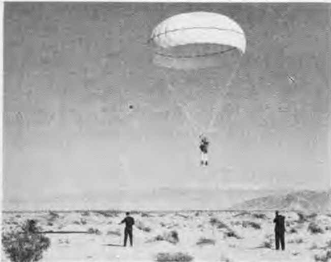
PROMISING extended-skirt type parachute lets jumper down easier than regular but 1000-jump tests have failed to solve riser twists
